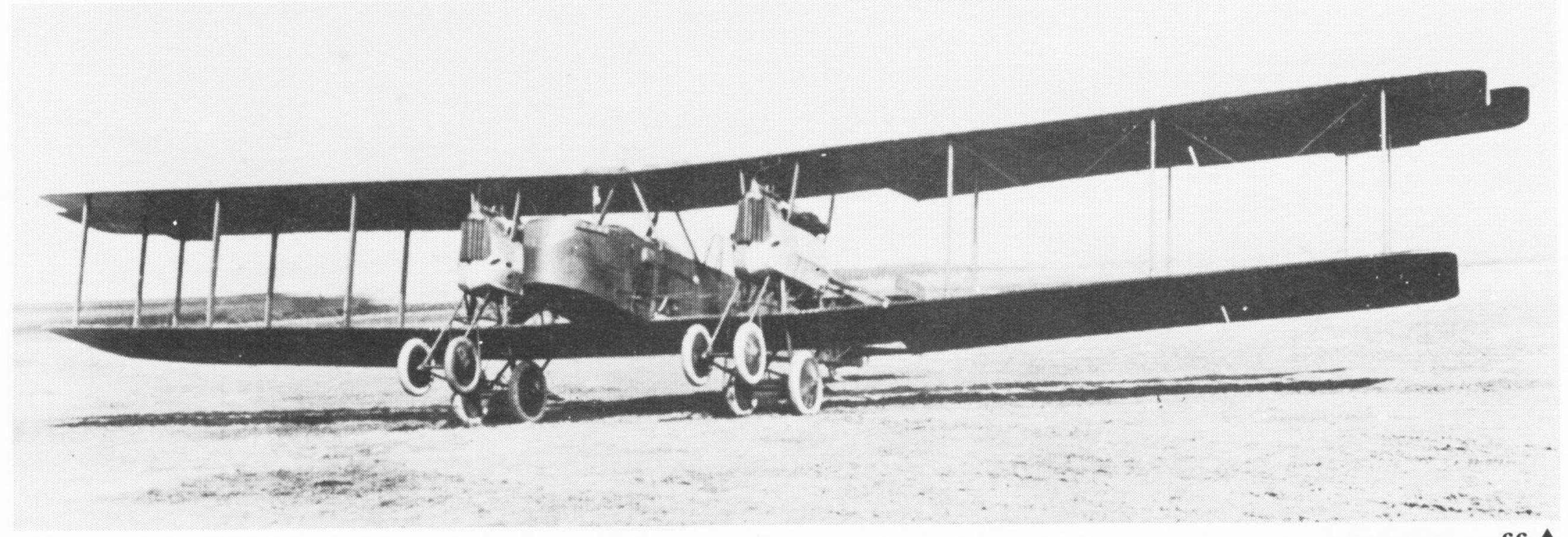
the auxiliary landing gear angled well forward to prevent the machine touching the ground with the fuselage nose, especially during night take-offs and landings. This 'stossfahrgestell' revived the feature first used on the prototype Gotha G II and patented in 1916, whereby the powerplant, including a section of the bottom wing, could be completely disconnected from the airframe and wheeled away
