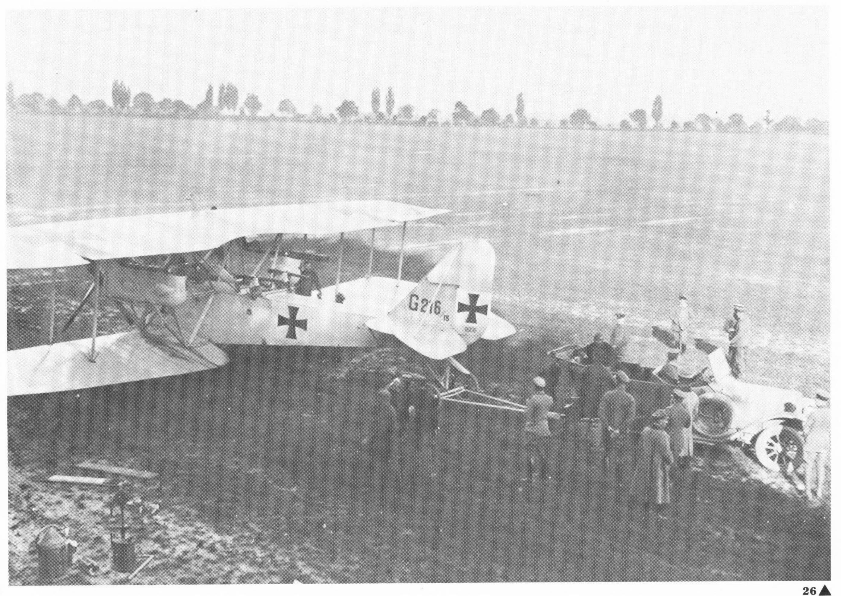
26. The touring car, a 30hp Benz 'Runabout', its bonnet marked with Kampfstaffel 7 OHL, about to pull the AEG to the take-off position by means of a wheeled towbar under the tailskid. It also provides transport for the aircrew,
