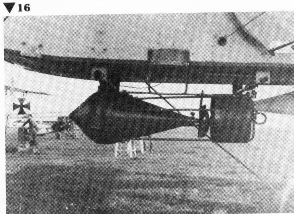
wheel landing gear approximately under the observer's front seat, but Hauptmann Hailer of Flieger Abteilung 9b had this removed from his unit's machines so that a simple rack could be installed to carry Carbonit bombs. Some pilots in other units devised means of carrying bombs under their aeroplanes by removing the claw brake usually fitted to the undercarriage spreader bar, but a number of minor accidents because of this resulted in an order forbidding 'unauthorized modifications'.
