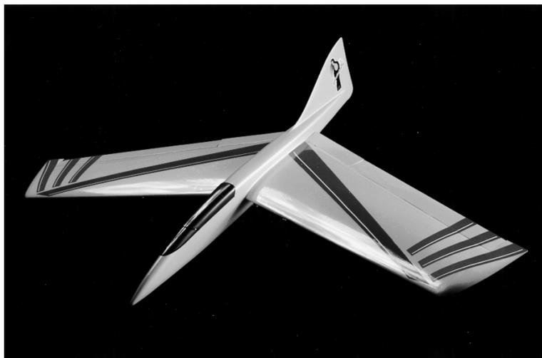
Fuselage cross section is minimal, and there's just enough room for a 225 mah battery pack, RCD Micro 535 receiver, and two Futaba 133 servos. A wing loading of 8 to 12 oz/ft<sup>2</sup> yields a good flying machine. For the experimentally minded, Larry suggests enlarging the "Toucan" to 1.5 size — thus making it a "Threecan." We're contemplating building a "Fourcan."
