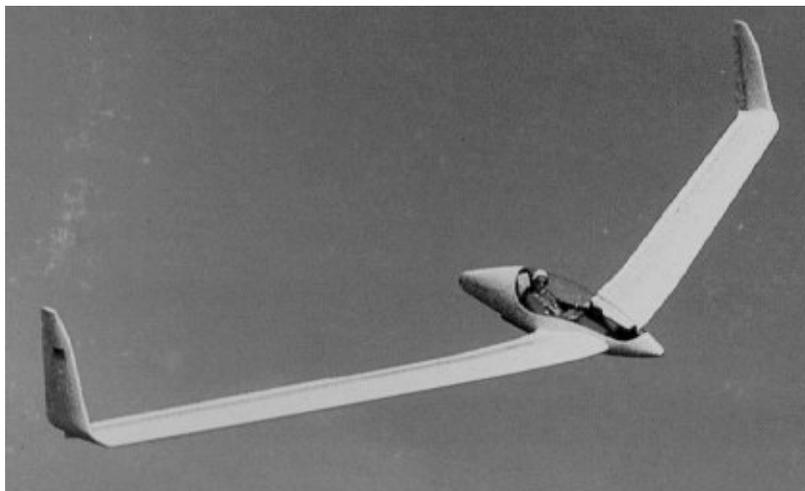
ends. The fins were then designed to cover the entire wing tip, providing sufficient area with reasonable height, and acting as winglets to reduce induced drag. A dihedral angle of four degrees was chosen to provide ground clearance for the wing tips during landing.
