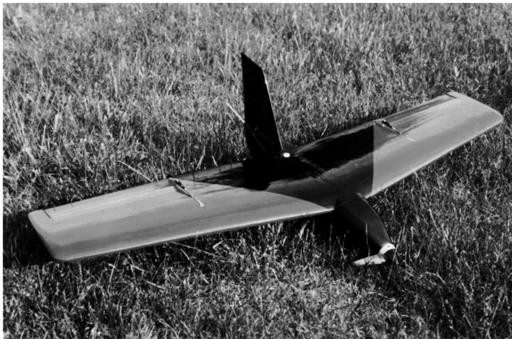
tall grass (thank goodness)! Damage was minor and quickly repaired. Rolf figured that the roll problem was adverse yaw due to the low airspeed. We moved the motor battery ahead 0.5" and tried again.
