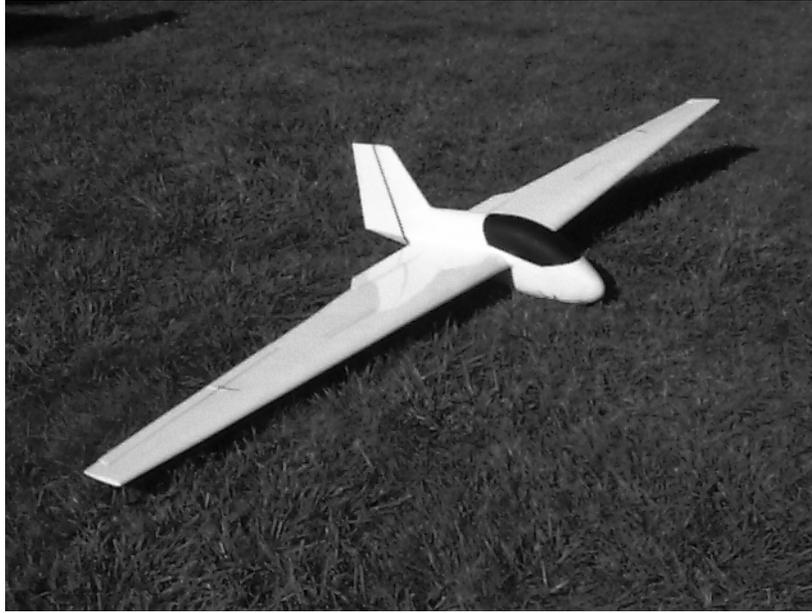
At 60 Acres in August, we got a chance to see first hand the change which had been imparted. Don had replaced the releasable tow hooks with more standard fare and constructed a bridle which snapped onto the end of the winch line. A large battery pack reduced the necessary lead in the nose to a minimum. Now all white, the Pioneer looked just like its full size counterparts.
