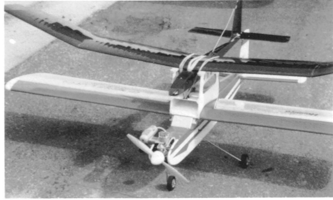
Fig. 4-21. This is a close up of the piggyback mechanism sold by Hobby Lobby with a sailplane mounted and ready for flight.
