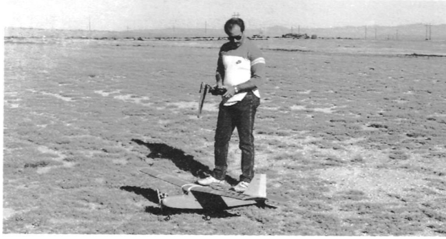
Fig. 3-11. Here's how to check the range of your radio. (Top) Collapse the transmitter and check the controls. (Middle) Walk away from the model while checking the controls. When control is lost, note the distance. (Bottom) Finally, extend the antenna. If control is regained, the check is complete.
