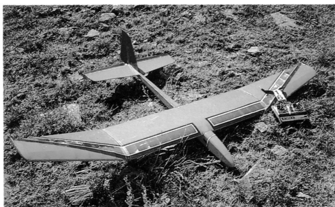
Fig. 2-3. Olympic 650. This two-meter sailplane is great for slope soaring as well as thermal flying
