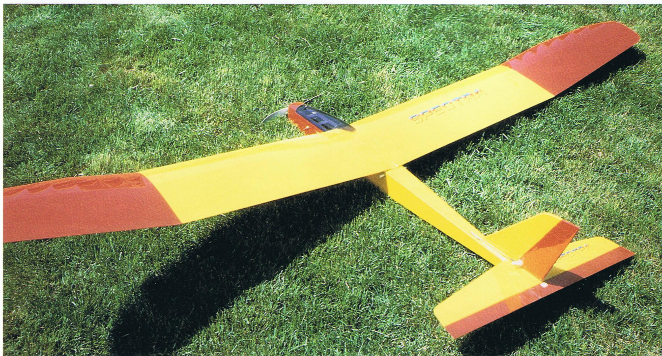
Fig. 1-2. The Spectra, produced by Great Planes, is an electric-powered sailplane. Because of its electric motor and propeller, it has all four forces of flight exerted on it.
