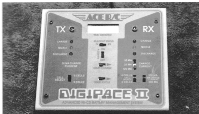
Fig. 3-14. The Ace Digipace II. This is the best unit to use when you need to charge or recondition your radio batteries.
