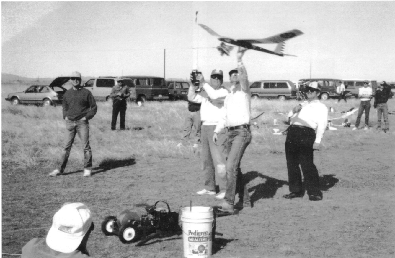
Fig. 4-1. An instructor launches his student's sailplane on a winch. The student can now concentrate on keeping the sailplane straight during its climb.
