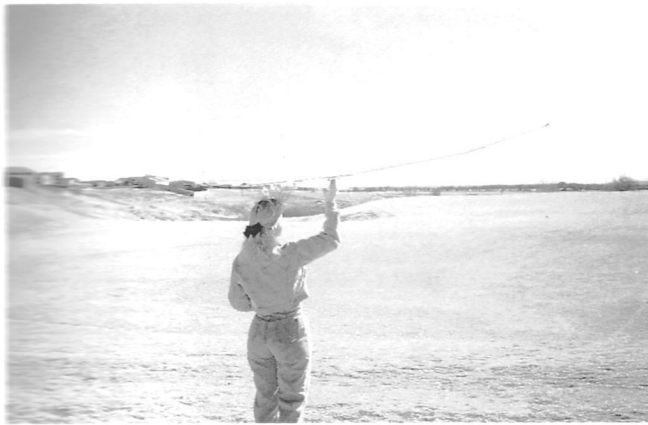
Fig. 4-2. To check the model's trim gently launch the sailplane straight ahead into the wind and keep it flying on a straight line with a gradual descent. After landing, change the trim tabs and control clevises until the plane flies straight with a good glide each time.
