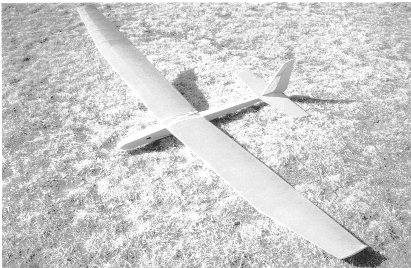
Fig. 2-8. Olympic II. This great flying sailplane has a 100-inch wing and is easy to build. It is light and has a terrific glide.
