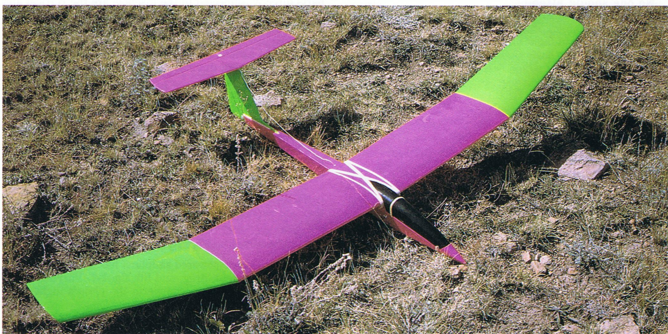
Fig. 1-3. This beautifully finished Sophisticated Lady by Goldberg Models features a T-tail. This allows the horizontal stabilizer and elevator to be up and out of the way of potential ground obstacles.
