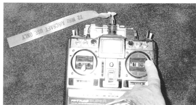
Fig. 3-9. When the right stick is moved to the right the rudder on a two-channel plane moves to the right and vice-versa.
