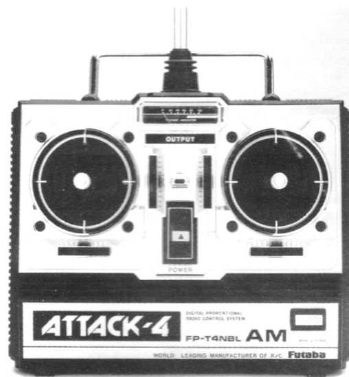
Fig. 3-2. Futaba 4NBL Transmitter. This is the same transmitter used in Futaba's popular four-channel system as well as in its set for electric-powered airplanes.
