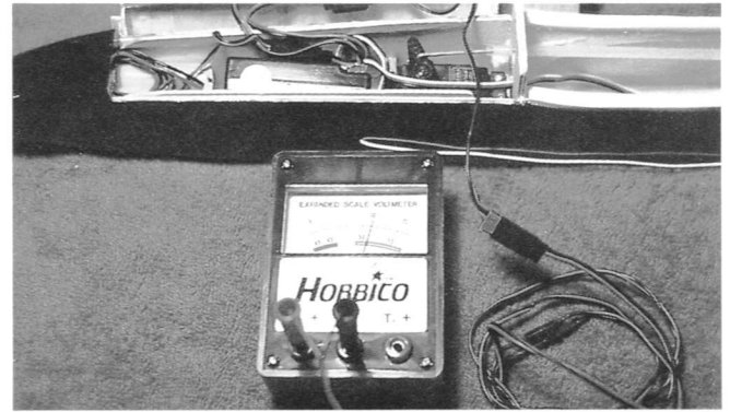
Fig. 3-13. This ESV (Expanded Scale Voltmeter) is being used to check the receiver battery's voltage before another flight. This inexpensive device can save you many dollars worth of damage.
