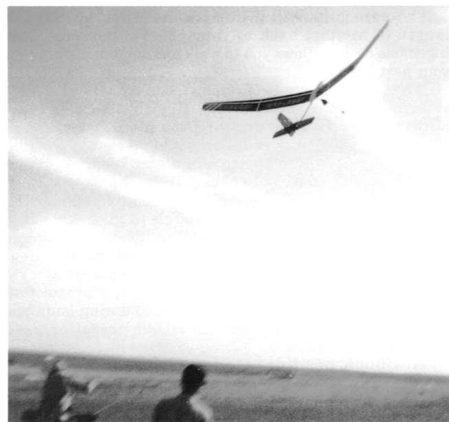
Fig. 4-12. (Second from top) This is a typical 12-volt winch that you can make easily. The car battery is connected to a starter motor that drives the large metal spool in the front. The foot activated switch is seen in the foreground. (Bottom two) Here is an actual launch using an electric winch. As soon as tension is felt in the launch line, the sailplane is firmly thrown forward and upward. Be sure to keep the wings level throughout the climb.
