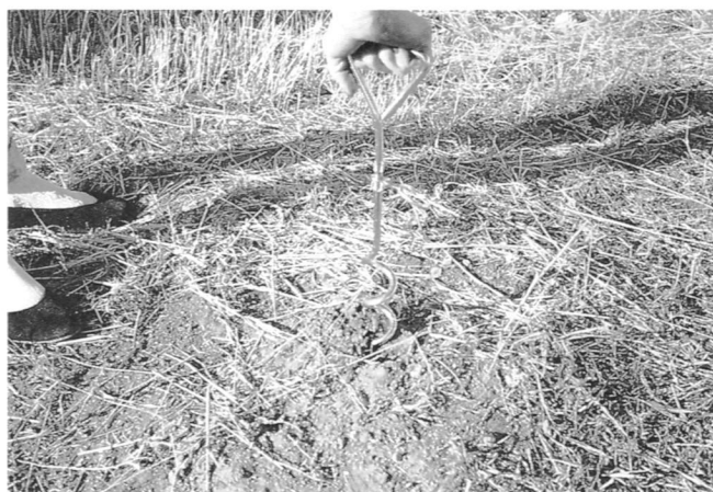
Fig. 4-7. This spiral dog stake can be bought at most pet and variety stores. I recommend that you use one with your hi start for added safety.
