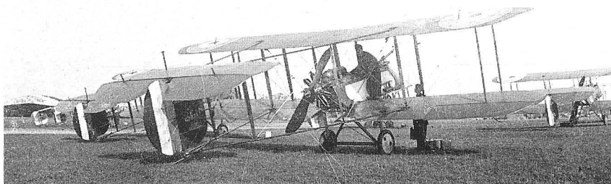
Vickers FB9s. The 'pusher' arrangement of the engine and propellor is particularly clear.
