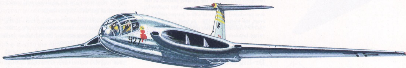
Heinkel's four-jet long-range bomber of 1945 was designed to carry a 3,000 kg (6,612 lb) bomb load over a range of 28,000 km (17,388 miles).
