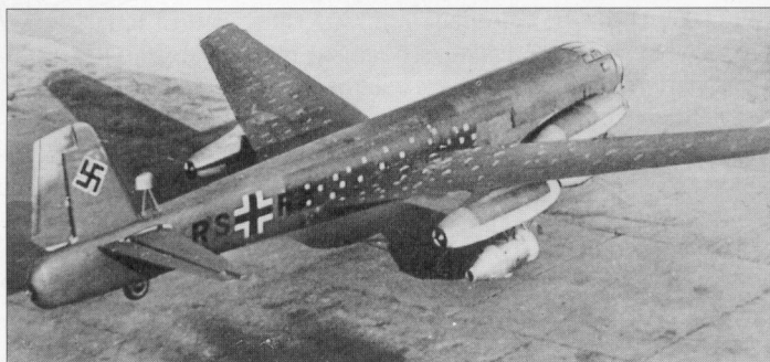
Bottom right: The Junkers Ju 287 V1 being readied for flight at Dessau. The undercarriage units came from a captured US B-24 Liberator bomber. Note the dynamo trolley used to start the turbojets.
