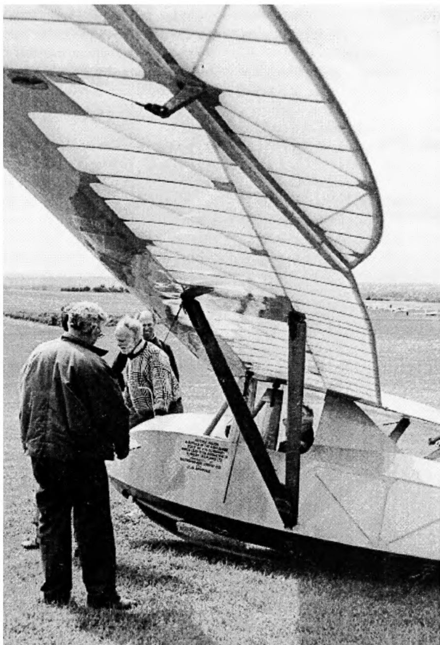
A poem in varnished ply and clear doped fabric – Mike Beach's replica of the Falcon I of 1928.
