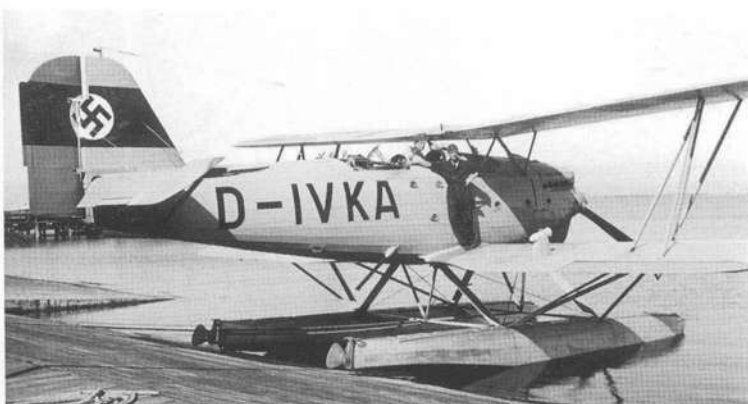
Ground crew pose with Heinkel He 60 C, D-IVKA at Berg am Rügen circa 1936. Finished in overall 63 with unpainted but treated floats, its black-painted civil registration and Reichsflagge across the fin and rudder suggests that the aircraft was in use up to the time of the unveiling of the new Luftwaffe.
