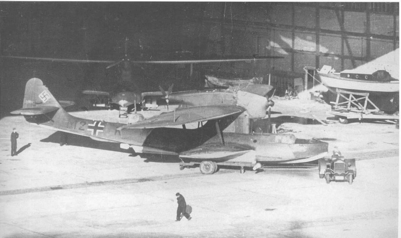
Finished in the standard 72/73 maritime camouflage, this Dornier Do 18 G-1 of the 2./KFIGr.106 carries the unit code and Staffel letter but has yet to have the individual aircraft letter applied. Although similar in general appearance to the Do 18 D, the G-1 featured a recontoured bow, a pair of more powerful Junkers Jumo 205D engines and improved defensive armament consisting of a 13 mm MG 131 in the bow position and a 20 mm MG 151 cannon mounted in a hydraulically operated turret in the rear fuselage. It also carried provision for the attachment of take-off assistance rockets.
