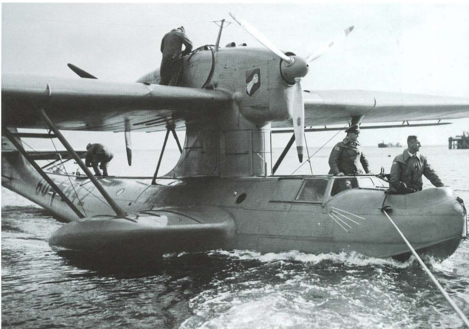
The Dornier Do 18 flying boat played a significant role in early wartime reconnaissance duties with its long-range capabilities making it a valuable asset in the Wehrmacht inventory. In this pre-war view, the aircraft appears to be under tow while servicing personnel attend to the dorsal gun position and the aft-mounted Jumo diesel engine.
