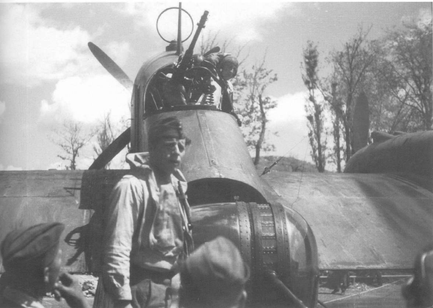
A stern view of a Blohm und Voss Bv 138 C-1 of the 3./SAGr. 125 showing the twin defensive weapons stations, the lower rear turret mounting a single MG 151 20 mm cannon and the upper open station, a 13 mm MG 131 heavy machine gun.
