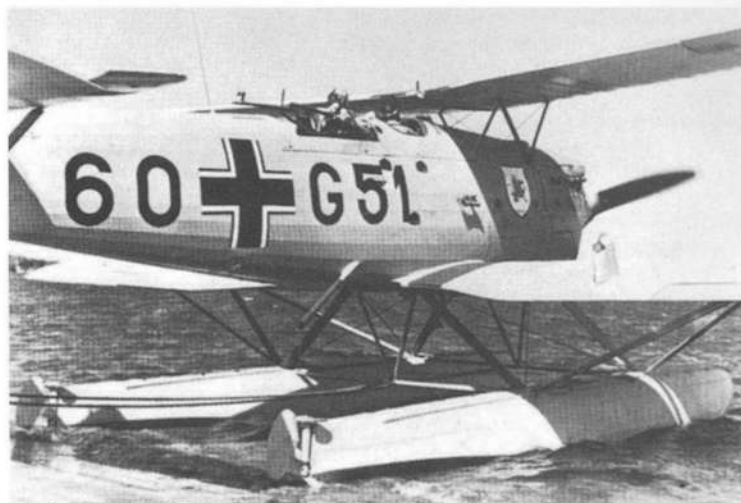
In this view the pilot of Heinkel He 60 C, 60+G51 of the 1./KFIGr.506 is starting his engine in preparation for moving away from a slipway, probably at its base at Dievenow – note the mooring lines still attached to the central float strut assembly. Visible on the forward fuselage is the Staffel emblem of a brown or red Griffin on a blue-bordered white shield.
