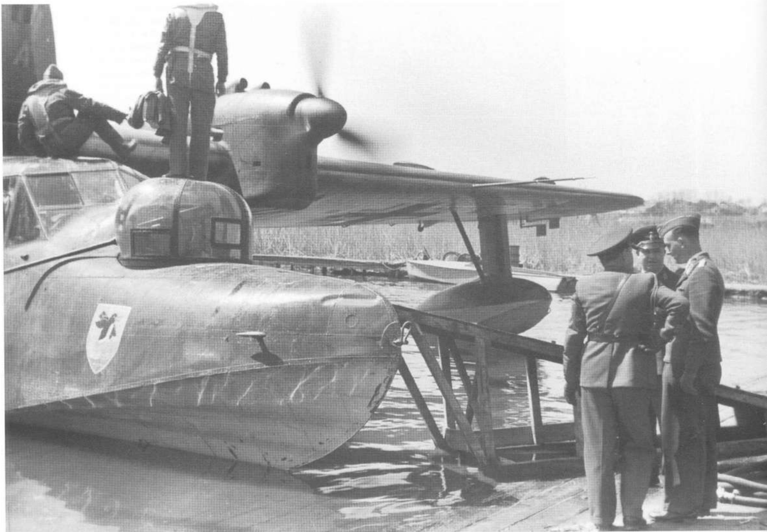
This frontal view of a Blohm und Voss Bv 138 C-1 of the 3./SAGr. 125 at Mamaia on the Black Sea coast gives a clear view of the bow-mounted turret, which, like its twin at the stern, mounts a 20 mm MG 151 cannon. The Bv 138s of the 3./125 would later play an important role in the evacuation of Kerch.
