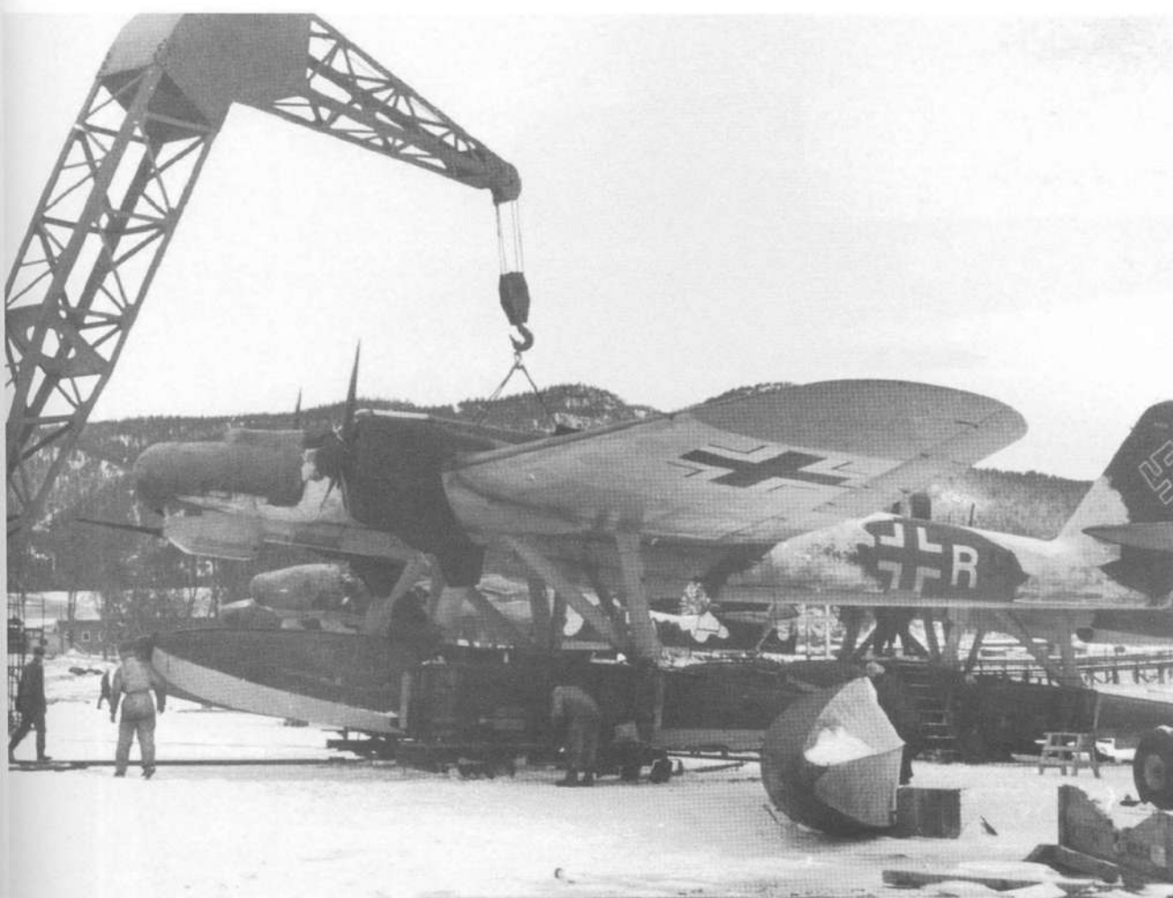
Wearing a partial temporary white finish over its standard 72 & 73 camouflaged upper surfaces, K6+RH, a Heinkel He 115 C-1 of the 1./KFlGr.406 is seen undergoing a float replacement at Trondheim during the winter of 1942.
