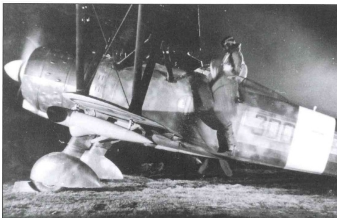
Equipped with searchlights (seen fitted under the fighter's port wing), this CR.42 was assigned to 167° Gruppo Autonomo 's 300 a Squadriglia , which was created in May 1942 to oversee the nocturnal defences of both Rome and Naples (via Giorgio Apostolo)
