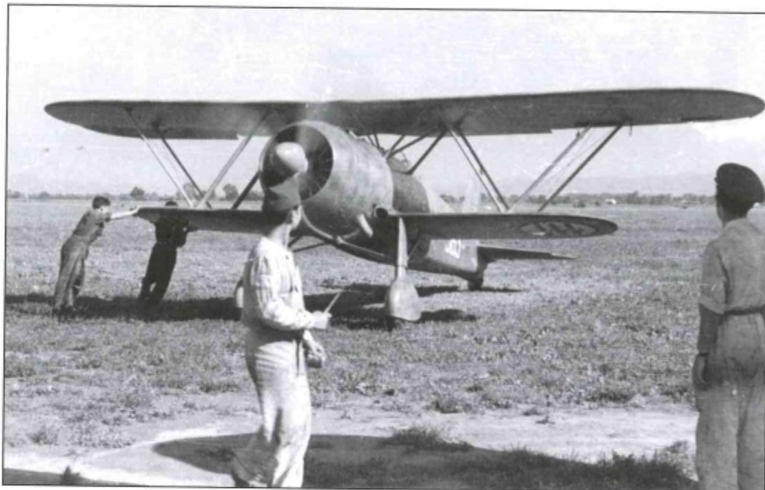
A CR.42 of 150° Gruppo taxis in after landing at an airfield near Valona. It is about to be swung round with the help of a burst of power and the mechanics holding onto the starboard wing (Giorgio Apostolo)
