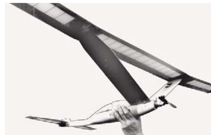
CF587 AVIAFIBER. Sport-Scale R/C hang glider can be flown as a sailplane or with .049 eng. Uses 2 to 3 channel gear. Big 75-inch span. H. Applegate. FM 1-82. $$C
