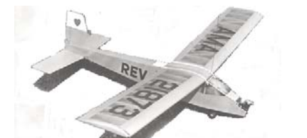
CF415 REVISION A. Single or 2 channel R/C trainer, featuring 44-inch span. For .09 eng. H. Applegate. FM 8-76. $$C
