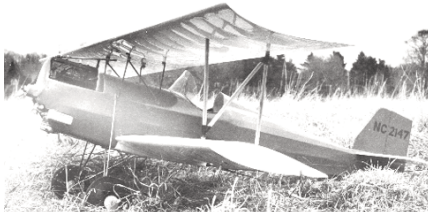
CF407 BIG "GERE" SPORT. R/C Stand-Off Scale biplane for .60 power. Has 54-inch span, and uses 4 channel guidance. Dr. J. Makovich. FM 6-76. $$D
