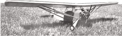
CF867 TAYLOR CHUMMY. Parasol wing Sport-Scale design for R/C. Spans 51 inches and requires .15 to .25 two cycle eng. A. Wolsky. FM 11-91. $$D
