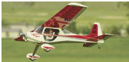
CD436 SKYSPORT . A model that someday maybe a full scale aircraft! Designed as a proof of concept, the SkySport features a unique counter-rotating prop design that keeps the craft arrow straight. The high wing design is stable for fun sport flying and the cockpit features an interior. Weighs 32 ounces, ready to fly, spans 47 inches. Plan on two sheets. Clark Salisbury FM 04-2012 $$$E
