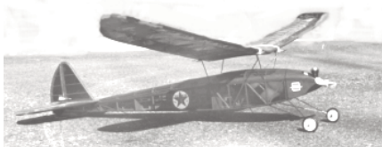
CF700 TEXACO MG. Mike Granieri's classic old timer down-sized for Texaco endurance events. 51-inch span, .049 eng., 2 channel R/C gear. M. Granieri. FM 6-85. $$C
