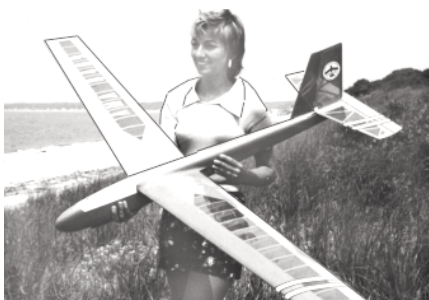
CF317 LONG ISLANDER. R/C slope or thermal soarer features 100" span. B. Aberle. FM 12-73. $$$D
