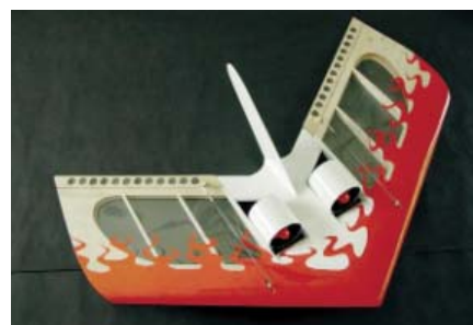
CD217 JET JUNIOR An R/C twin electric ducted fan sport model suitable for park flying. All balsa construction with a wing span of 26¼ inches. Weight is 11 ounces. For three channels, it uses EDF-50 fans. Plans on one sheet. Olan Hanley. FM 03-2004 SSC
