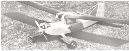
CF710 GOOD BUDDY. Sporty parasol wing R/C trainer for .15 eng, and 3 channel radios. Spans 66 inches. J. Cole. FM 10-85. $$D
