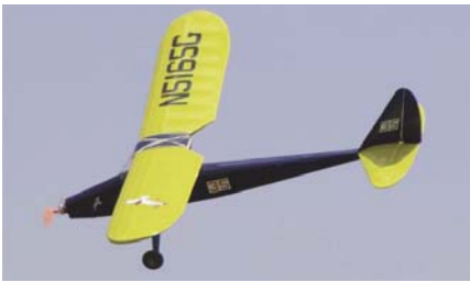
CD429 GULL II . Based on the Comet freeflight model, Pat Tritle enlarged the original drawings to make this a relaxing R/C model. The Gull II is just the thing for those early morning or late afternoon flights. Model is built of traditional balsa and ply construction, and uses a Tower Pro 2208/17 brushless motor, 20-amp ESC and two 9-gram sub-micro servos. Weighs 13 ounces, ready to fly, spans 50 inches. Plans on two sheets. Pat Tritle FM 12-2011 $$$L
