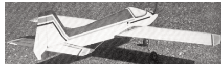
CF637 THE HAMMER. High-performance R/C Sport-Pattern design, featuring 50-inch span. For .19 to .25 eng., and 4 channel gear. D. Sarpolus. FM 7-83. $$D
