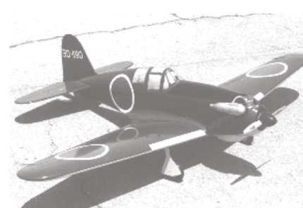
CF784 MITSUBISHI J2M3 RAIDEN. R/C Sport-Scale model of WWII fighter. Has 68-inch span, requires .60 to .61 eng., and 4-channel system. D. Reiss. FM 9-88. $$F
