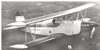
CF921 GRANDSON. Sporty R/C Biplane uses a geared Astro 40 motor and 21 cells. Spans 61.5 inches, 1180 sq. in. Two sheets. Ellis Grumer. FM 12-93. $$L
