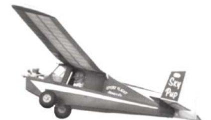
CF919 SKY PUP. Here's a true quarter scale model of an ultralight for 3-channel operation and a .45 2-cycle eng. 93-inch span. Al Wolsky. Two sheets. FM 11-93. $$Q
