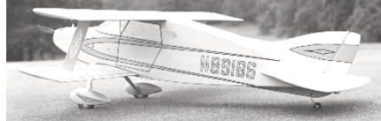
CF349 HIPERBIPE. Wild looking R/C Stand-Off Scale biplane, 45-inch span, 4 channel R/C, .40 eng. S. Hines. FM 11-74. $$D
