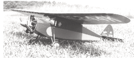
CF678 KARI KEEN COUPE. 1930's lightplane for fine R/C flying. has 60-inch span, 3 to 4 channel system, .35 eng. A. Wolsky. FM 10-84. $$D
