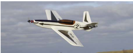
CD 420 ARROW . A fun, go fast, go where you point it, twinmotor hot rod! The Arrow builds fast with traditional balsa construction and is powered by two brushless outrunner motors. This unique electric twin is sure to get noticed at the field. 3 channels, 2 sub-micro servos. 35.5-inch wing span, flying weight of 19 ounces. Plans on two sheets. John Rutter. FM 07-2011 $$$M
