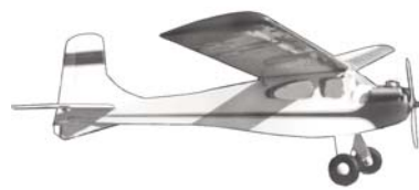
CF624 R/C SUE. R/C version of perennial freeflight favorite. For 3 channel radio, and .19 to .25 eng. Has 59-inch span. D.B. Mathews. FM 3-83. $$D
