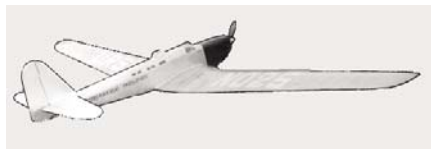
CF546 ANT-25. 96" span R/C powered glider for .09 eng. Semi-scale design of Russian endurance ship. P. Bosak. FM 9-80. $$$D
