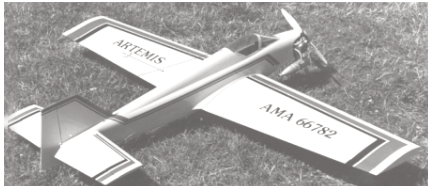
CF714 ARTEMIS. Aerobatic Sport-Pattern ship, featuring 58-inch span. .40 to .45 eng., 4 channel radio. R. Allison. FM 12-85. $$D
