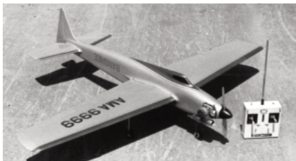
CF236 BANSHEE. R/C design for full AMA/FAI patterns. The 62 inch span bird needs a hot .61 eng., and 5 channel R/C gear. J. Martin. FM 9-71. $$D
