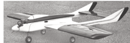
CF550 VAMP. R/C Sport-Pattern, twin-boom ship with 58-inch span, .40 eng., and 4 channel gear. J. Sheeks. FM 10-80. $$$
