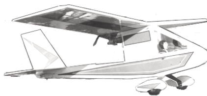
CF525 QUIXOTIC. R/C sport pusher design, with a 67-inch span, .35 eng., 4 channel gear. D.B. Mathews. FM 12-79. $$$
