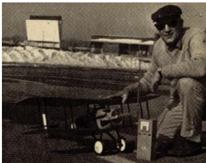
CF057 SPAD SV-II. French WWI fighter requires 3 to 4 channel R/C systems and .09 eng. 43-inch span. P. Palanek 5-64. $$J
