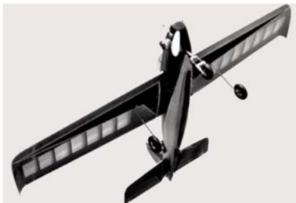
CF232 VICTOR. Originally designed for Open Pylon racing 4 channel R/C design is fine for hot sport flying: 56-inch span, and uses .45 eng. G. Rogers. FM 8-71. $$D
