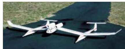
CD210 WHITE KNIGHT Join the next 100 years of flight with this electric ducted fan scale model of Burt Rutan's futuristic launch aircraft for space flight. An R/C giant, its wing spans 134 inches and has an area of 1044 square inches. Power required are two Midi Fans with Mega 22/30/3 motors on two 30-cell packs. Construction is balsa over foam for the wings, balsa and ply for the booms, and fiberglass for the pod and nacelles. Finished weight 16 pounds. Plans on four sheets. Ivan Munninghoff. FM 12-2003 SSU
