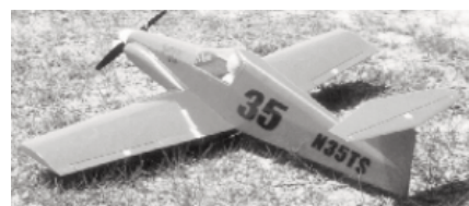
CD065 SUMP 'N ELSE. This little 34 1/2-inch R/C ship is one of three patterned after Formula One racers. It's great as a racer with a .15 2-stroke, but can be flown as a sport ship with a .10. Uses three channels; rudder optional. Build this one or all three. Jim Wise. FM 11-98. $$$
