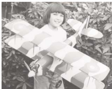
CF420 SUPER SPAD. Scale-looking R/C sport biplane with 38-inch span, .19 to .30 engs. 4 channel gear. G. Weaver. FM 10-76. $$D
