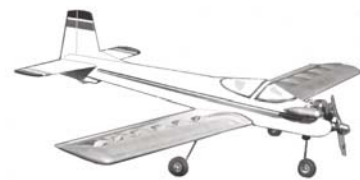
CF642 PEPPER. Low wing R/C sport design with 50-inch span. .19 to .25 eng., 4 channel R/C. D. Sarpolus. FM 9-83. $$D
