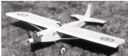
CD005 PILCHARD, A FAUX FIGHTER. This .20 size R/C ship could have been the scourge of the Eindecker, but is more at home for Sunday flying. 47 \frac{3}{4} -inch span, foam board construction. Plans on two sheets. Roy Clough Jr. FM 10-96. $$G
