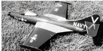
CD108 F9F PANTHER. This jet uses a cobalt 05 motor driving an APC 7-7 prop. Spans 39¼ inches, and needs a 3-channel radio. Can also use a brushless motor. Pat Trittle. FM 04-2000. $$D
