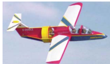
CD141 RFB600 FANTRAINER An R/C Sport Scale ducted fan, without the ducting. All balsawood construction, except for the wing which has a foam core. With a wing span of 77 inches, its finished weight is about 11½ pounds with optional retracts. Requires a .61 to .75 engine, and 4-6 channel radio gear. Canopy and servo fairing available from the author. Greg Moore. FM 07-2001 SSQ
