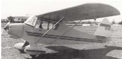
CF462 PORTERFIELD COLLEGIATE CP-65. Stand-Off Scale R/C ship with 74-inch span. For .35 to .45 eng., and 4 channel gear. D. B. Mathews. FM 2-78. $$D
