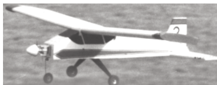
CF591 CAPRA. Foam board is the principle construction material used in this R/C utility trainer. 68-inch span, .40 eng., and 4 channel gear. D.B. Mathews. FM 2-82. $$D
