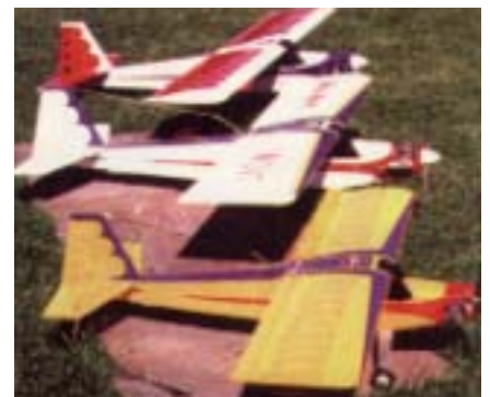
CD040 AKRO-KNAT. Under the guise of a high wing sport ship lies a real R/C aerobat for a .25-.36 size 2-stroke. Yet still, it's very stable at very slow speeds. Spans 50". Michael Chattin. FM 11-97. $$J
