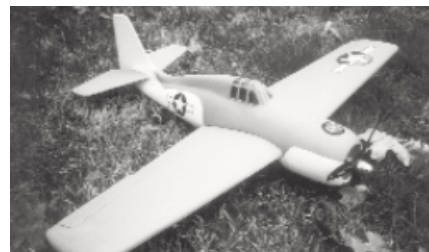
CD060 WILDCAT. Whether you use it for AMA 704 Combat or just plain sport flying, this 38-inch span R/C sport scale ship uses a .15-.21 glow engine. Needs a 3- or 4-channel radio. Gus Morris. FM 8-98. $$$
