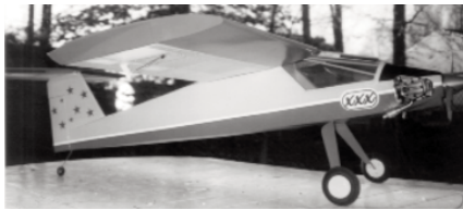
CD004 TRES EQUIS. Snappy T-tail R/C sport model is all balsa construction; 46 \frac{3}{4} -inch span, .40 four-stroke, or .32-.40 two-cycle. Plan is two sheets. Bill Brechley. FM 9-96. $$H
