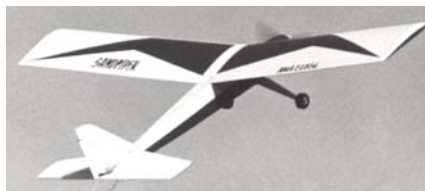
CF902 SANDPIPER. 60-inch span electric R/C sportster; Hobby Lobby Turbo 700 motor, 4 Channel R/C gear. Plans on 2 sheets. B. Winter. FM 3-93. $$$J
