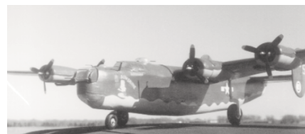
CD035 B-24 LIBERATOR. Two PAW 03 diesels power this 2-3 channel R/C model of WW II bomber as the "G," "H," or "J" model. Can also substitute two Cox .049s. Spans 62 inches, weighs 34 ounces. Eric Clutton. FM 9-97. $$$
