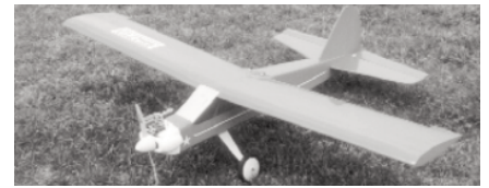
CD029 MAINSTREAM. Fun flying by one of R/C's most respected seniors. 72 \frac{3}{4} -inch span flown originally on an ST .46, livelier with a .50-.60 two-stroke. Bill Winter. RM 7/97. $$M
