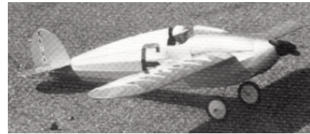
CF696 HEATH BABY BULLET. Schoolyard racer for 1/2A power, 35-inch span, 2 channel R/C gear. M. Leasure. FM 5-85. $$C
