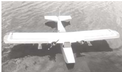
CF942 RIPPLE SKIPPER. Two versions of R/C electric twin seaplane, with or without ailerons. One spans 49½ inches. Two spans 52¾ inches, uses two Astro Flight 035 motors. Plans on 2 sheets. P. Hook. FM 9-94. $$ K.
