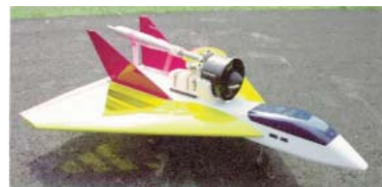
CD175 SUNSPOT A kit bash of the popular delta pusher, the Force One , designed by Laddie Mikulasko and kitted by Balsa USA. This revision utilizes fan power from a K&B 7.5DF and Turbax I fan system. A stretched nose and larger fins streamline the model. Wing spans 36½ inches. Finished weight is 6 pounds. Single sheet plan shows only changes to the stock kit. Wallace Louie. FM 08-2002 SSD
