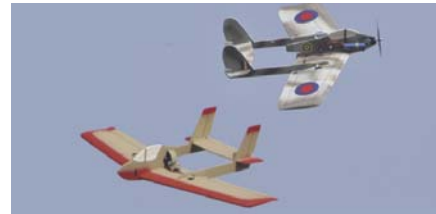
CD451 LEAF BLOWER Here are two models for the price of one! The Leaf Blower can be built as a deHavilland looking early jet with a standard brushless motor and prop or a sleek, modern sport jet with a 70mm fan unit. Either model builds up fast and easy. Models use pre-cut foam wing cores available through the Core House (article has details) while the rest of the model is built of sheet foam, balsa and plywood. Build both to have a pair of fun sport models for your new flying season. 39-inch wingspan, weighs 21 ounces ready to fly. Plan on one sheet. Dick Sarpolus FM 01-2013 $$$E
