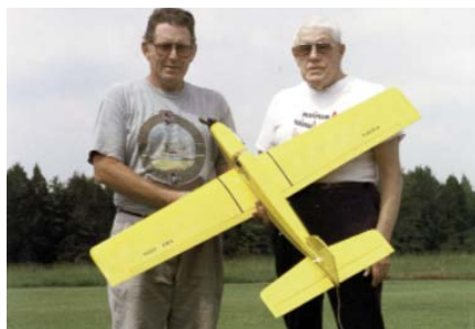
CF986 AERIOLE. Low wing R/C sportster with or without coupled throttle and flaps. 52-inch span, .15 to .20 eng., 4 channel gear. W. Winter and J. Hunton. FM 3-96. $$D
