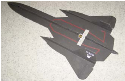
CD424 SR-71 . Known for clandestine operations throughout the Cold War, the SR-71 can now be an easy-to-build foam electric. Foam board or Depron and balsa construction. Wing span is 27¼ inches with 515 square inches of wing area. Flying weight is 20 ounces. Plan on one sheet. Laddie Mikulasko. FM 08-2011 $$$D
