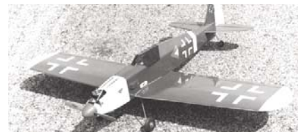
CF289 ME-109. 1/4 midget pylon racer with 39-inch span. For hot .15 eng., and 4 channel gear. J. Sheeks. FM 2-73. $$$
