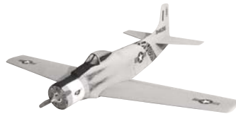
CD112 DOUGLAS AD-1 SKYRAIDER. This R/C semi-scale warbird is designed for Speed 400 electric power. On eight cells, it has pretty nimble performance. Wing span is 33¼ inches. Gus Morfis. FM 05-2000. $$D
