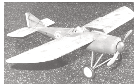
CF326 BRISTOL M1B. WWI Stand-Off Scale monoplane with 52-inch span. Uses 4 channels and a .40 eng. T. Eck. FM 3-74. $$D
