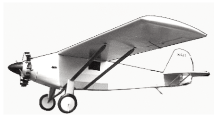
CF494 SPIRIT OF ST. LOUIS. Stand-Off 2-inch scale R/C model of Lindbergh's classic. 93-inch span, .40 to .71 eng., and 4 channel radio. D. McGovern and T. Lombardo. FM 1-79. $$L
