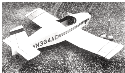
CF522 THORP T-18. Popular homebuilt design translates well into R/C Stand-Off Scale design for .60 eng. Has 62-inch span, and uses 4 channel units. T. Lombardo and D. Palumbo. FM 11-79. $$D
