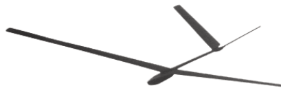
CF112 DANCER. Try this 144 inch span, pod and boom V-tail soarer for thermals. C. Lorber. FM 3-68. $$L
