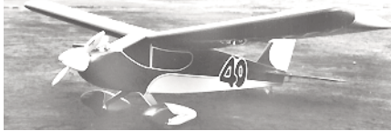
CF697 FAST FREDDY. Hot high-wing model for .40 eng. Spans 50 inches, and uses 3 channel R/C gear. F. Reese. FM 6-85. $$D
