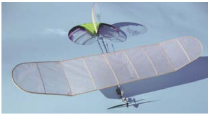
CD419 VAPOR ENDURE O 2 . Build it for R/C or F/F. built from the plans, the Endure is a great CO 2 endurance model or use the wing on a ParkZone Vapor for R/C endurance. 14.75-inch wing span, 80 square inches of wing area. Flying weight of 12 grams without battery. Plan on one sheet. Daniel Walton. FM 06-2011 $$$
