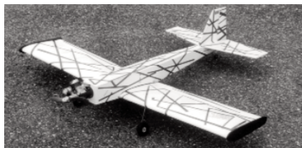
CF989 BEEP. .20 engine powered sport design with a 48-inch span; is built up from balsa and artist's foamboard. D. Woodward. FM 4-96. $$D
