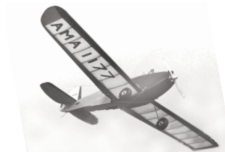
CF559 ZINGER. Two or three channel R/C low-wing fun ship for 1/2A engines. Has 32-inch span. H. Clukey. FM 2-81. $$B
