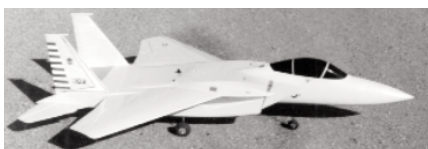
CF978 F-15 EAGLE. A single engine version of the famous jet fighter. Spans 41.5 inches, and requires a K&B 7.5cc engine in a Turbax-1 fan unit. Use five channel R/C gear. Plans on two sheets. I. Munninghoff. FM 11-95. SSL
