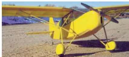
CD164 FAIRCHILD F24R An R/C electric powered sport scale model of the classic two seater. All balsa construction is designed to be extra light weight so that it would fly like a glider. Requires 4 channel radio with two micro sized servos. Uses a 6V Speed 400 and 2.3:1 gear drive. Finished weight ready to fly with batteries is 23 ounces. Wing span is 60 inches. Plans on one sheet. Pat Trittle. FM 05-2002 $$F
