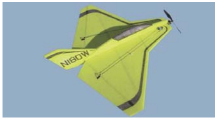
CD440 3D DYKE DELTA . The full scale Dyke Delta was a home-built airplane that was originally designed in the 1960's. This profile foam model is easy to build and will fly the full range of 3D maneuvers. Weighs 6.5 ounces, ready to fly, spans 32.5 inches and uses an E-flite Park 300 motor. Plan on one sheet. Daniel Walton FM 06-2012 $$$D
