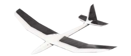
CD093 CLOUD DANCER. A straight forward two meter sailplane that loves to loiter and is easy to build. Offers three different wing styles. Wing span is 77 3/4 inches, fuse length is 39 1/2, finished weight is between 18-20 ounces with mini R/C gear. One plan sheet. Henry Haffke. FM 9-99. $$$D
