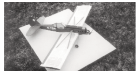
CD046 DEMIDUSTER. If you have a .10-.15 2-cycle engine looking for a home, here's a neat little R/C design that's patterned after the Piper Pawnee ag duster. Uses 3-4 channels and spans 44 inches. Tyrone Parker. FM 3-98. $$D
