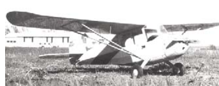
CF585 AERONCA CHAMP. R/C model of light plane favorite. .09 to .15 eng., 3 to 4 channel. 32-inch span, 52-inch length. Doc Mathews. FM 12-81. $$D
