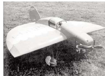
CF812 ARUP. Unusual R/C Scale flying wing design of the 1930's, 40-inch span. .35 to .40 size eng., 4 channel guidance. Plans on 2 sheets. A. Wolsky. FM 10-89. $$L
