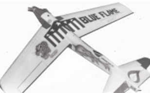
CF293 BLUE FLAME. Sport-Pylon R/C racer with 54-inch span, and 505 sq. in. wing area. For Schneurle .40 eng., and 4 channel gear. D. Gierke. FM 4-73. $$$
