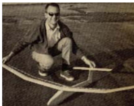
CF020 LIL T. A 74" span, rudder only, T-tail glider. B. Hahn. FM 6-65. $$H
