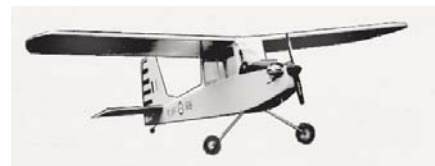
CF936 OBSERVER. Sport-scale version of high-wing military observation plane. Spans 57 inches; .20 4-stroke engine, and a 4 channel R/C system. A. McLeod. FM 7-94. $$D
