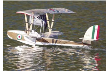
CD274 MACCHI M5. Electric R/C Scale amphibious airplane flown with a 3:1 geared Speed 400. Balsa and ply construction. The wing span is 52 inches and wing area of 534 square inches which provides a wing loading of 8.36 oz/sq.ft. Flying weight: 1 pound, 15 ounces. Plans on one sheet. Keith Sparks. FM 03-2006 $$ K
