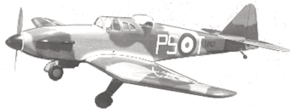
CF406 BOULTON-PAUL DEFIANT. R/C Stand-Off Scale British WWII fighter uses .60 eng., and 4 channel R/C gear. Has 60-inch span. D. Reiss. FM 5-76. $$D
