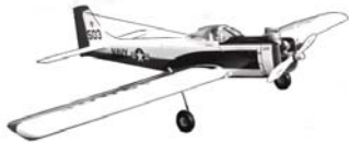
CF206 RAIDER. A 56-inch span semi-scale R/C ship for .40 eng. or larger. Uses 4 channel R/C gear. J. Sheeks. FM 3-71. $$C
