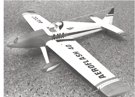
CF682 AEROFLASH 40. Spirited sport-pattern .40 design, 4 channel R/C. Uses foam core, 54-inch span. E. Ajamian. FM 12-84. $$D
