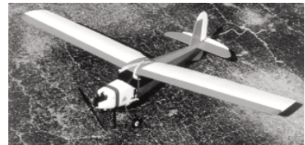
CF963 CLASSICAL GAS. Use the Cox E-Z Bee or Sundance ARF power pods in a 2-channel R/C funster. Spans 44 inches. R. Clough. FM 5-95. $$D
