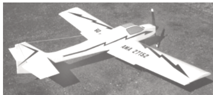
CF884 VOLTSWAGON. 72-inch span R/C sportster with .60 cobalt electric motor or .40 to .45 glow eng. Operating flaps. 5 channel gear. I. Munninghoff. FM 6-92. $$F
