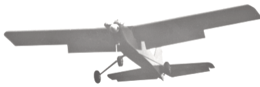
CF926 SWALLOW. With proportionally operated flaps. 56-inch span, .28 to .32 eng., 3 to 4 channel R/C. Plans on two sheets. W. Winter and J. Hunton. FM 3-94. $$L
