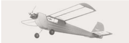
CF703 SEE-3. Reminder-scale version of Aeronca C-3 for training and fun. 37 inch span, .09-.15 eng., 3 channel radio gear. L. F. Randolph. FM 7-85. $$C
