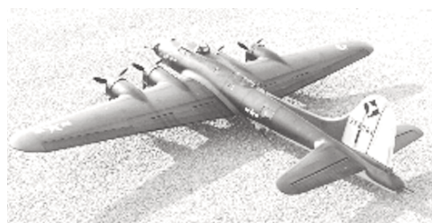
CF286 B-17G FLYING FORTRESS. Uses four .20 engs. and a 4 to 6 channel R/C system. First in '72 NATS flight achievement. T. Cook. FM 1-73. $$J
