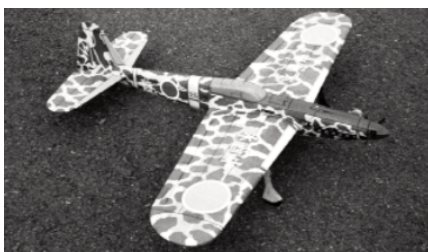
CF985 KAWASAKI Ki25SF. R/C Sport-Scale aerobatic version of the WWII Japanese fighter. Features optional retracts. 44-inch span, .25 size engine, 4 to 5 channel radio. T. Parker. FM 2-96. $$$
