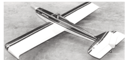
CD008 VOLTMASTER. Sizable electric R/C ship has performance and duration. All balsa with novel powertrain pull-out tray. Spans 69 inches, for 21 cells, ModelairTech H-1000 belt drive. Gene Rogers. FM 11-96. $$$D
