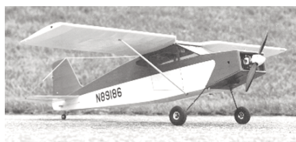
CF251 NESMITH COUGAR. Eyeball-Scale R/C with 54-inch span, .40 to .60 eng., 4 channel R/C units. S. Hines. FM 2-72. $$F
