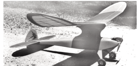
CF790 DUSTY. R/C freeflight sport model in tradition of the 1940's. Features a pylon mounted 66-inch wing, uses 3 channel radio and .09 to .15 eng. D. Fortuna. FM 1-89. $$D
