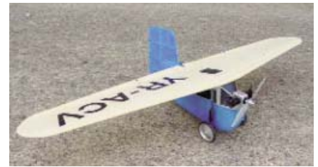
CD223 STABILOPLAN IV A R/C semi-scale electric powered homebuilt aircraft. It's basically a flying wing with a big trunk, and as the name implies, it is very stable in flight. Light weight balsa construction, it can be powered with a brushed or brushless motor system. For three channel control. Its wing spans 44¼ inches. Weight is 15.1 ounces. Plans on one sheet. Dick Miller. FM 05-2004 $$C
