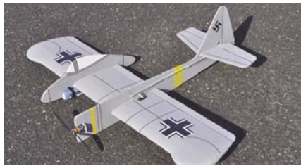
CD448 BLOHM & VOSS P.179 . Dick Sarpolus designed this odd looking model to build up from sheet Styrofoam, balsa and plywood. The unique wing is fully symmetrical thanks to the hot wire cut foam core wing. The B&V P.179 features a 42-inch wingspan, weighs 26 ounces ready to fly and requires a four-channel radio with three micro servos, a 120-150 Watt brushless motor, 20-amp ESC and a 3S 1800-2200 mAh Li-Po battery pack. Plan on one sheet. Dick Sarpolus FM 11-2012 $$$C
