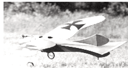
CF321 TAUBE. Stand-Off Scale WWI R/C design, 84-inch span. Uses 3 to 4 channel R/C gear. Plans on 2 sheets. N. Zirolì. FM 1-74. $$L
