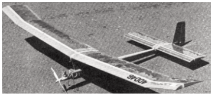
CF459 THE HUNGRY EAGLE. R/C duration model with freeflight looks. For .40 eng., and 2 channel. Features 96-inch span. D. Sarpolus. FM 1-78. $$$
