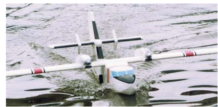
CD124 CANADAIR CL-415 An R/C semi-scale water bomber designed for two geared Speed 400 motors to power this distinctive R/C ship. It can fly equally well from water or from grass, without gear. Its wing spans 63¾ inches, and weighs just 72 ounces. Balsa and hardwood construction. Plans on one sheet. Laddie Mikulasko. FM 12-2000 $$F
