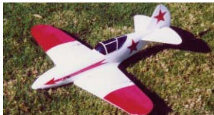
CD182 MIG-3 An R/C electric for AMA 704 Combat. Balsa and plywood construction, fully sheeted to take the beatings of landing without wheels. With a wing of just 30½ inches, the finished weight is 16 ounces. Power is provided by a Speed 400 motor on a 7-cell pack. Plans on one sheet. Gus Morfis. FM 11-2002 $$C
