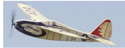
CD456 AJ 404 INTERCEPTOR . Based on the AJ 404 Interceptor from the American Junior freeflight glider of 1947, this R/C version boasts a larger size and a better possibility of staying out of treetops. Pat Tritle has designed this sport electric model for an E-flite Park 180 brushless motor and the micro servos, ESC and receiver from the Great Planes micro F-86. The model spans 30 inches and weighs 3.3 ounces ready to fly. Plan on one sheet. Pat Tritle FM 07-2013 $$$B
