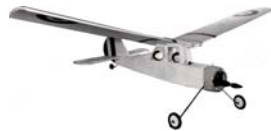
CF931 MORLES 1915. Featuring foam board and balsa construction, this scale-like 1/2A R/C funster is easy to build. Uses two channel gear, 43-inch span. Plans on two sheets. R.L. Clough, Jr. FM 5-94. $$J
