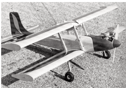
CF438 REISS ROOSTER. R/C sport-biplane, 48-inch span, rolled plywood fuselage. .61 eng., 4 channel R/C. D. Reiss. FM 5-77. $$D
