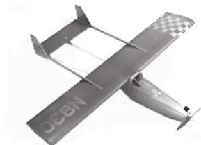
CF340 LIT SPECIAL. A 1/2A twin-boom R/C Pylon Racer for Cox Tee Dee .049 eng., 31-inch span. V. A. Calouri. FM 8-74. $$$
