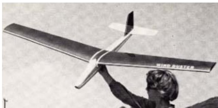
CF658 WINDUSTER. Two-meter R/C glider for slope or thermal flying. Balsa covered foam core wings. B. Evans. FM 2-84. $$$C
