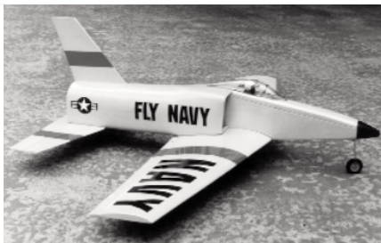
CF953 ELECTRA VIPER. Speedy easy-to-build electric ducted fan design for Astro Lite 15 motor. Spans 50 inches, balsa & foam construction. E. Brightbill. FM 1-95. SSD
