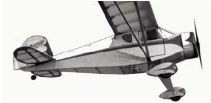
CF631 SYS MONOCOUCPE. Schoolyard classic R/C for single channel pulse or micro multi-channel. 36-inch span, .020 eng., 3 channel unit. J. Kostecky. FM 5-83. $$B
