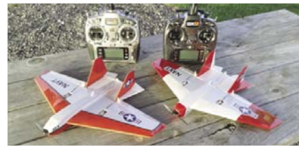
CD461 SHRIKE 180 . The Shrike 180 is a micro version that is based on Joe Beshar's 1980's sport flying hot rod. The average modeler can build the Shrike 180 over the span of the weekend, making it a fun group build. Spans 18.75 inches and weighs 2.5-3.5 ounces ready to fly. Uses a Spektrum AS6410NBL RX/ESC, two Spektrum SPMSA2030L and three 2.3-gram linear ultra micro servos for the elevator and ailerons. Plan on one sheet. Andy Kunz FM 11-2013 $$$A
