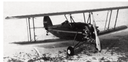
CF701 WACO CSO. 62-inch span R/C biplane, 4 channel radio, 90 four stroke power. Plans on 2 sheets. D. Watz. FM 7-85. $$L
