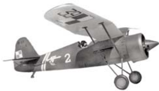
CF617 POLISH P.IIC FIGHTER. Distinctive 1/2A gull wing design of Polish fighter of late '30s. Has 40-inch span, 2 to 3 channel R/C. C. Nagy. FM 12-82. $$C
