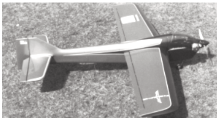
CF229 RAMPANT. Toledo R/C pattern class winner, features tandem retract gear. For .60 eng and 5 channel R/C gear. Features 62-inch span. J. Worth. FM 7-71. $$F
