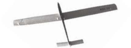
CF369 BOMMEL. Giant 114" span R/C soarer with full wing flaps. P. Keim. FM 5-75. $$F
