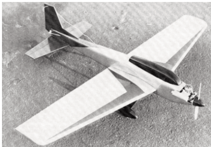
CF653 FASER. A 48-inch span Sport-Pattern ship for use with .21 to .25 eng., and 4 channel gear. A. Trapanese. FM 1-84. $$D
