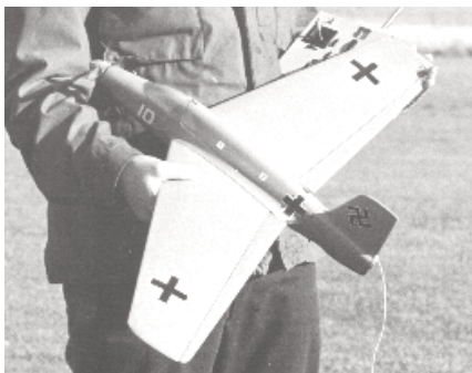
CF574 ME-163 KOMET. 1/2A R/C Sport-Scale version of German WWII rocket plane. .049 eng., 3 channel systems. Spans 33 inches. A. Adamisin. FM 8-81. $$B
