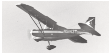
CF353 CITABRIA PRO. Stand-Off Scale R/C design for .60 eng., 63-inch span, 4 channel equip. B. Godfrey. FM 12-74. $$J
