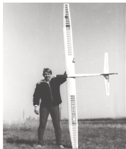
CF208 SABRE SOAR. This 125" span R/C soarer features Eppler 385 airfoil. It's a big one! N. Liptak. FM 4-71. $$D
