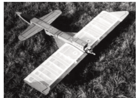
CF964 WHICH WAY? 1/2A 3 channel R/C canard for great aerobatics. 36¾-inch span. T. Parker. FM 6-95. $$D
