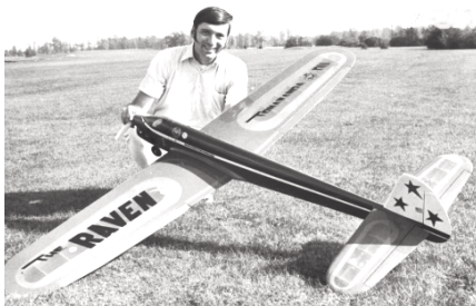
CF220 BRAZEN RAVEN. Large, 84-inch span Sport-Pattern R/C design for .60 eng., and 4 to 5 channel R/C gear. Plans on 4 sheets. D. Gierke. FM 5-71. $$Q
