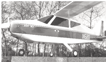
CF380 BD-6. Stand-Off Scale R/C design for .19 to .35 eng., and 4 channels. Features a 56-inch span. B. Aberle. FM 9-75. $$D
