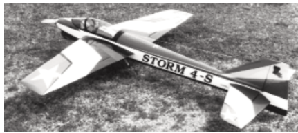
CF980 STORM. Top caliber FAI R/C Pattern ship features foam surfaces, built-up balsa fuselage. 78-inch span, 1.20 4-cycle engine, 5 to 8 channel R/C. Plans on three sheets. B. Hebert. FM 12-95. $$R
