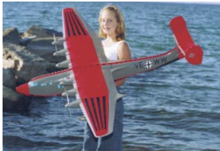
CD091 POTEZ-CAMS 161. Designed for six Speed 400 motors, powered by two 10-cell 1700 mAh batteries. Construction is mostly foam, with some balsa. It qualifies as IMAA legal at 80-inch span. The 3-sheet plan includes all templates, motor and battery circuit, and a detailed isometric. Laddie Mikulasko. FM 8-99. $$R
