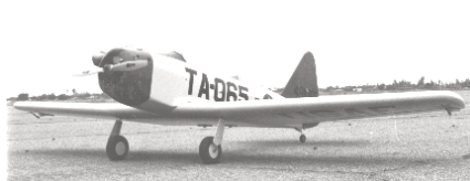
CF771 AT-6 TEXAN. R/C Sport-Scale version of famous trainer. Features foam core 66-inch wing. For two stroke .60 eng., and 4-channel radios. D. Reiss. FM 3-88. $$$
