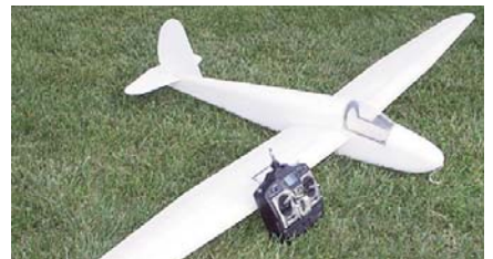
CD305 SCHWEIZER 1-23 STANDARD. An R/C scale glider, constructed of expanded polypropylene foam and sheet balsa. This plane has an SD 7037 airfoil, with a 57 1/2-inch wing span, wing area of 587 square inches, length of 57 1/2 inches and weighs 48 ounces, that gives this glider a wing loading of 13 ounces per square foot. Plans on two sheets. Thomas J. Martin. FM 03-2007 $$$L
