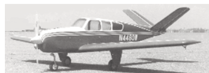
CF579 BONANZA. R/C Sport-Scale version of famous Beechcraft design. .60 eng., 4 to 5 channel systems. Spans 59 inches, uses foam core wings. D. Reiss. FM 10-81. $$D
