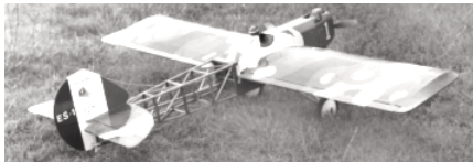
CF898 CAP'N EDDIE'S SCOUT. 57-inch span Semi-Scale design. Takes 4 stroke .40-48, or 2 stroke .29-.35 eng., 4-channel radio. B. Shepherd. FM 1-93. $$F
