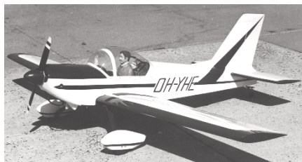
CF719 PIK-15. Giant Sport-Scale Finnish lightplane. All sheet balsa fuselage, foam core flying surfaces. 89-inch span uses Quadra Q-35 eng., and 4 or 5 channel radio. Plans on 2 Sheets. D. Sarpolus. FM 3-86. $$Q
