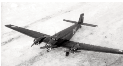
CD011 JU-52/3M. R/C stand-off scale transport is powered with single .40-.45 2-stroke for center engine. Spans 71 1/2 inches, length 45 1/2 inches. Pavel Bosak. FM 12-96 $$$
