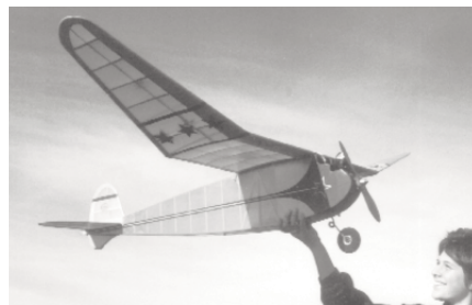
CD47 RAMBLER. Refined version of the Gil Shurman freeflight Old Timer, with mods for a more powerful Super Cyclone engine and a pop-up stab dethermalizer. 69-inch span. Plans on two sheets. B. Augustus. FM 3-98. $$ L
