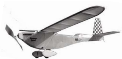
CF928 SKYSCRAPER SPECIAL. Embryo Endurance F/F rubber design inspired by old Scientific Skyscraper. Spans 24½ inches, wing type dethermalizer. M. Fineman. FM 3-94. $$ A.
