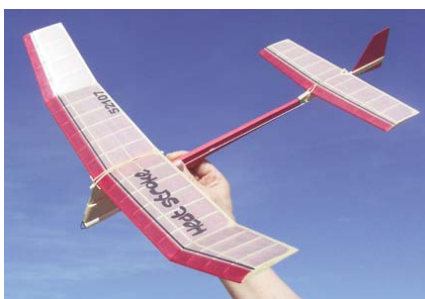
CD307 THE HEAT STROKE. This design for Rapier/Jetex duration events is constructed of stick and tissue. It has an HLG airfoil with a 20-inch wing span, wing area of 61 square inches, length of 18 \frac{3}{4} inches and weighs 20.2 grams, which provides a wing loading of 0.33 ounces per square foot. Plans on one sheet. Larry Kruse. FM 03-2007 $$ A
