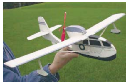
CD230 REPUBLIC SEABEE A "fat" freeflight No-Cal model of the stalwart amphibian. All balsa sheet construction. It can be powered with either CO 2 , as tested, or electric power. Spans 29 inches; finished weight is 43 ounces. Plan on one sheet. Tom Sandor. FM 08-2004 $$ B
