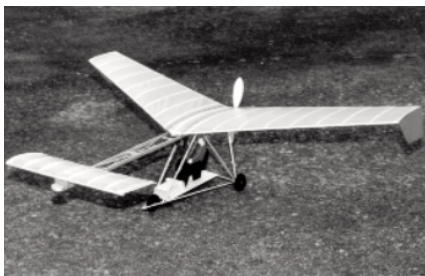
CD010 EAGLE X/L. Made largely from dowels, this graceful electgrid freeflight model is a scale version of a real ultralight. Spans 28 inches and is 19½ inches long. Uses a HiLine Mini-6 motor. Al Flesher. FM 11-96. $$ B
