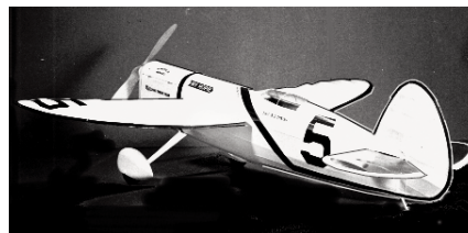
CF674 MY HOPIE. 21½-inch span CO 2 Golden Era racer features plug-in wings and motor module. R. Theiss. FM 9-84. $$ B
