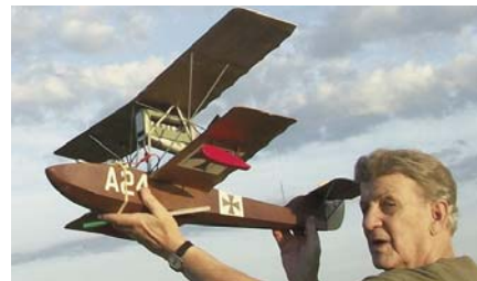
CD433 HANSA-BRANDENBURG CC. A perfect model for Power Scale, the full scale aircraft was an early flying boat and was designed by the Germans in 1917. The aircraft is characterized by its unique star-strut interplane bracing and single pylon mounted engine in pusher configuration. The model features scale construction and uses an electric motor for power. Weighs 7.9 ounces ready to fly, spans 31.5 inches. Plan on one sheet. Tom Sandor FM 02-2012 $$ C
