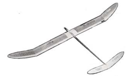
CF209 ATHENA. 80" span Nordic A/2 with glass fuselage. Open class winner '66 NATS. R. Simpson. FM 3-67. $$ C
