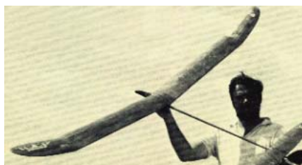
CF176 SCARAB. A2 Nordic F/F with 79" span. Fiberglass fishing rod fuselage. R. Mathis. FM 10-69. $$ C
