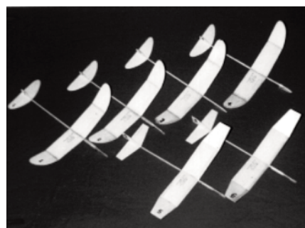
CF973 HECKIZZIT. All sheet balsa catapult glider with 16" span. Easy to build and fly. M. Keville. FM 9-95. $$ A
