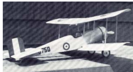
CF770 BRISTOL SCOUT D. All sheet balsa "Fun Scale" freeflight biplane, 30-inch span. .049 eng. D.B. Mathews. FM 2-88. $$ C
