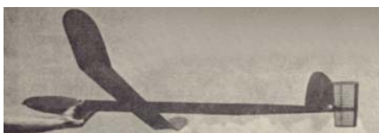
CF091 SOUTHERNER. Unlimited rubber design with folding prop, high aspect ratio 52-inch span wing. R. Simpson. FM 8-67. $$ C
