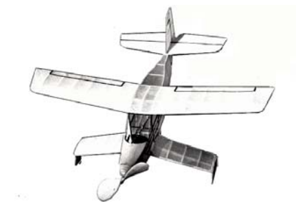
CF626 NEGABIPE. Unique rubber powered biplane with negative stagger planform, conforms to Bostonian F/F competition rules. Has 16-inch span. J. Tudor. FM 3-83. $$ A
