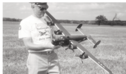
CD036 B-24J LIBERATOR. For the multi-engine freeflight scale fanatic, 55" span uses cracked rib technique to keep weight to eight ounces without motors. 35-40-sec. flights. Dennis O. Norman. Plans on two sheets. FM 9-97. $$ J
