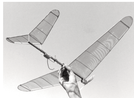
CD125 OUT-OF-DOORS INDOOR MODEL An electric powered freeflight sport model for those calm, leisurely evenings made for flying enjoyment. Wing span is 26½". Finished weight is 1¼ ounces with three 50 mAh batteries. Balsa and bamboo construction. Plans on one sheet. Roy L. Clough Jr. FM 12-2000 $$ A
