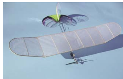
CD419 VAPOR ENDURE O 2 . Build it for R/C or F/F. Built from the plans, the Endure is a great CO 2 endurance model or use the wing on a ParkZone Vapor for R/C endurance. 14.75-inch wing span, 80 square inches of wing area. Flying weight of 12 grams without battery. Plan on one sheet. Daniel Walton. FM 06-2011 $$ A
