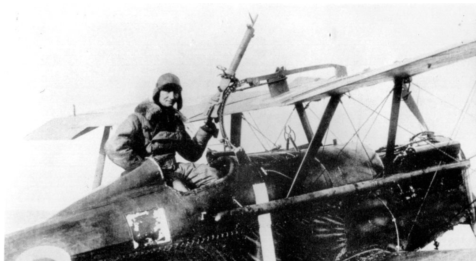
Tutschek sitting on the cockpit edge of his penultimate victory, number twenty-six, on 5 March 1918. An SE.5A (C1057) from 24 Squadron, its pilot was captured. Tutschek is demonstrating how the wing Lewis gun could be pulled towards the pilot, both for upward firing, and for changing an ammunition drum. The drum here is not in place, and note the different design of the Vickers' gun-sight.
