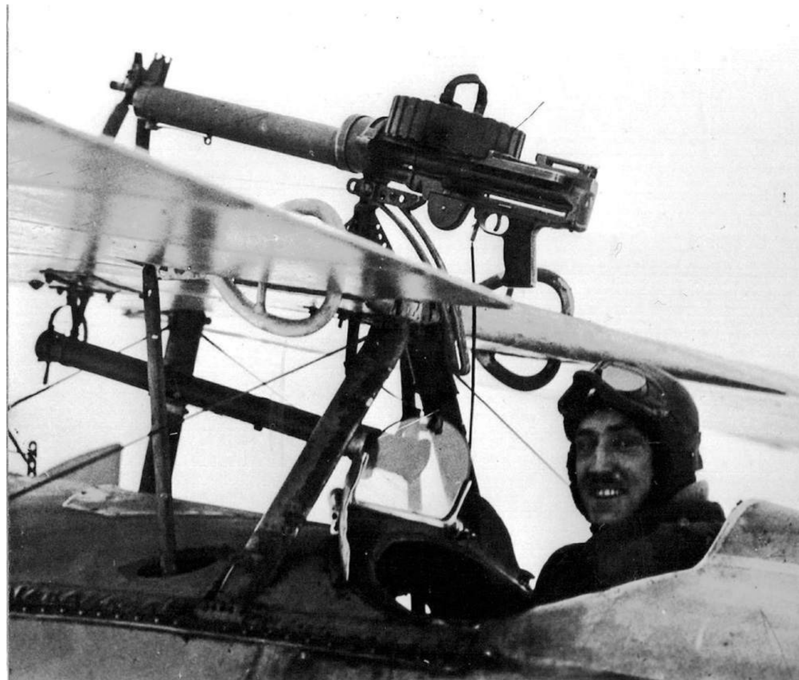
The RFC continued to fly the French Nieuport Scouts in 1917. This No. 1 Squadron machine, with Captain W. W. Rogers in the cockpit, clearly shows the wing-mounted Lewis gun and the cable that allowed the pilot to fire it. Also clearly seen is the telescopic sight giving the pilot every chance of scoring against an opponent ahead of him. Wendell Rogers, a Canadian, received the MC for his air fighting, ending 1917 with nine victories. Included in his score was a Gotha bomber which he shot down in daylight on 12 December.
