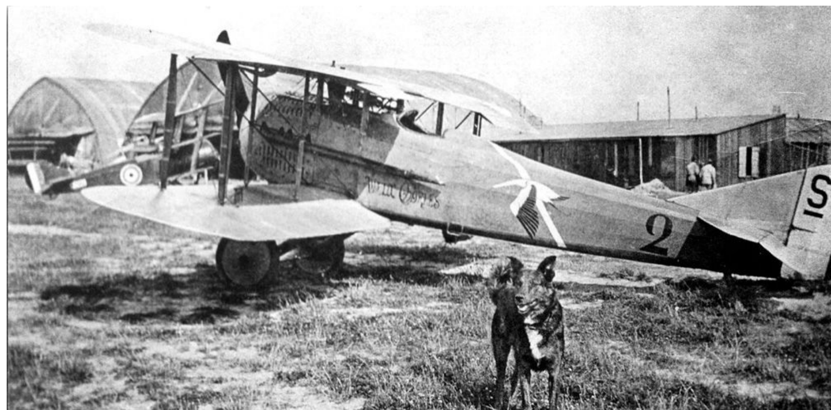
One of the Spad VII fighters used by Guynemer. Again we see the Stork emblem of Escadrille N3 . Each escadrille in the group carried a Stork emblem, but in different designs. Beneath the exhaust pipe is written Vieux Charles , the name carried on all of his Nieuport and Spad aircraft. The number '2' is in red. Note the RNAS Sopwith Triplane in the background.
