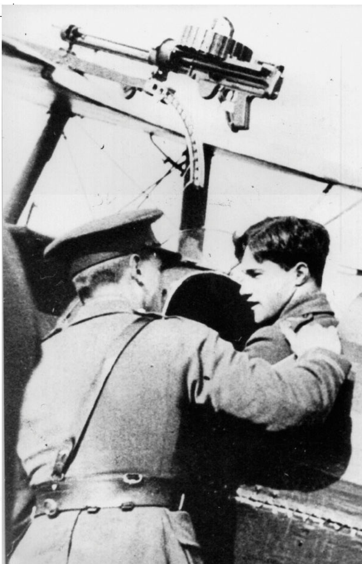
Captain Albert Ball DSO MC seated in his 56 Squadron SE.5 at London Colney shortly before the squadron moved to France on 7 April 1917. Note the Lewis gun on the top wing, fixed to fire over the arc of the propeller. The SE.5 also had a single Vickers gun in front of the pilot, firing through the propeller. The previous year, Ball had become proficient in sneaking up on German two-seaters from below in Nieuport Scouts and, by pulling down the wing Lewis gun, was able to surprise his opponents by firing upwards into their machines. As senior flight commander with 56, his victory score was already over thirty. In one month he raised this score to forty-four but was killed in early May.
