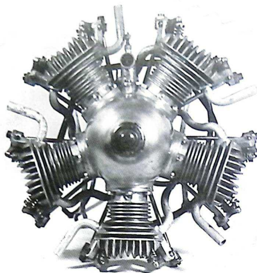
1945 Morton M-5 4 stroke ign. Made at Omaha, Nebraska. Later built by Burgess Battery Co, of Illinois
