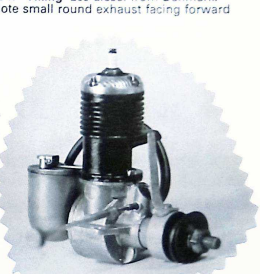
Late 1944 Vivell .35. Manufactured by Earl Vivell, San Francisco. Note stamped sheet metal timer arm
