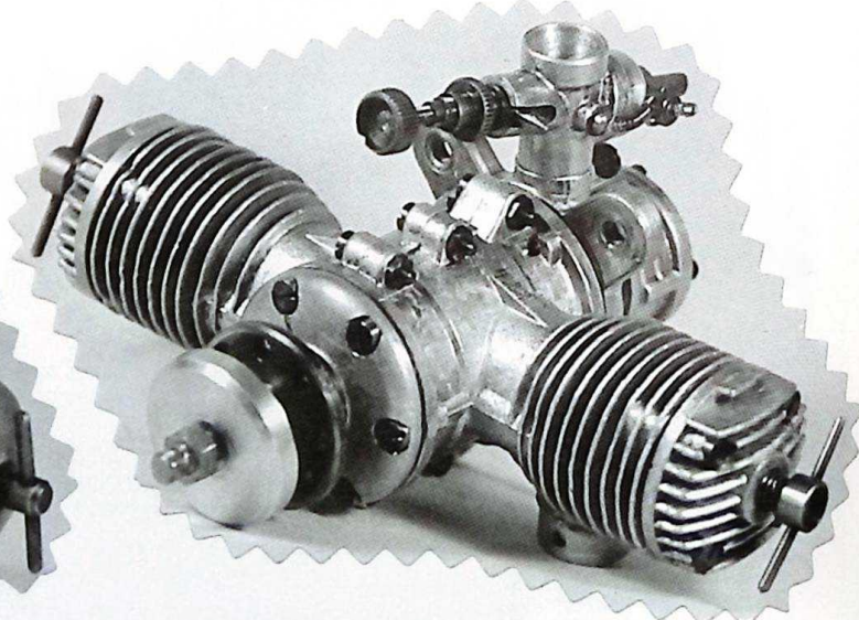
7.6cc twin by Webra in 1958. Previously designed and built by 'Ruppert' at 8.5cc capacity
