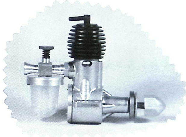
Gordon Burford, of Taipan engine fame, produced a run of 'copy' Mills .75 in 1974. Known as the ' Doonside Mills .75'. The Series I is shown above. The Series II is shown below. Note the case strengthening webs. The cylinder heads were anodised various colours.
