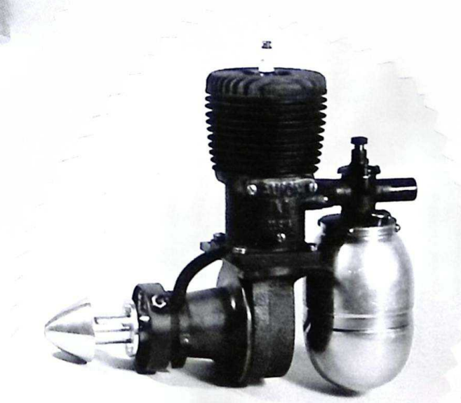
Avion Mercury '45' 1.6 cu.in. or 26.25cc and only 20ozs. This 1947 example is made from magnesium castings
