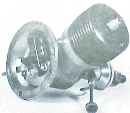
Another view of the Micron 10cc ign. , showing how well the points are kept clear of oil and dirt.
