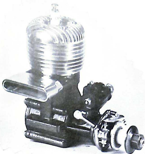
Seventy Seven Products U.S.A. Custom built ign. engine, using Merco .61 parts. This example finished with blue crank case, polished head and gold plated timer assembly
