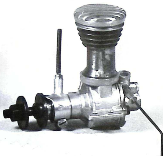
Ouragan 3.3 rear drum induction, from 1949. Quite an advanced induction system for its time
