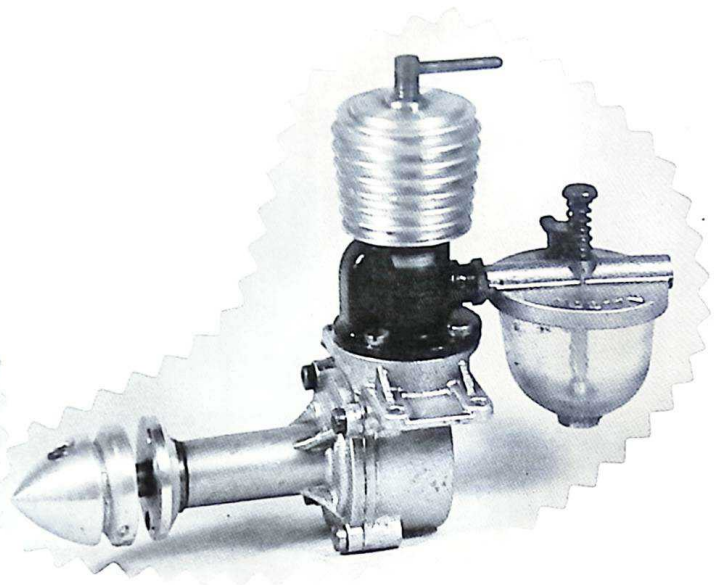
Allbon 2.8cc Produced in Bedfordshire in 1948. Ball bearing shaft version shown. Most were plain bearing
