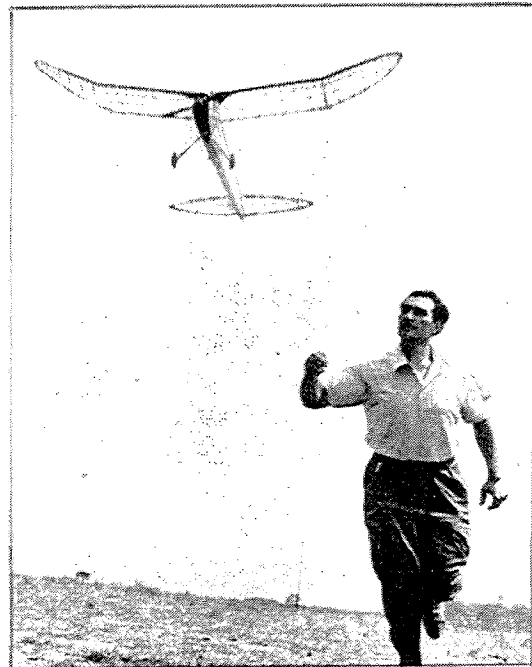
Test glide. Dodger has proper incidences built in, no side thrust, slight downthrust. Climbs wide left circle, glides sharp left circle.
