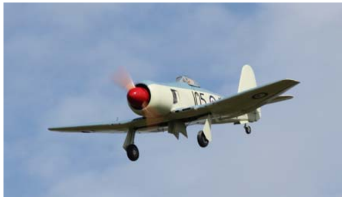
Brian Hutchinson's Hawker Sea Fury is scratch built from the Jerry Bates plan. At 1/5 scale it has a wingspan of 2.4m and is powered by a 3W 110 twin cylinder two stroke petrol engine. The wings have a hydraulic powered folding system.
