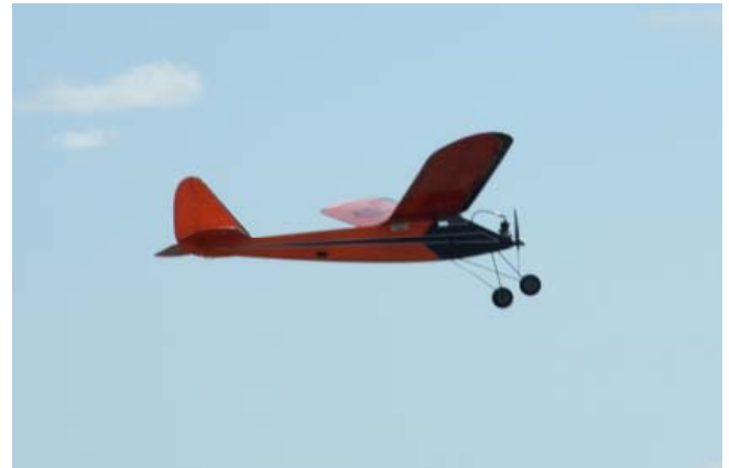
Brian Laughton's "RC1" powered by an OK Super 60 spark ignition engine.
