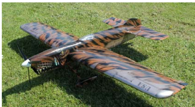
P.J. Rowland's "Tiger", 1.6m wingspan and powered by a PA75 engine.
