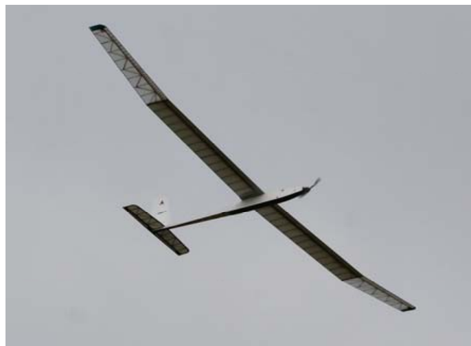
Tedium E7 in flight and showing the delicate structure of the high aspect ratio wing.
