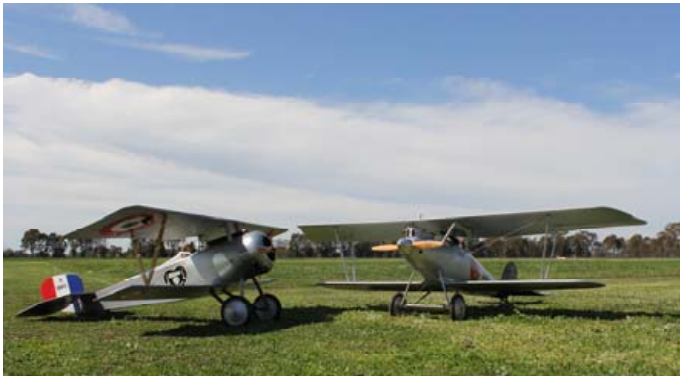
Colin Mitchell's Nieuport 17 and David Foster's Pfalz D.III. The 1/4 scale Nieuport is built from a Balsa USA kit and powered by an OS120 four stroke engine. David's Pfalz is scratch built, also to 1/4 scale, and powered by a Saito 180 four stroke engine.
