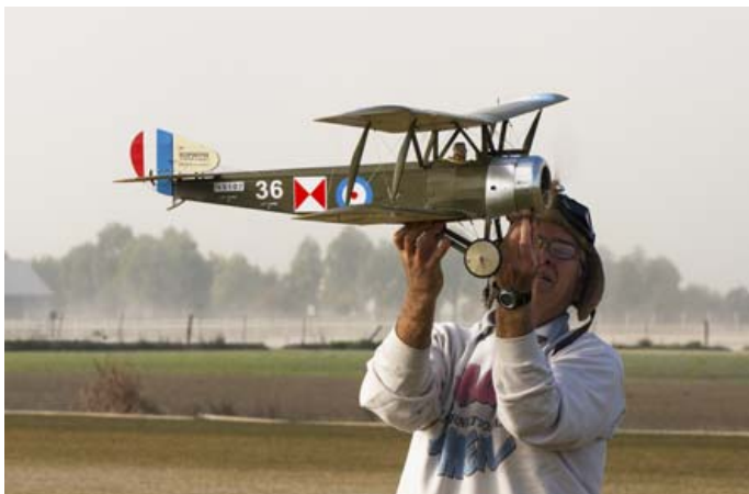
Phil Mitchell prepares to launch his Mills 1.3 diesel powered Sopwith 11/2 Strutter. A lot of down thrust but the Mills wasn't quite up to the job.
