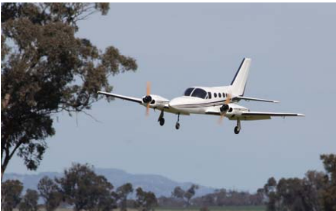
This large Cessna 421 Golden Eagle was flown by Gary Schmedje. Model is 27% scale with a wingspan of 3.4m and was scratch built from plans by Wendell Hostetler. Powered by two Zenoah 62 two stroke engines, it weighs in at 24.5kg.
