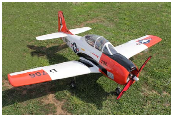
Paul Holland's T-28 Trojan is an ESM ARF. With a wingspan of 2m and powered by DLE 35cc petrol engine, it weighs 8kg.
