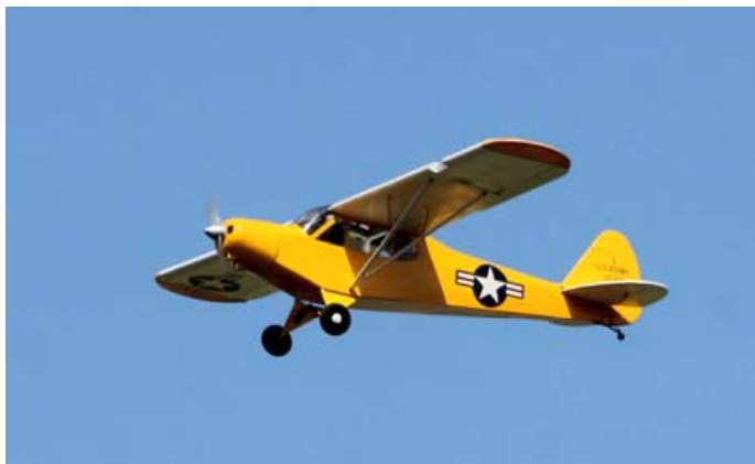
Derek Slevin's 1/4 scale Super Cub is a VQ ARF powered by a Saito 150 four stroke engine. Model weighs 6.5kg.
