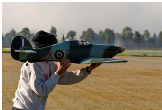
Tahn Stowe launching his Hawker Hurricane, this large model is powered by a vintage ED 3.49cc diesel engine.
