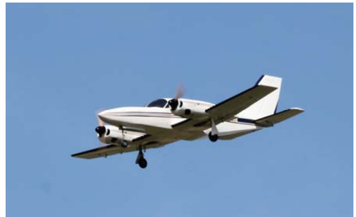
This large Cessna 421 Golden Eagle was flown by Gary Schmedje. Model is 27% scale with a wingspan of 3.4m and was scratch built from plans by Wendell Hostetler. Powered by two Zenoah 62 two stroke engines, it weighs in at 24.5kg.
