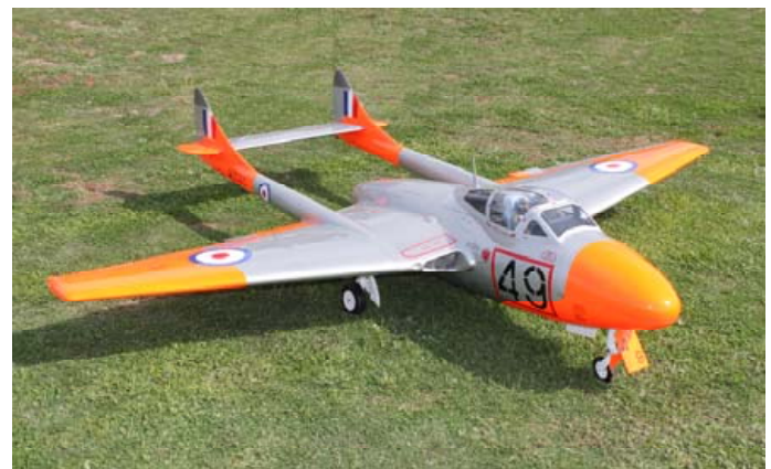
This ARF De Havilland Vampire by Fly Eagle Jets was flown by Scott Matthews. Model is 2.4m wingspan and powered by a Kingtec 140 turbine. Weight is 24kg.
