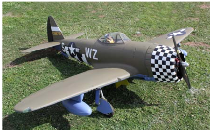
This P-47 Thunderbolt flown by Paul McCarthy is a Robart ARF from the Zirolì plan. With a wingspan of 2.4m and powered by a Saito 80cc three cylinder radial engine converted to petrol operation, it weighs 18kg.
