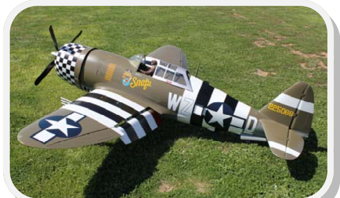
Garry Bergen usually brings his 1/3 scale Stearman to Shepparton but this year he also had this P-47 Thunderbolt. The model is a COMP ARF and has a wingspan of 2.8m. Powered by a Moki 250 five cylinder radial engine driving a 30" four blade propeller, it weighs 49.7kg.
