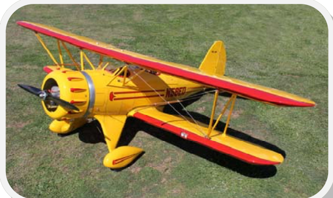
A Golden Oldie from the 1930's, Terry McCleary's WACO YMF-5 is built from a kit produced by Peter Barth in Germany. The model is 1/3 scale with a wingspan of 3m and is powered by a DA150 twin cylinder petrol engine driving a 32" x 12" propeller. Covering is SIG Koverall and it is finished with 2-pack epoxy paint. Weight is 24.5kg.
