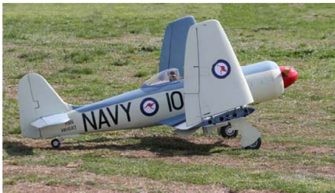
Brian Hutchinson's Hawker Sea Fury is scratch built from the Jerry Bates plan. At 1/5 scale it has a wingspan of 2.4m and is powered by a 3W 110 twin cylinder two stroke petrol engine. The wings have a hydraulic powered folding system.
