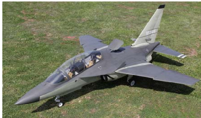
Theo Arvanitakis' AerMacchi 346 is a C&C Models ARF. Model spans 2m at 1/5 scale and is powered by a Jetcat 140 turbine. Weight is 15kg.
