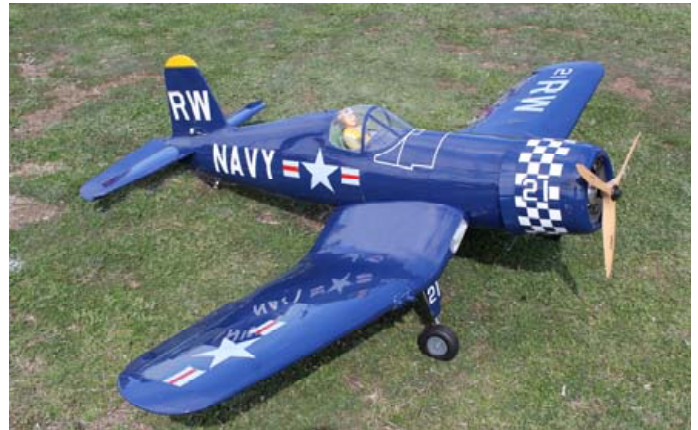
Flown by Neil Addicott of Model Engines, this ARF Corsair by Phoenix is 2.2m wingspan at 1:5.5 scale and powered by an OS five cylinder radial engine.
