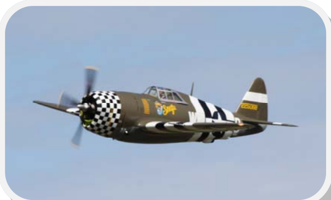
Garry Bergen usually brings his 1/3 scale Stearman to Shepparton but this year he also had this P-47 Thunderbolt. The model is a COMP ARF and has a wingspan of 2.8m. Powered by a Moki 250 five cylinder radial engine driving a 30" four blade propeller, it weighs 49.7kg.
