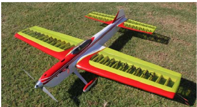
Doug Grinham's "Starcraft" is electric powered with a wingspan of 1.5m.
