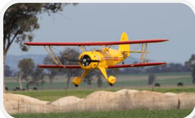
A Golden Oldie from the 1930's, Terry McCleary's WACO YMF-5 is built from a kit produced by Peter Barth in Germany. The model is 1/3 scale with a wingspan of 3m and is powered by a DA150 twin cylinder petrol engine driving a 32" x 12" propeller. Covering is SIG Koverall and it is finished with 2-pack epoxy paint. Weight is 24.5kg.
