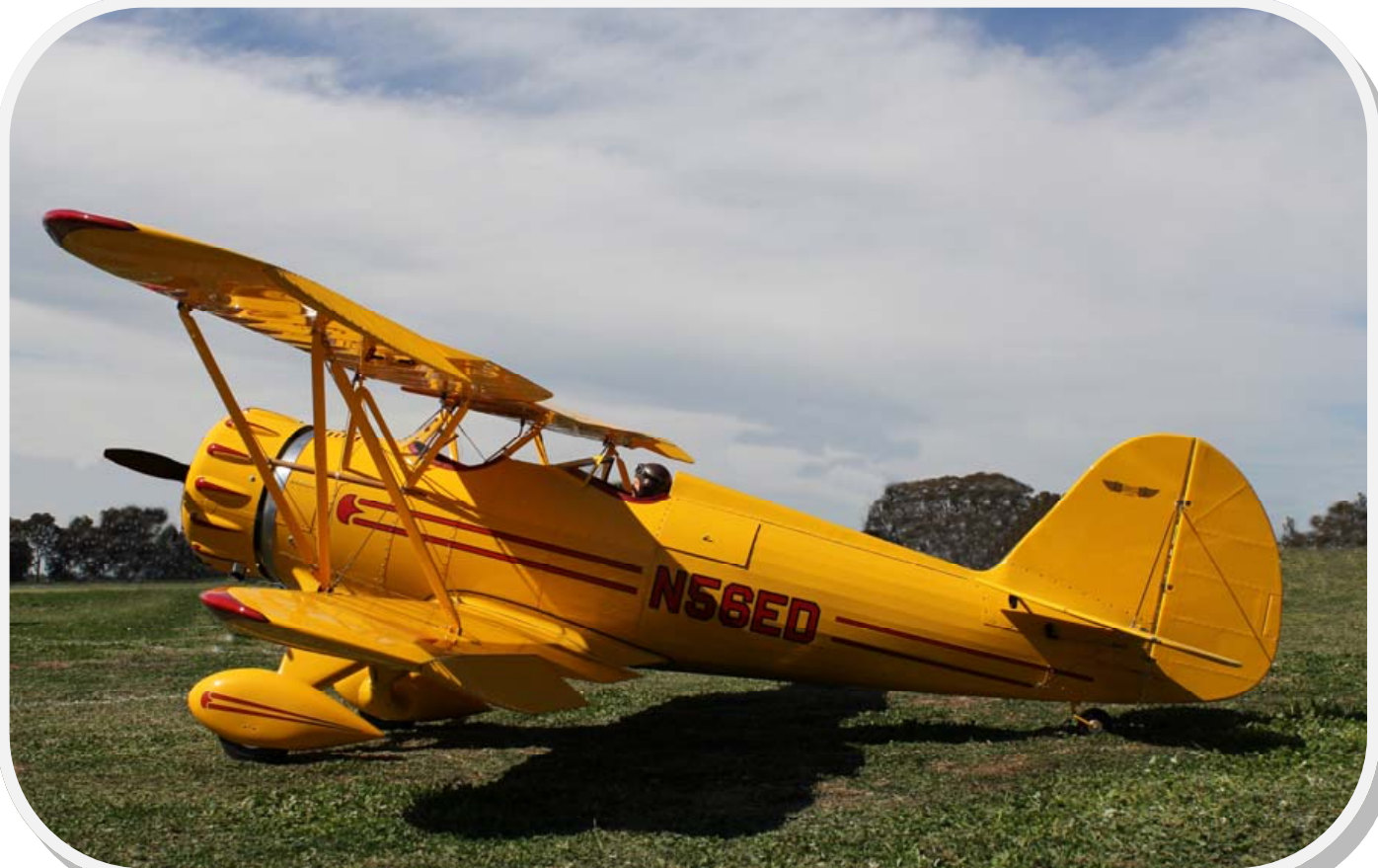
A Golden Oldie from the 1930's, Terry McCleary's WACO YMF-5 is built from a kit produced by Peter Barth in Germany. The model is 1/3 scale with a wingspan of 3m and is powered by a DA150 twin cylinder petrol engine driving a 32" x 12" propeller. Covering is SIG Koverall and it is finished with 2-pack epoxy paint. Weight is 24.5kg.
