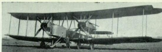
*F9569*, first Vimy to have Rolls-Royce engines. In this view the shape of original radiators can be seen. Below: *F9569* had enlarged rudders and pointed side fairings on engine nacelles.
