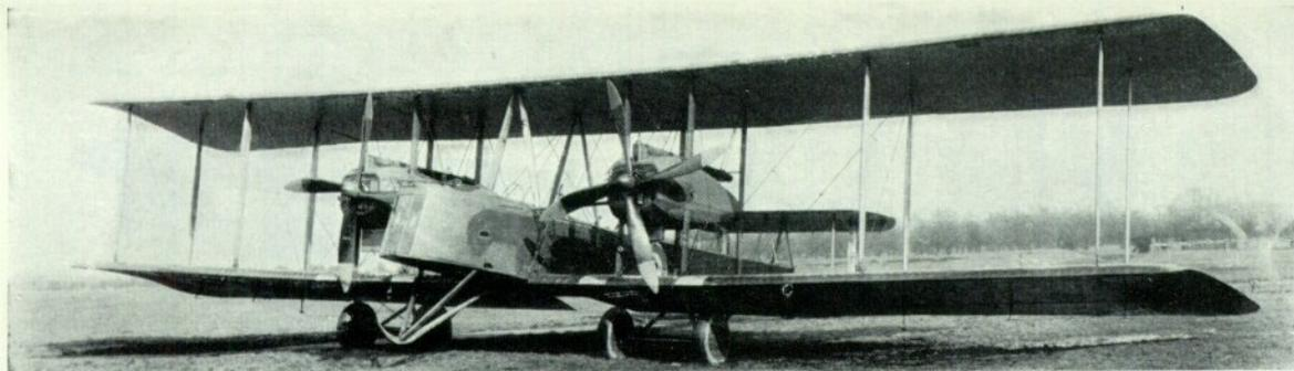
The second prototype, B9953, with Maori engines and inversely tapered ailerons. Below: Details of B9953's central fuselage.
