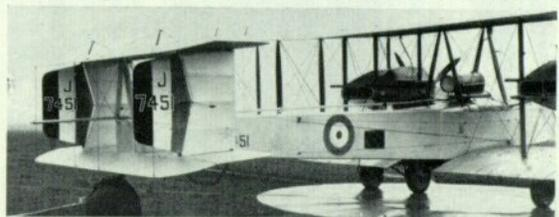
but distinguished by their twin exhaust pipes and four-blade left-hand airscrews. As on *B9954*, the water header tanks were in the centre section, but they were located centrally above the engines and their water-supply and vapour-release pipes were midway between the struts.
