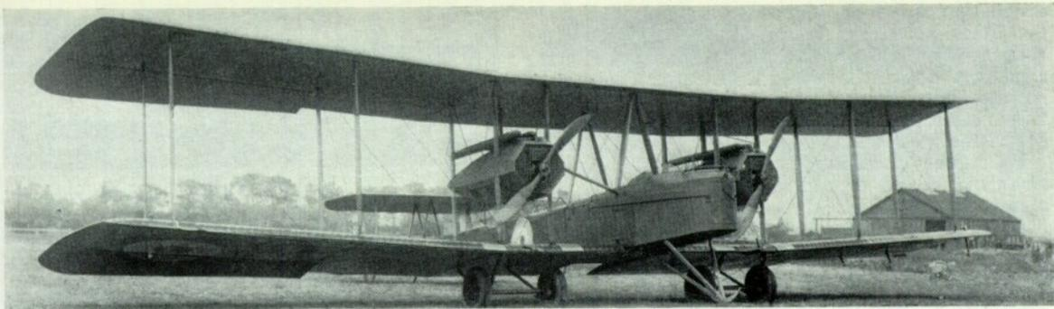
*B9954 in its original form with inversely tapered ailerons.*
