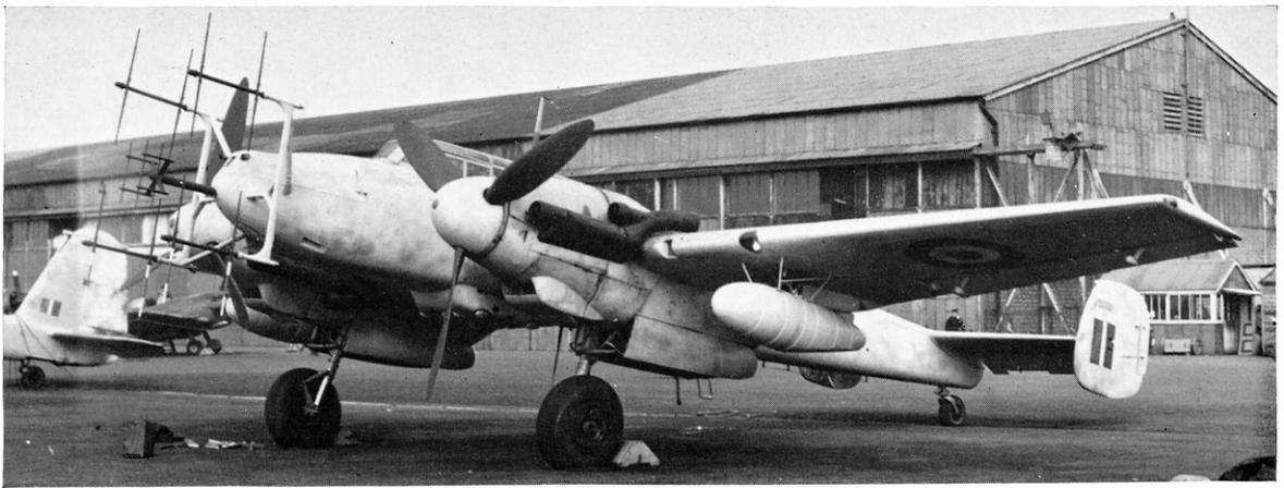
A captured Gf 110G-4/R7 night fighter. Note drop tanks, fuselage bomb racks and radar array. (Photo: Imperial War Museum)
