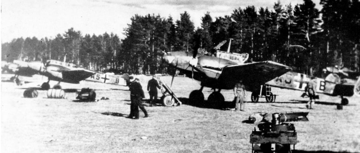
*Bf 110s of Schlachtgeschwader 1 dispersed in a Russian clearing. The two nearest machines, A 5 + E B and A 5 + H B, are aircraft of the 1st Gruppe staff flight. The yellow belly-band near the tail indicates service in the North and Central Russian zones. The under wing-tips were also painted yellow.*
