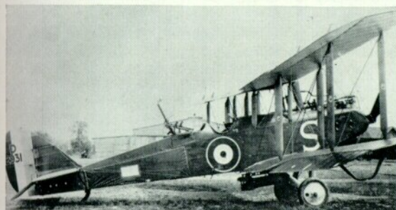
Left: D2931 fell into German hands intact during August 1918. It is here seen on the aerodrome of Jasta 78, with a 230-lb. bomb still in place on the rack under the fuselage. Although squadron markings for bomber squadrons were officially discontinued after March 1918 this aircraft still had a small white rectangle painted on the rear fuselage. (Photo: Egon Krueger.) Right: D2825 with frontal radiator, overwing gravity tank and arrester gear clips on the undercarriage spreader bar. The aircraft is here seen aboard H.M.S. Eagle in the course of deck-landing trials conducted during 1921.
