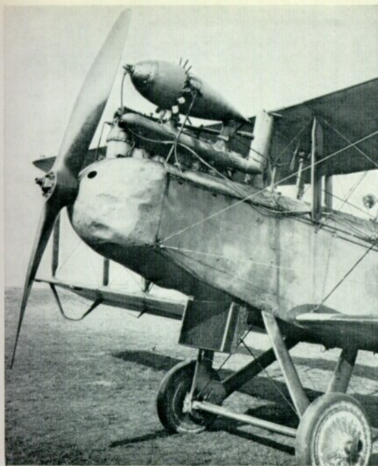
D.H.9 fitted with an early version of the Birger Ad Astra silencer, here seen at Farnborough on 24th April 1921. The Birger silencer that was demonstrated on a D.H.9C at Stag Lane late in 1921 was of an improved type and was mounted on the port side of the nose, below the level of the top longeron.
