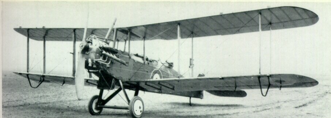
C6078 at Farnborough, fitted with the first Napier Lion engine. When this photograph was taken hot-air pipes and muffs had been added in order to heat the carburettor air intakes. (Photo: Imperial War Museum MH3514)
