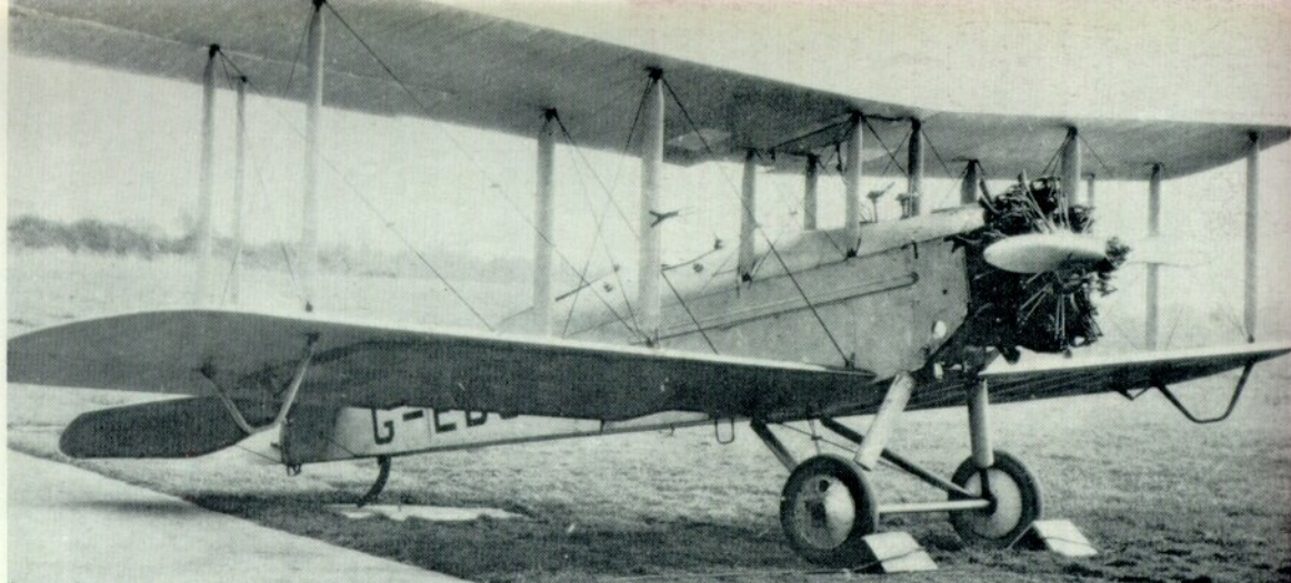
The D.H.9J was a 1926 conversion of the D.H.9 for training purposes, powered by the 350-h.p. Armstrong-Siddeley Jaguar III engine. An improved undercarriage incorporating rubber-in-compression shock-absorbing struts was fitted, together with D.H. differential ailerons. The D.H.9J illustrated here did not have Handley Page slots, but these were fitted to most aircraft of this sub-type.
