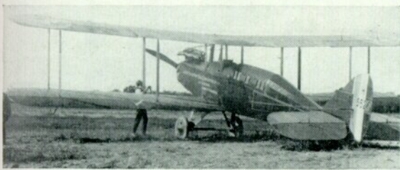
One of the D.H.9s that went to New Zealand, H5627, was modified in much the same way as the British D.H.9C conversions to have an enclosed two-seat cabin. It is here seen at Nelson, New Zealand, on 13th November 1921, in the service of the Canterbury (N.Z.) Aviation Co. Ltd. Its registration in the N.Z. civil register was G-NZAE.
