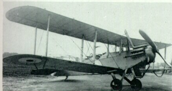
Left: C6078 at Martlesham Heath with enlarged radiator. (Photo: Imperial War Museum Q68133.) Right: A later installation of the Fiat A-12 engine was made in D5748, which also had an experimental tailplane with duplicated bracing wires. The plywood covering of the tail of the fuselage was extended forward. (Photo: Imperial War Museum MH3532)
