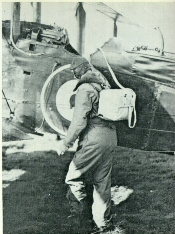
The D.H.9 participated in tests of the Mears parachute in 1918. In normal flight the parachute pack rested on a shelf immediately behind the cockpit, under the fuselage decking.
