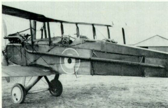
One of the experimental silencers tested on D.H.9s at the R.A.E., Farnborough. (Photo: Imperial War Museum Q67633)
