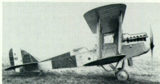
Left: C6078 at Martlesham Heath with enlarged radiator. (Photo: Imperial War Museum Q68133.) Right: A later installation of the Fiat A-12 engine was made in D5748, which also had an experimental tailplane with duplicated bracing wires. The plywood covering of the tail of the fuselage was extended forward. (Photo: Imperial War Museum MH3532)
