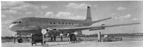
The second prototype Comet G-ALZK before painting, showing the large main undercarriage wheels originally fitted. (Photo: Hawker Siddeley)
