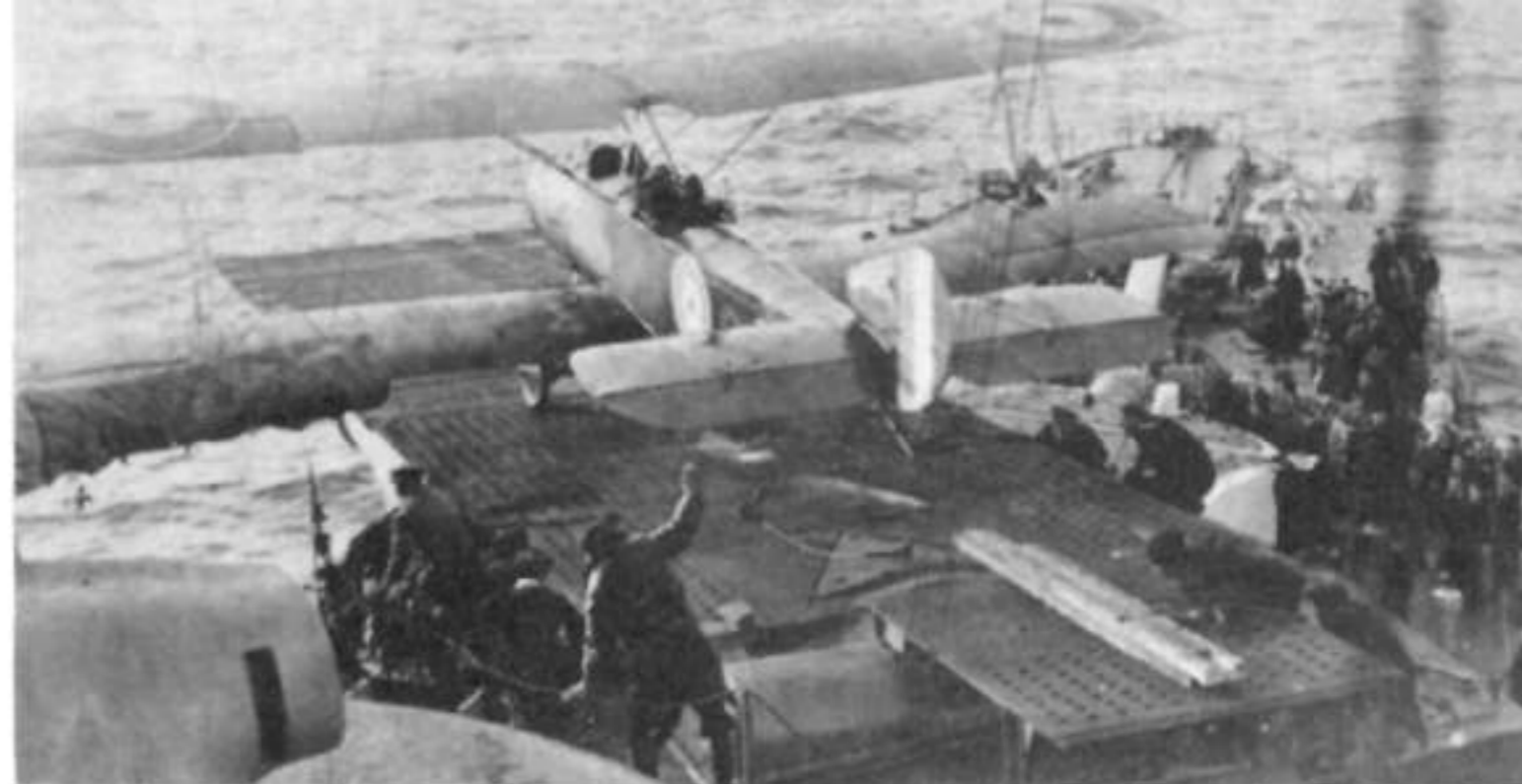
A take-off from B turret of H.M.S. Emperor of India. Note the slotted length of timber serving as a tail guide trestle at the aft end of the platform.
