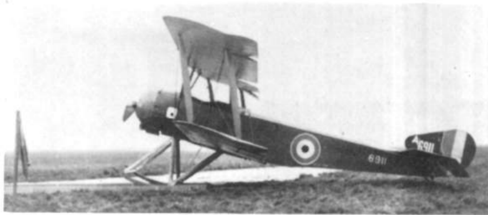
A6911 at Grain with skid undercarriage, 28th February 1918. The skids are resting in wooden troughs, and the lower part of the engine cowling has been cut away.
