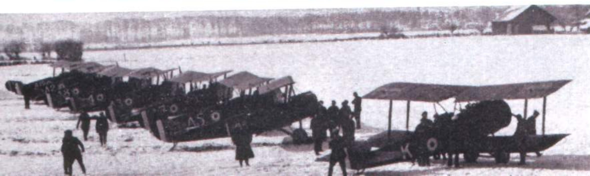
Nine 1 1/2 Strutters of No. 5 Wing, R.N.A.S., at Coudekerque; five are two-seaters, the remainder single-seat bombers. Three of the single-seaters have a Lewis gun above the upper wing.
