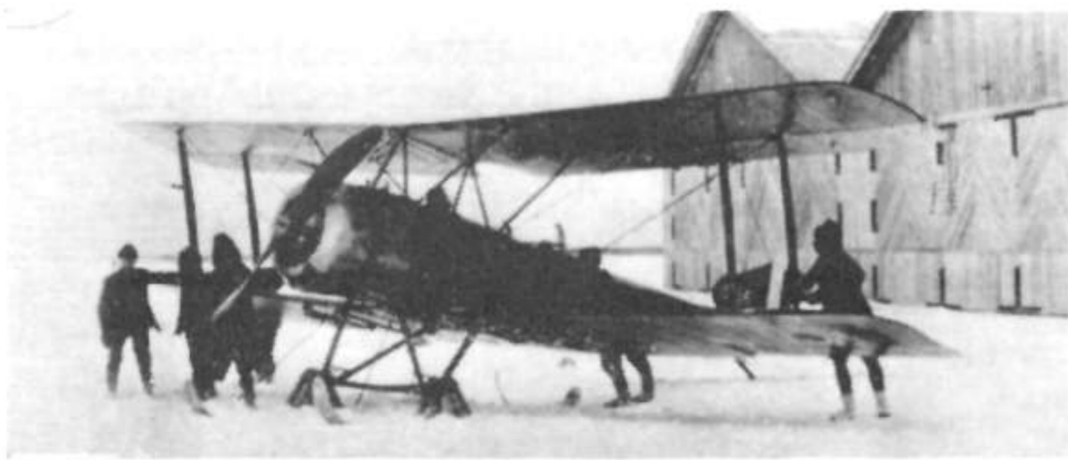
A two-seat 1½ Strutter on skis in Russia. It has a 110-h.p. Le Rhône engine and bomb racks under the lower wings. The serial number is partly obscured but appears to be either A5256 or A5956. (Photo: Peter M. Bowers)
