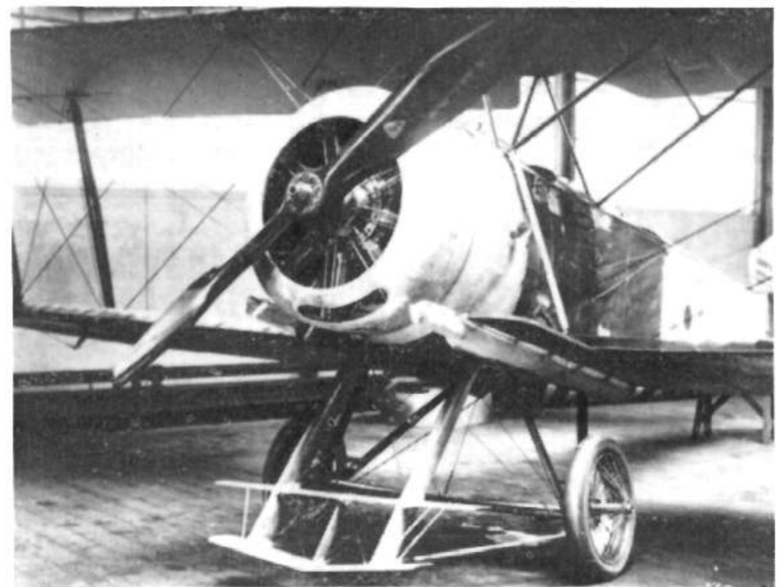
9390 photographed at the Isle of Grain on 8th September 1917, fitted with biplane hydrovane, inflatable air bags mounted on boards that were braced to the upper longerons, and auxiliary bracing at the mid points of the outboard cabane struts.
