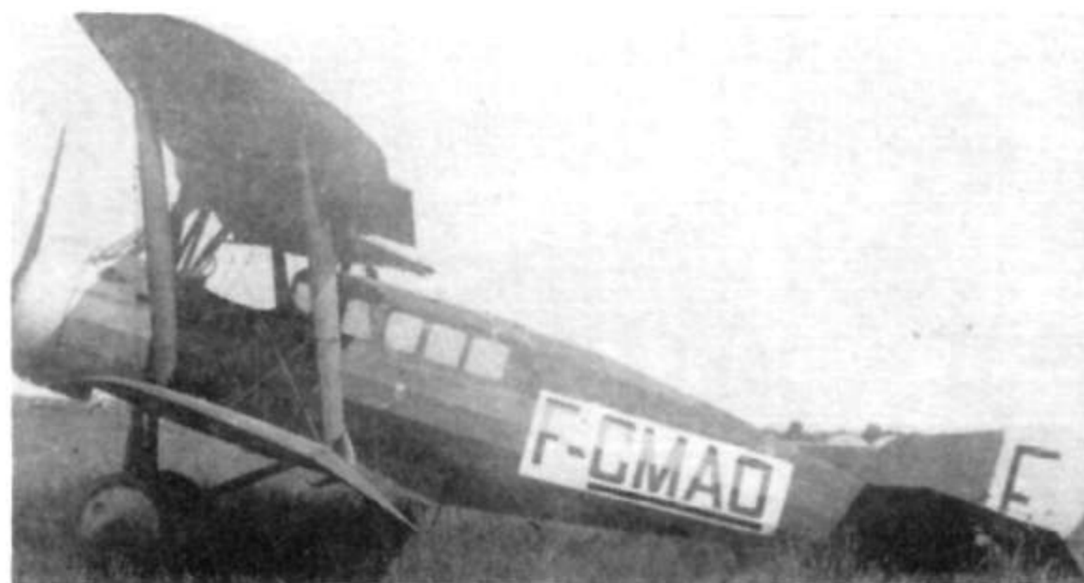
Elaborate modifications to F-CMAO provided an enclosed cabin for two passengers. Gravity fuel tanks were fitted under the upper wings to replace the normal fuselage tanks, the cabane bracing was augmented, and the fuselage sides were faired.
