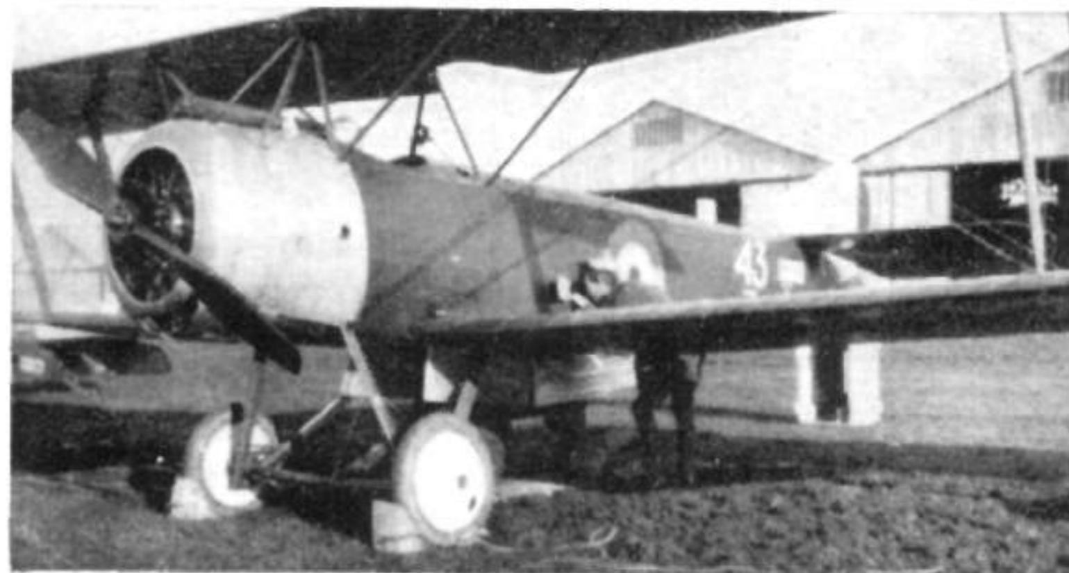
N5116, a Sopwith 9700 of No. 3 Wing, R.N.A.S., Luxeuil-les-Bains, with its bomb doors open and port rear access panel in use. (Photo: Imperial War Museum Q68078)
