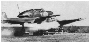
Ground-firing tests by an F 15 machine with heavy calibre rockets.
