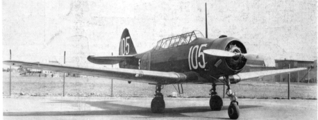
This J 10 aircraft appears to have suffered surprisingly light damage after an undercarriage failure.
