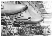
The J 21A production line at SAAB's Trollhättan plant.
