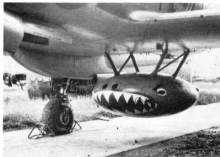
Colourfully decorated weapons pack installed on a J 21RB; this pod mounted eight heavy machine guns, bringing total gun armament to twelve machine guns and one 20 mm. cannon.
