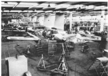
J 21R production at Linköping. First estimates indicated that only 20 per cent. redesign work would be necessary to convert the J 21A airframe for jet power, but in fact the alterations were nearer 50 per cent.
