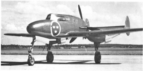
Two views of the prototype J 21A after painting in Swedish Air Force colours. Note nacelle details and long nose-wheel undercarriage.
