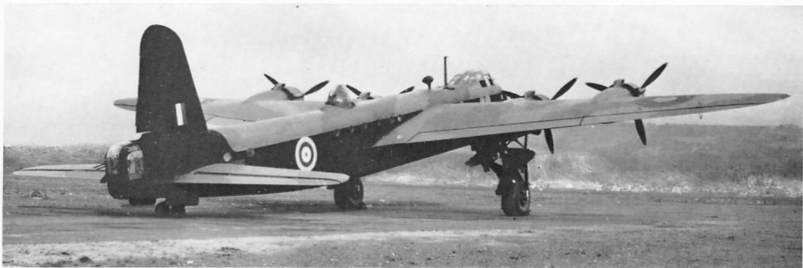
Belfast-built Stirling Mk. I Series III, with twin-Browning F.N.7 dorsal turret; and (below): Mk. I Series III with later-style turret.
