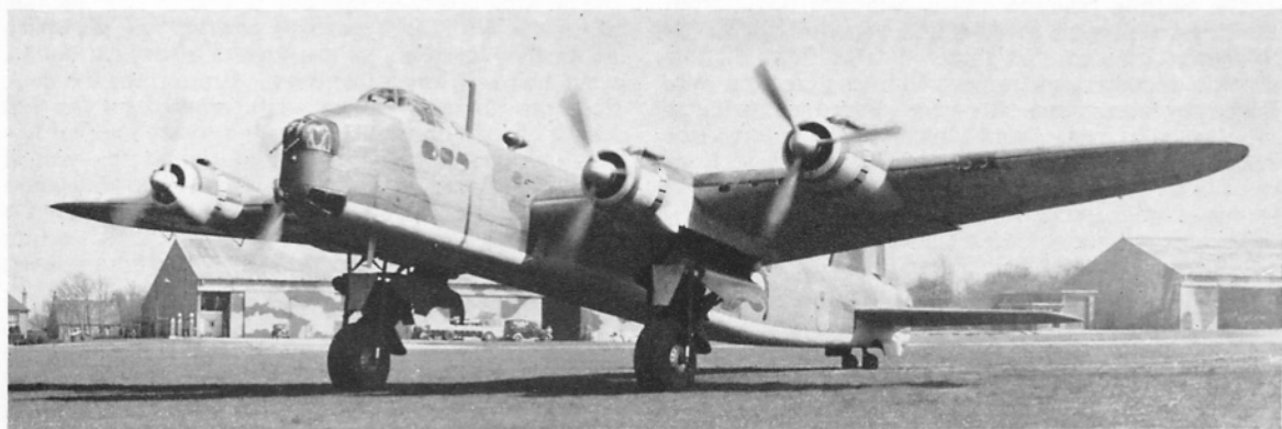
Second prototype Stirling L7605, with strengthened undercarriage.
