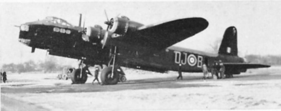
An Austin-built Mk. I, W7455, in the markings of No. 149 Sqn. A fact which the Luftwaffe was quick to exploit was the initial location of the hydraulic recuperators for dorsal and rear turret operation systems in the fuselage immediately behind the R.A.F. roundel marking—a perfect target. (Photo: "The Aeroplane")
