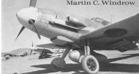
This fine study of a Bf 109F-4 (Tropical) with a drop-tank mounted on centre-section shackles also displays to advantage the insignia of II Gruppe, JG 27 on the cowling. The aircraft was photographed in the Western Desert; and it is with the exploits of JG 27 in the North African campaigns that the Bf 109F is mainly associated in the popular imagination. (Photo: R. C. Seeley Collection)
