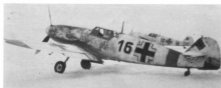
A typical view of a Bf 109 during the Russian winter—in this case, an aircraft of Jagdgeschwader 51. Points of note are the temporary snow camouflage roughly applied over the basic green finish; the yellow wing-tips and belly band; and the removal of the oleo leg covers from the undercarriage.
