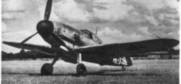
A pre-production Bf 109F-0, powered by the DB 601N engine. (Photo: Imp. War Mus. HU2918)
