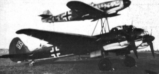
One of the most interesting of all German aircraft projects was the well-known Beethoven/Mistel composite. This sequence of photographs shows the Beethoven-Gerät composite of a Bf 109F-4 and a Ju 88A-4 at three stages of the performance pattern: running up, in flight, and immediately following separation.
