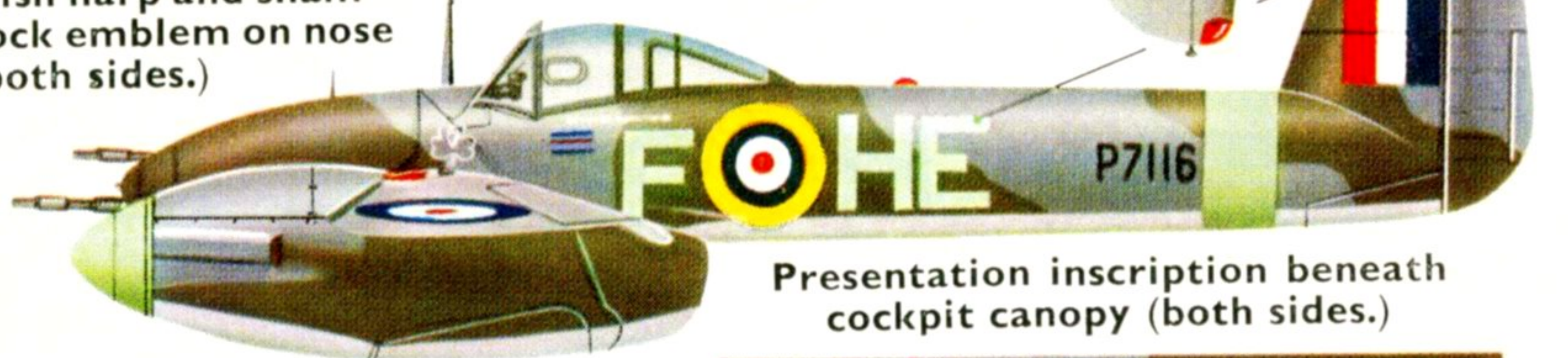
Camouflage pattern on inside of each cowling identical to outer pattern on same engine.
