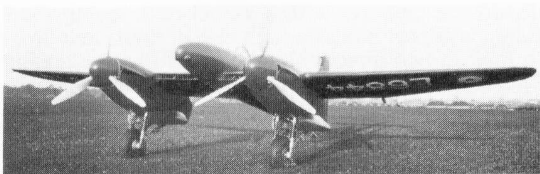
Three views of the first prototype, L6844, October 1938. Note girder bracing of front spar visible through intakes; also mudguards, and position of pitot head. Colour of L6844 was dark grey and NOT red, as is often stated.
