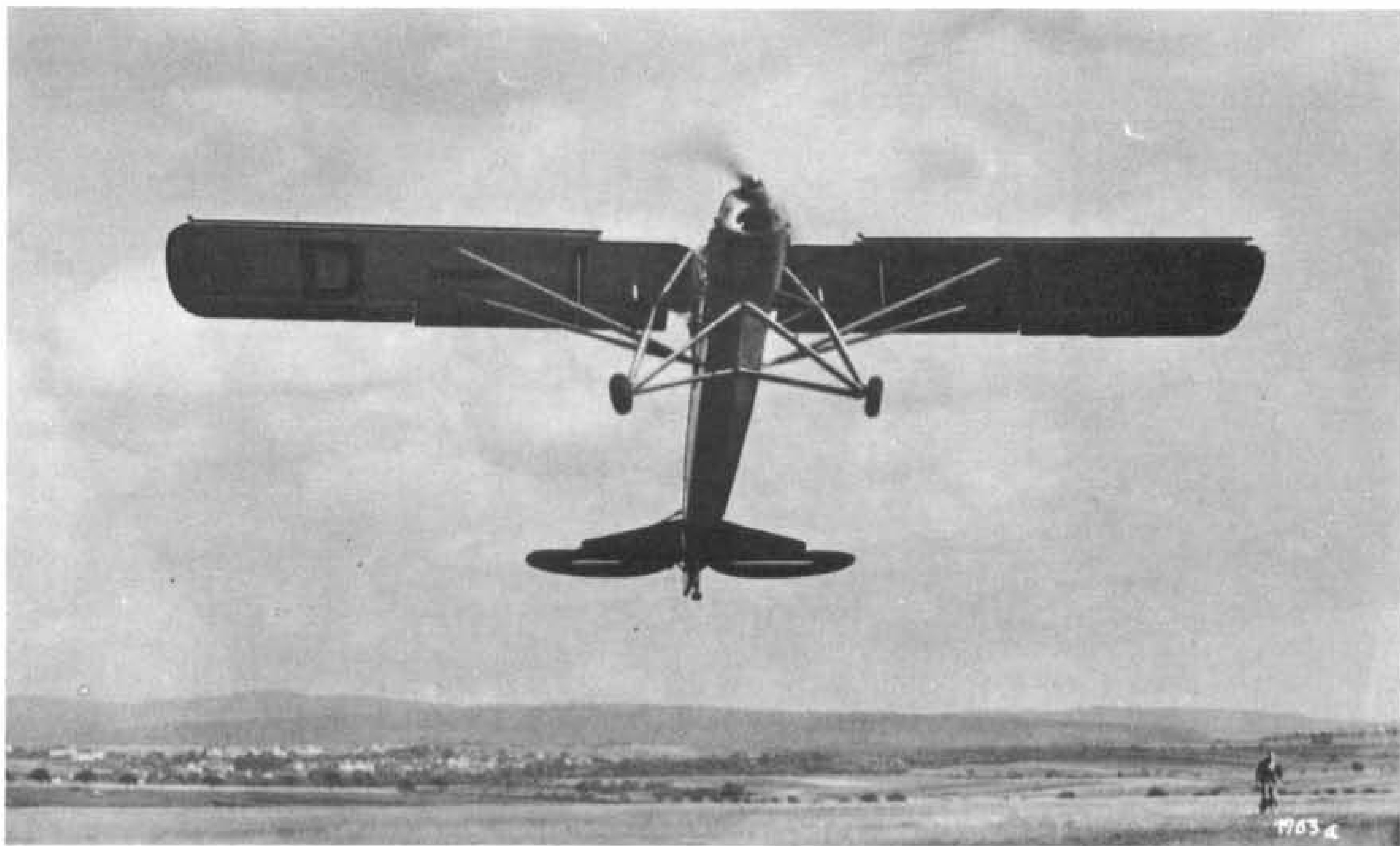
D-IDVS, the Fi 156 V 2 (second prototype), claws into the air during a short take-off demonstration from Fieseler-Flugzeugbau G.m.b.H.'s factory airfield at Kassel-Bettenhausen. (Photo: Fieseler-Flugzeugbau G.m.b.H. ref. 1763d via John F. Brindley)
