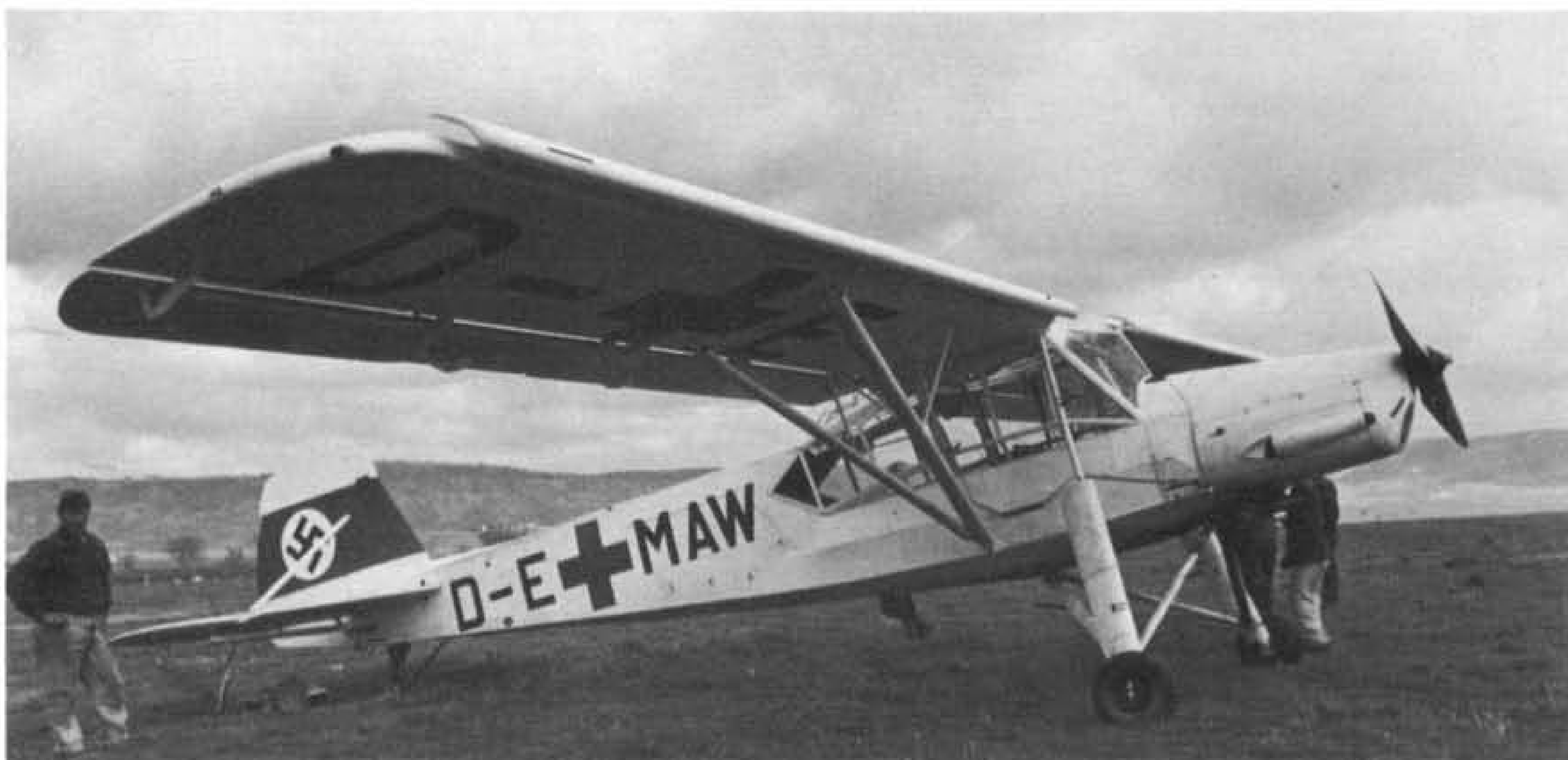
A Fi 156 D-O pre-production series ambulance aircraft. Probably taken in the Mediterranean Theatre during the 1941 period, this aircraft is unusual in not having a Class B.1 (D-I series) registration as carried by other civil Störche. Also interesting is the repeating of the Red Cross symbol within the registration sequence under the machine's wings. (Photo: Bundesarchiv ref. 426-383-16a)
