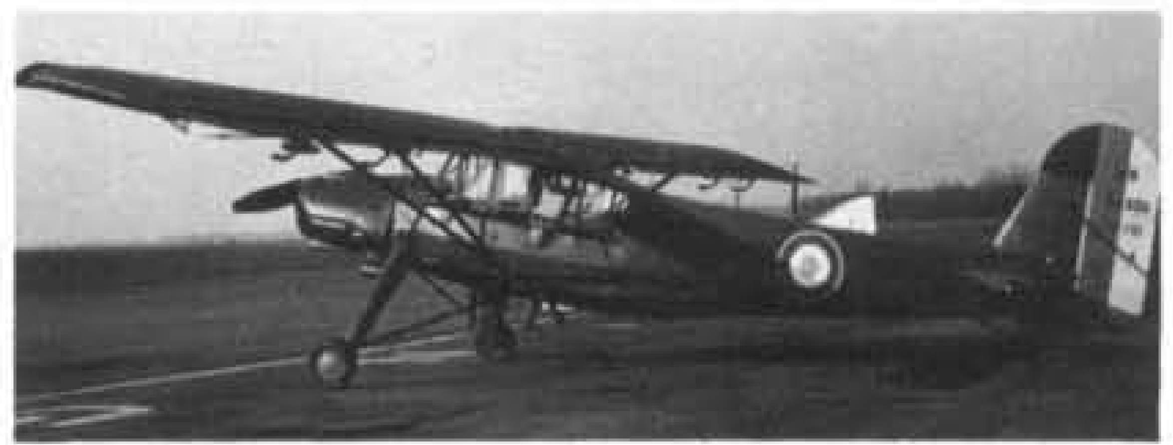
Contrast the MS 500 flown immediately post-war at Boscombe Down with this late-production Criquet—No. 751—taken in France during the mid-1950s. Apart from the addition of a port wing-mounted landing light and both fixed and whip fuselage radio aerials, the later model has a revised rudder contour and other slight modifications to the cabin area.
