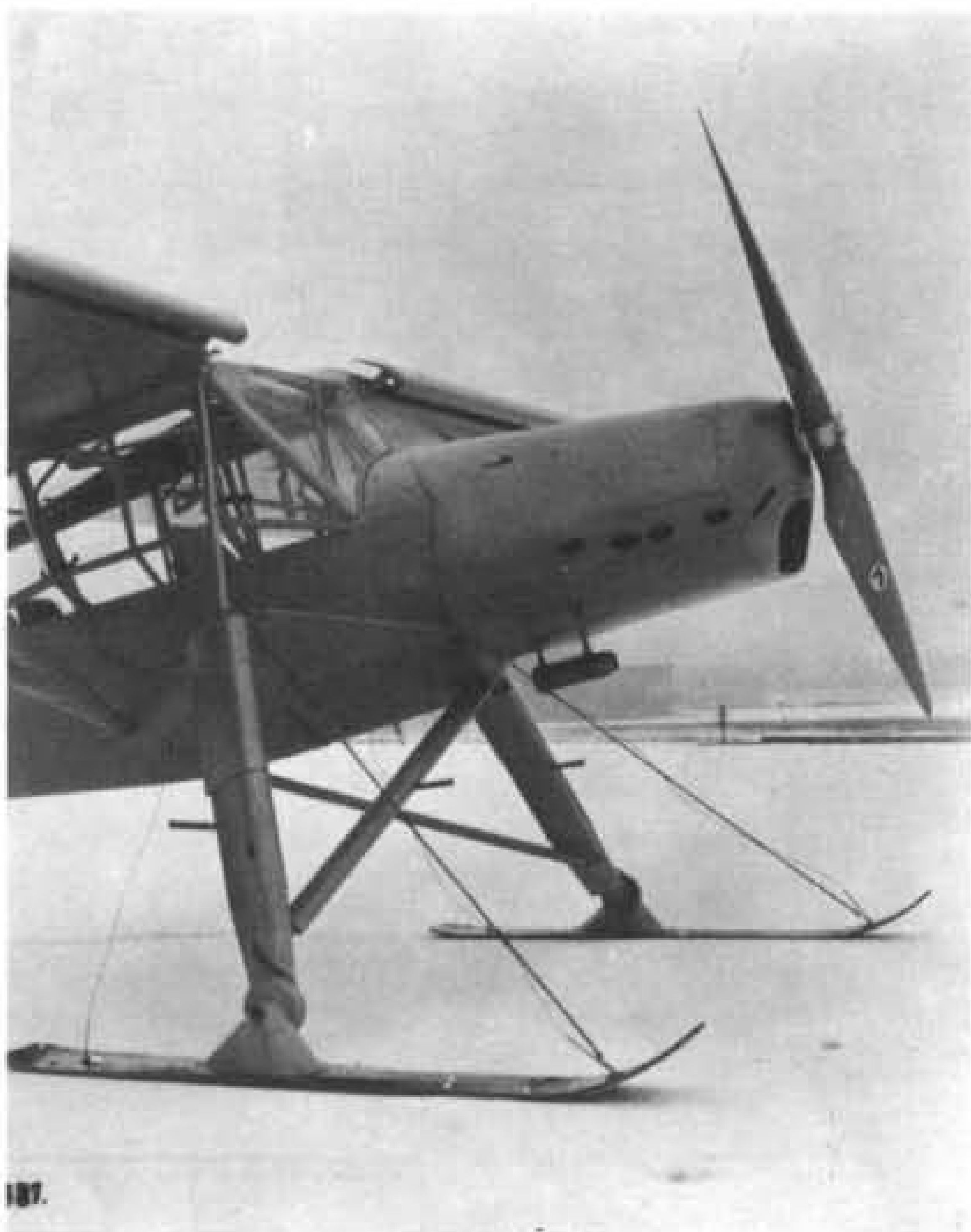
Stork sire. The first Storch prototype, Fi 156 V 1, D-IKVN, depicted here with its conventional mainwheel landing gear replaced by wire-braced skis. (Photo: Fieseler-Flugzeugbau G.m.b.H. ref. 2381 via John F. Brindley)
