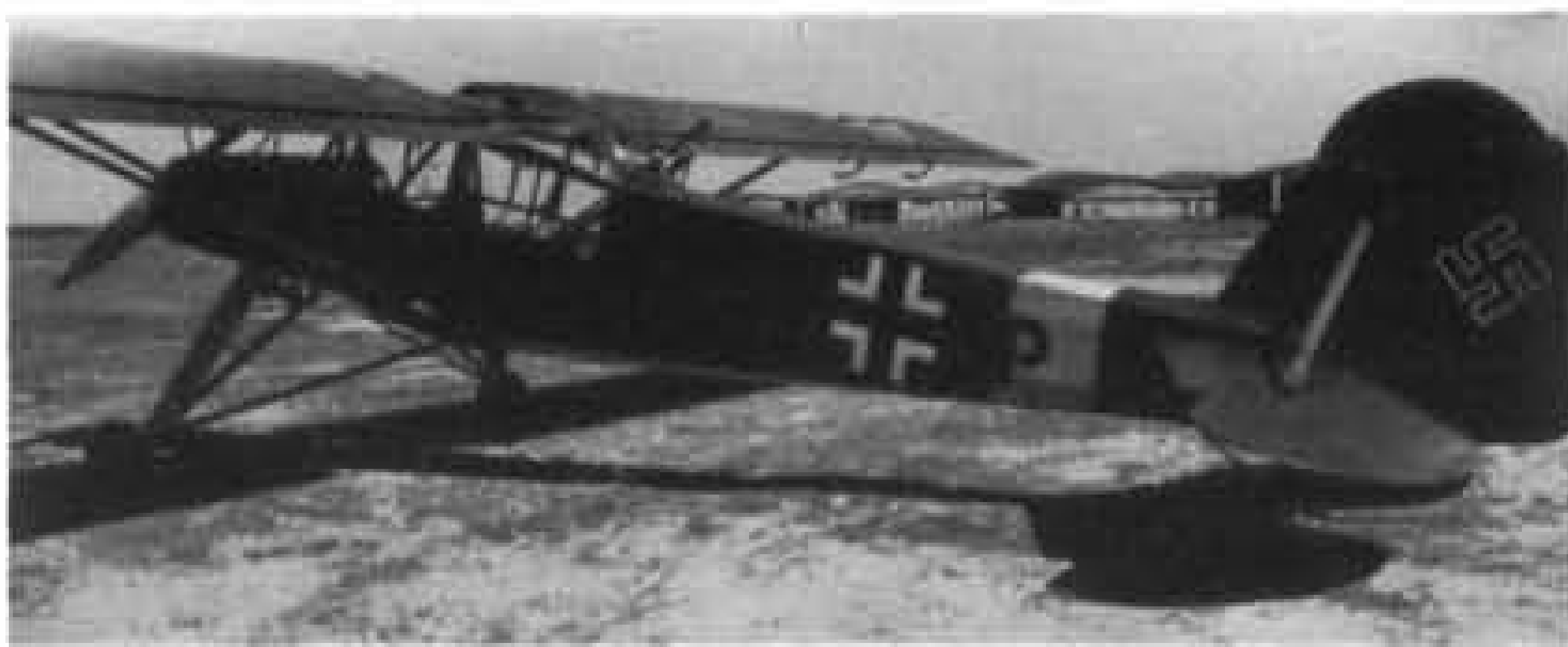
BG+IP is typical of the Fi 156 C-3 variant (armed with a rearward-firing 7.92 mm. Rheinmetall-Borsig MG 15 in a circular cupola) produced in large numbers simultaneously at Kassel and Puteaux in the middle war years.
