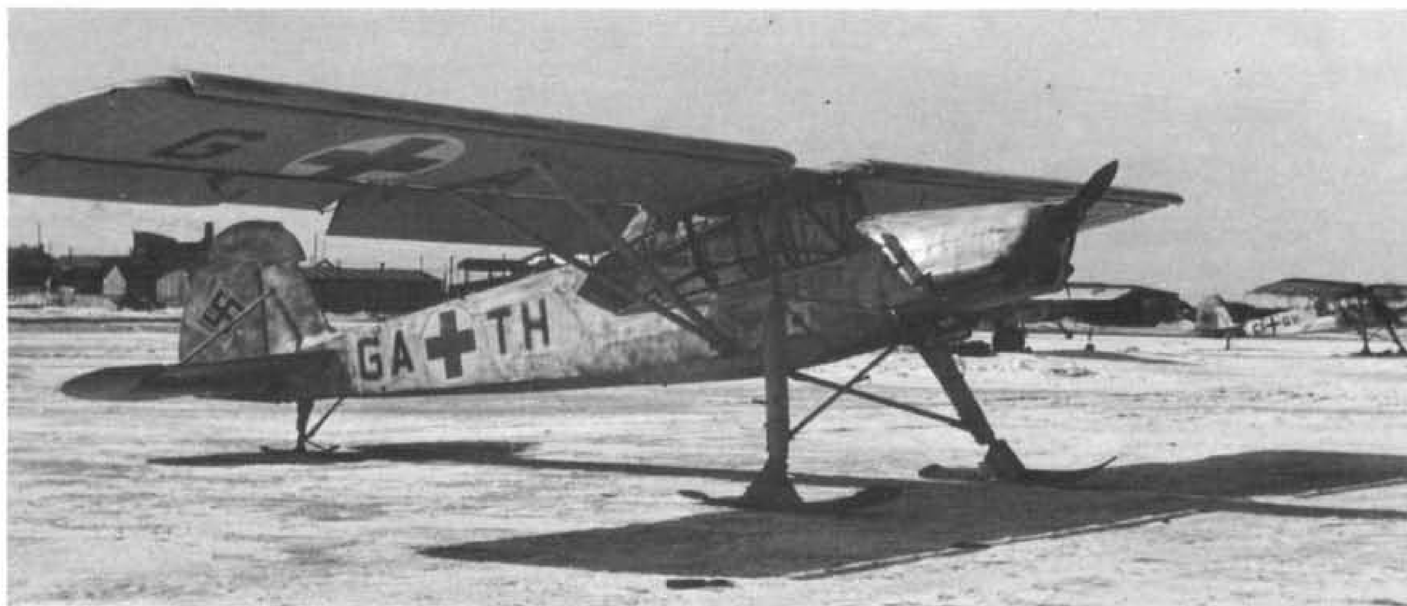
Unarmed ski-equipped Fi 156 D-1 ambulance aircraft (coded GA+TH) flown by an unidentified Sanitätsflugbereitschaft—Duty Ambulance Flight. Note the revised Red Cross symbol boldly outlined by a white circle. (Photo: Bundesarchiv ref. 394-1452-15)
