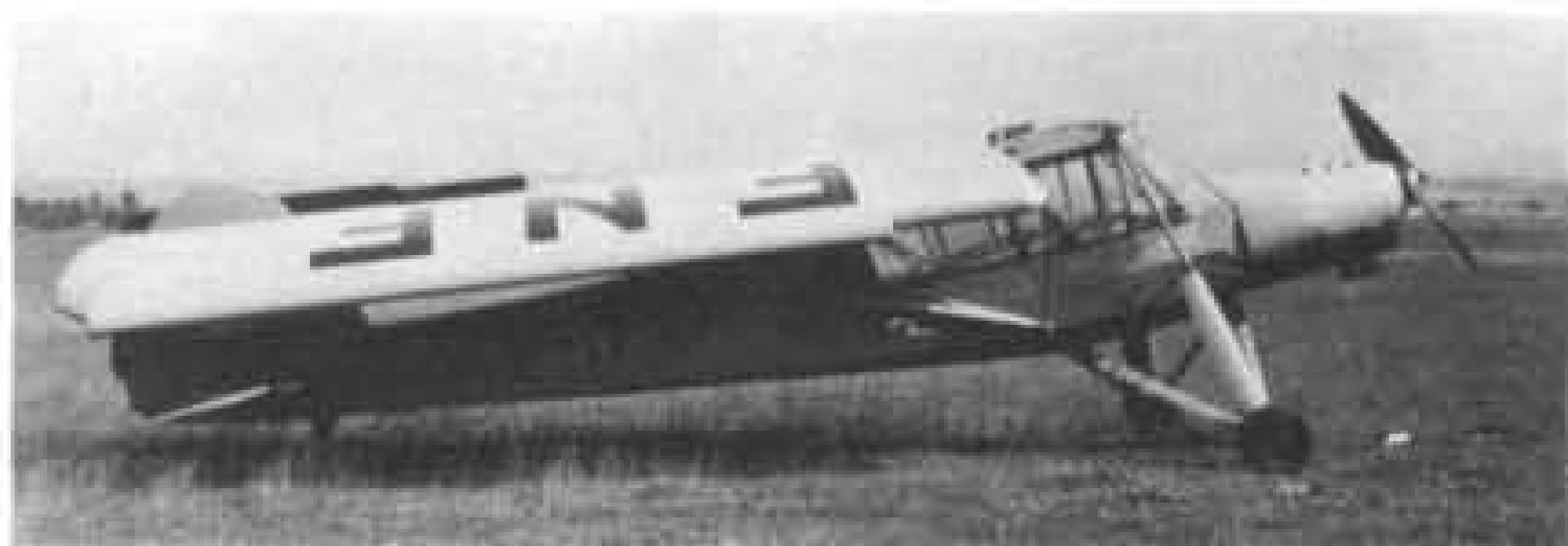
Little stressed, was the wing-folding capability of the Fieseler Storch. This considerably eased the problem of accommodation at airfields with limited hangar space and made the type speedily transportable by road. D-IFNF was a pre-production Fi 156 A-O. (Photo: Fieseler-Flugzeugbau G.m.b.H. ref. 1766 via John F. Brindley)
