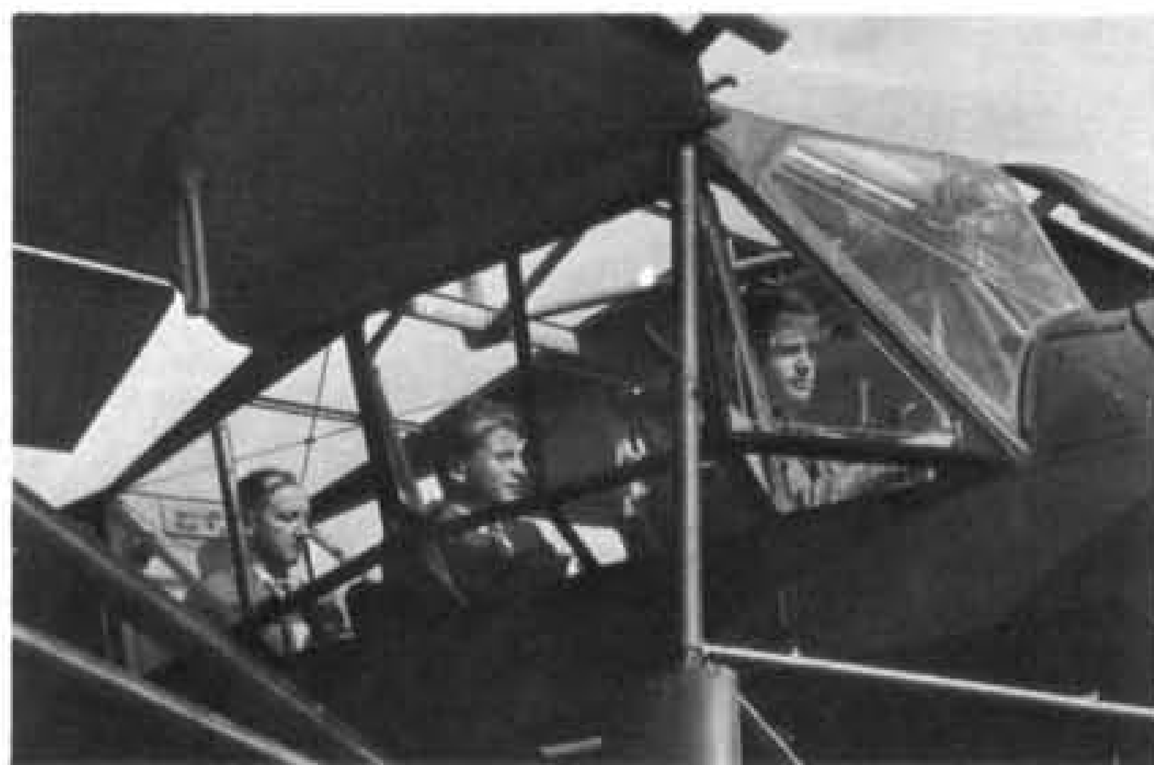
Close-up of the tandem seating arrangement in the Fi 156. Equipment changes according to varying rôles was the deciding factor as to whether two or three seats (or in the case of the ambulance version, a solo layout) were fitted in the Storch. (Photo: Fieseler-Flugzeugbau G.m.b.H. ref. 677L via John F. Brindley)
