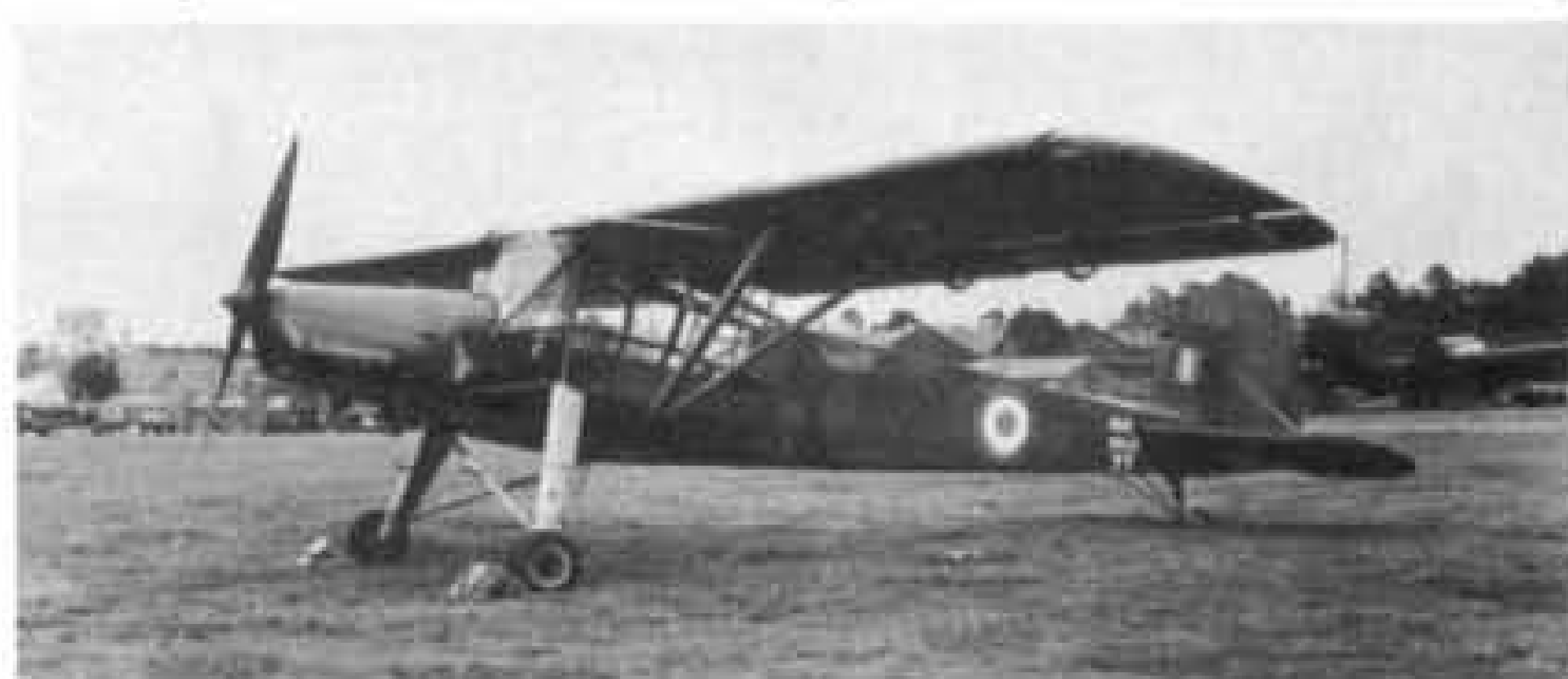
Taken on September 11, 1945 at the Royal Aircraft Establishment, Farnborough, this is the final production variant of the Storch , the Fi 156 C-7 .
