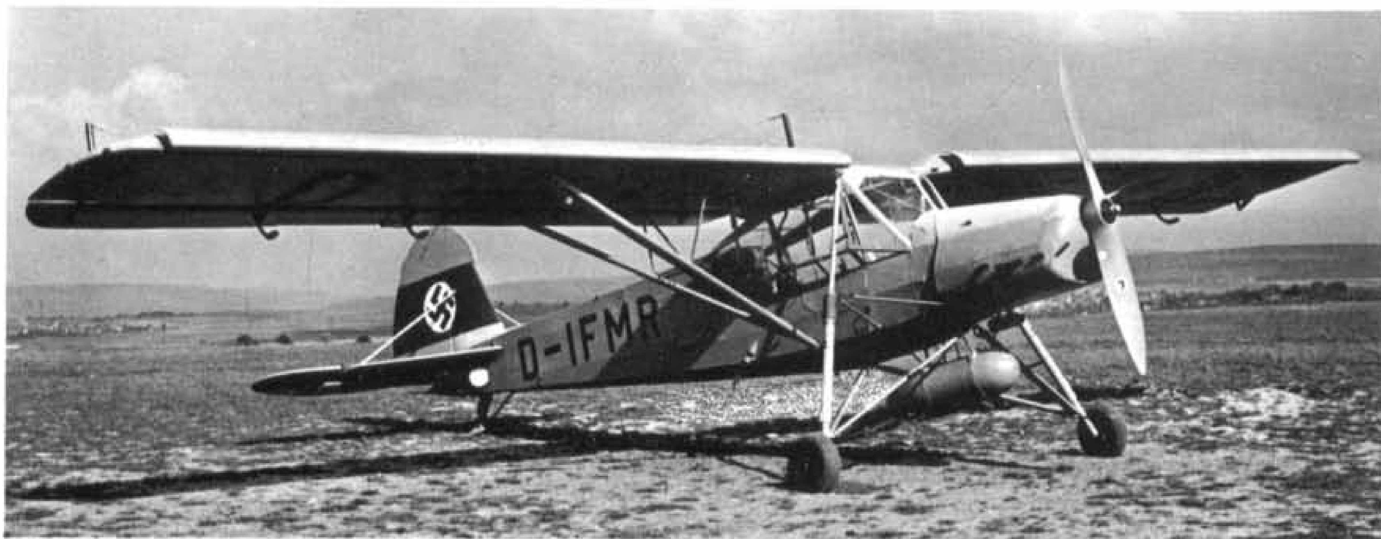
The fourth prototype Storch, D-IFMR, was used for a variety of trials. These included range tests—with an additional fuel tank slung below the main undercarriage cross-bracing—and the proving of radio equipment.
