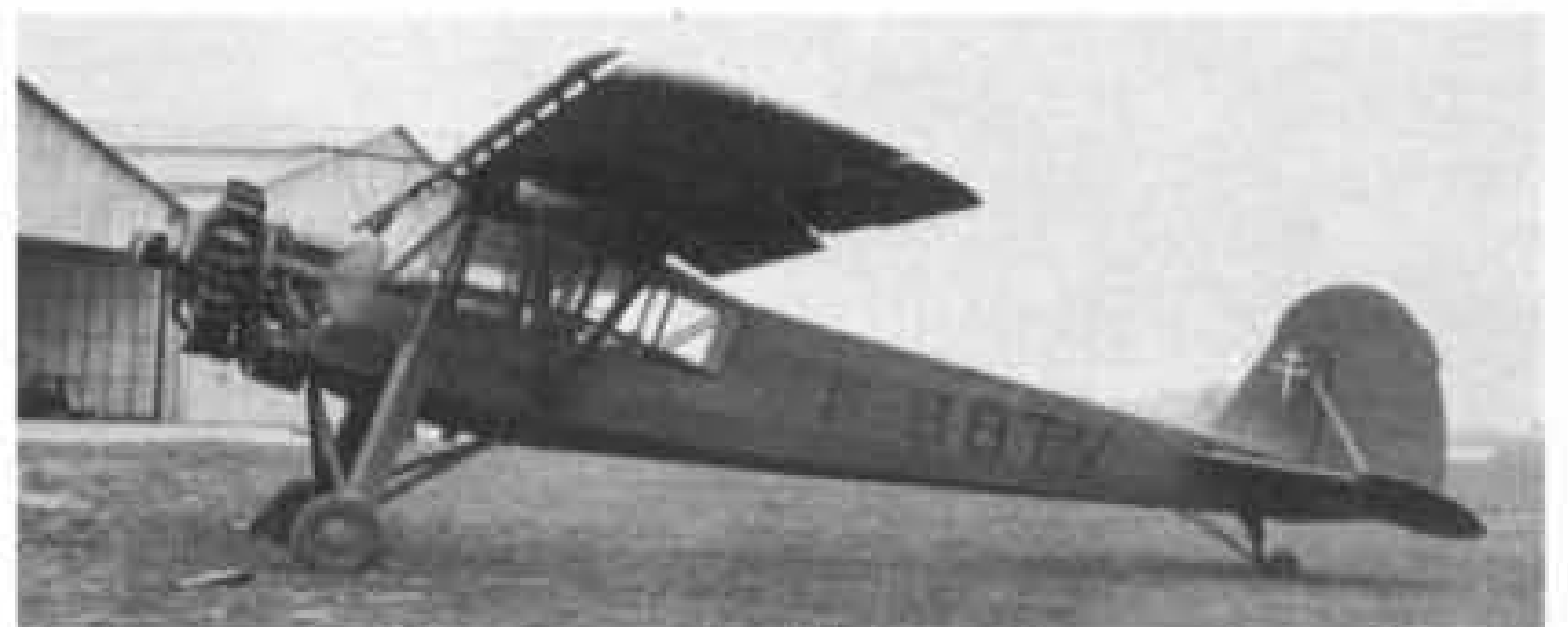
Replacement of the Argus As 10 C or P motor by a 230 h.p. Salmson 9 ABC air-cooled 9-cylinder radial engine, although marring the lines of the Storch, was inevitable as supplies of the German-manufactured motors dried up in the West. F-BBTV is seen at Guyancourt, near Paris, during early May 1948.
