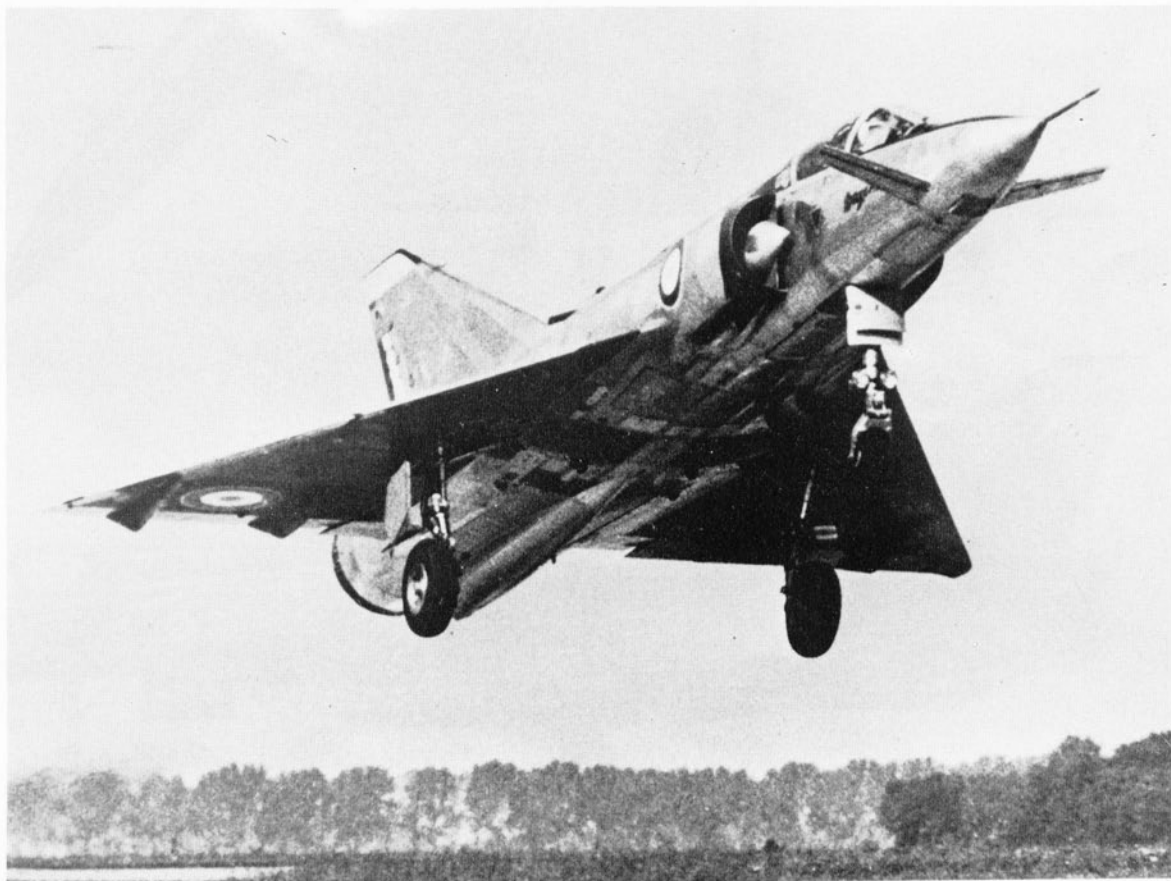
The first Milan development aircraft, with fixed foreplanes.
