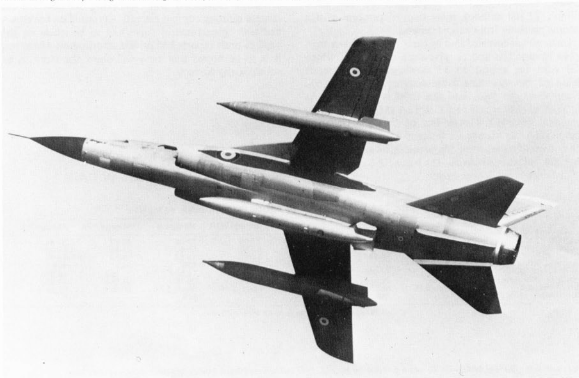
The variable-geometry Mirage G with wings in their forward position and carrying three 1,200-litre (264 Imp. gallon) external fuel tanks.
