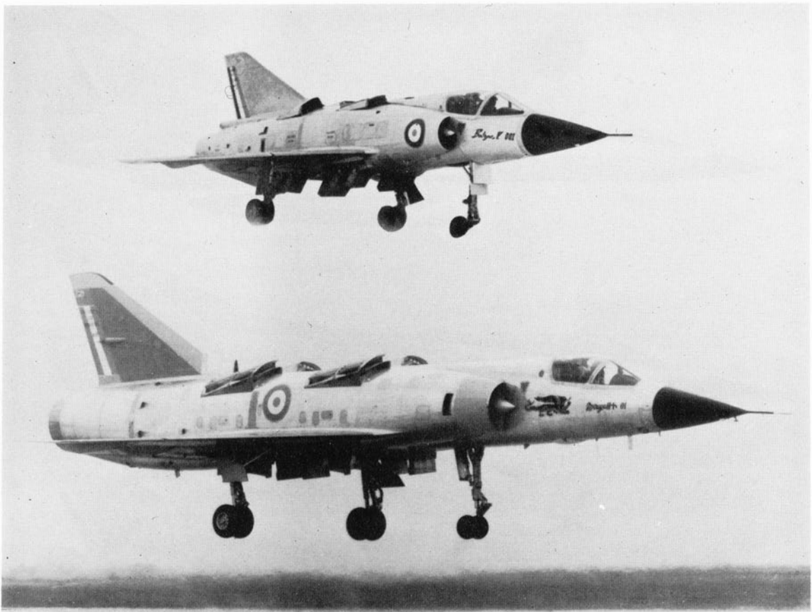
View of the Balzac (upper) and Mirage III V-01 (lower) experimental VTOL aircraft in hovering flight.
