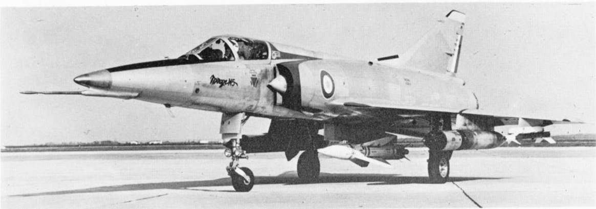
Mirage 5 development aircraft carrying an Nord AS 30 missile under the centre-section and two Dassault JL 100 combined fuel tank/rocket launchers and two Sidewinder missiles under the wings.
