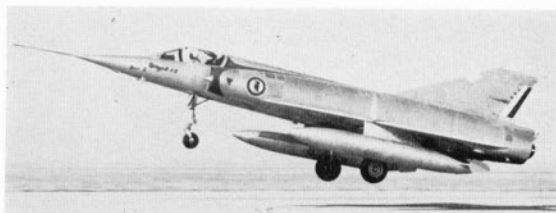
First pre-production aircraft was the Mirage IIIA-01, seen here landing at Istres with external fuel tanks.
