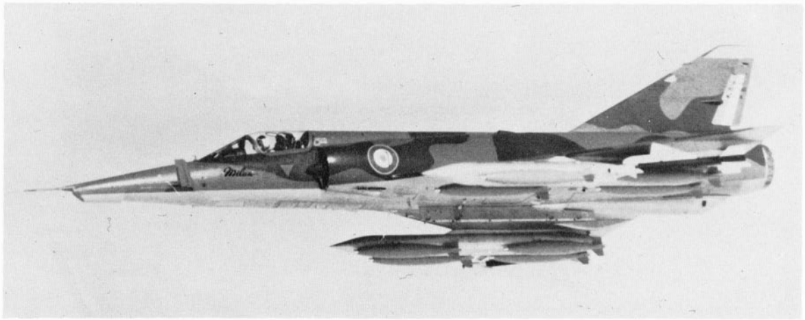
The Milan S-01 seen carrying two Sidewinder missiles, two 500-litre (110 Imperial gallon) auxiliary fuel tanks, and eight 250-lb. bombs—these latter attached to the fuel tanks. This is not the Milan's maximum load: it could also carry another two 250-lb. bombs under the centre section.
