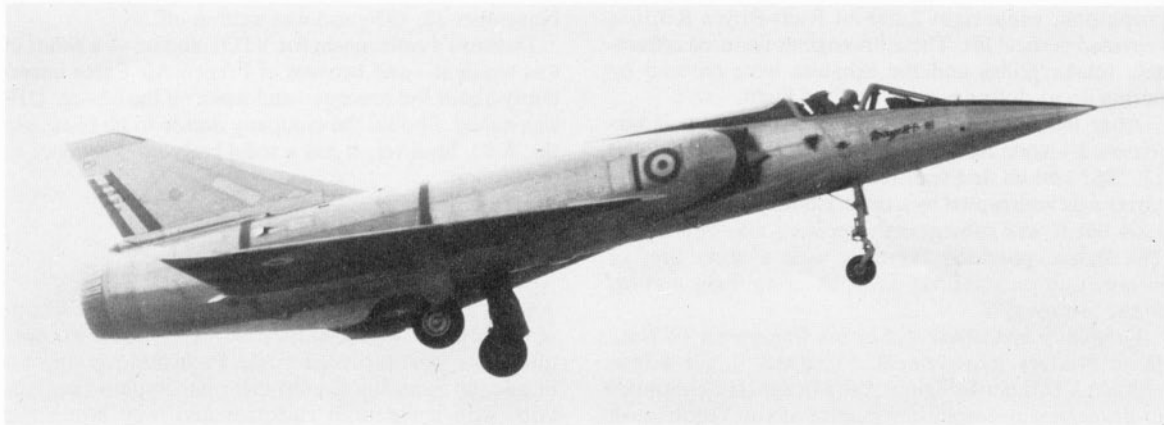
The Mirage IIIT-01 engine test-bed.
