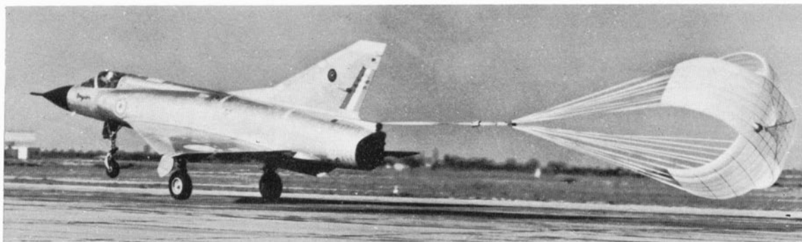
Mirage IIIC deploying its braking parachute during the landing run.
