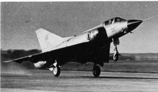
One of the pre-production Mirage IIIAs was converted to take a Rolls-Royce Avon engine when the Royal Australian Air Force expressed interest in using this powerplant on its Mirages. In the event R.A.A.F. Mirages have Atar engines.
