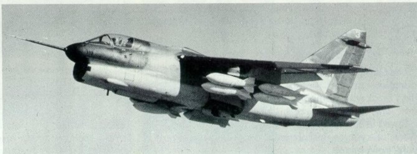
(Right) Another stores' arrangement tested on the first A-7D; inboard pylons each have a single 300-US gal. drop tank and middle pylons have paired AGM-65A TV-guided missiles. (Photo: Vought PR-9343)
