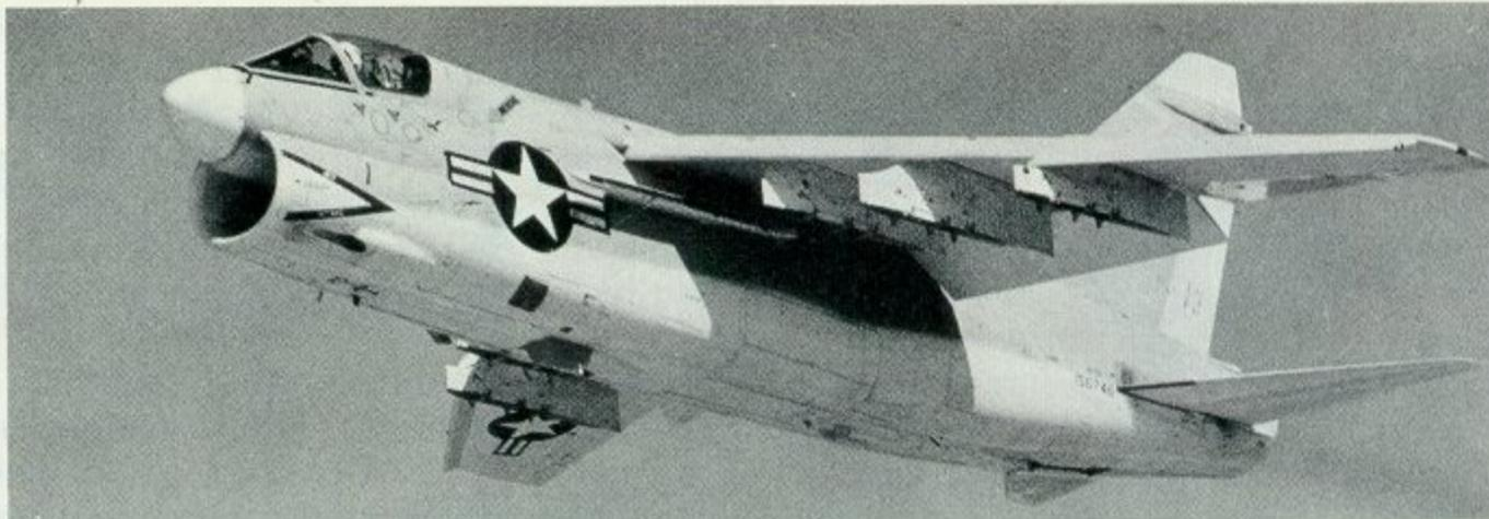
The Navy's Mk. 12 cannon—used on the earlier A-7A/B—were replaced by a single M61 and 1,000 rounds of ammunition.
