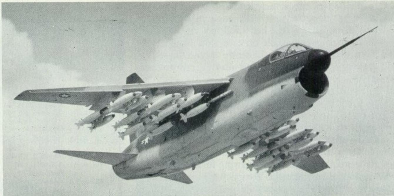
(Right) Third USAF A-7D (AF67-14584) reveals characteristic refuelling "hump" above wing root. Except for the 17th A-7D, this feature was not incorporated in production until the 27th example. Single pylons each carry 4 × 750-lb. dummy bombs for test purposes. (Photo: Vought PR-8878)
