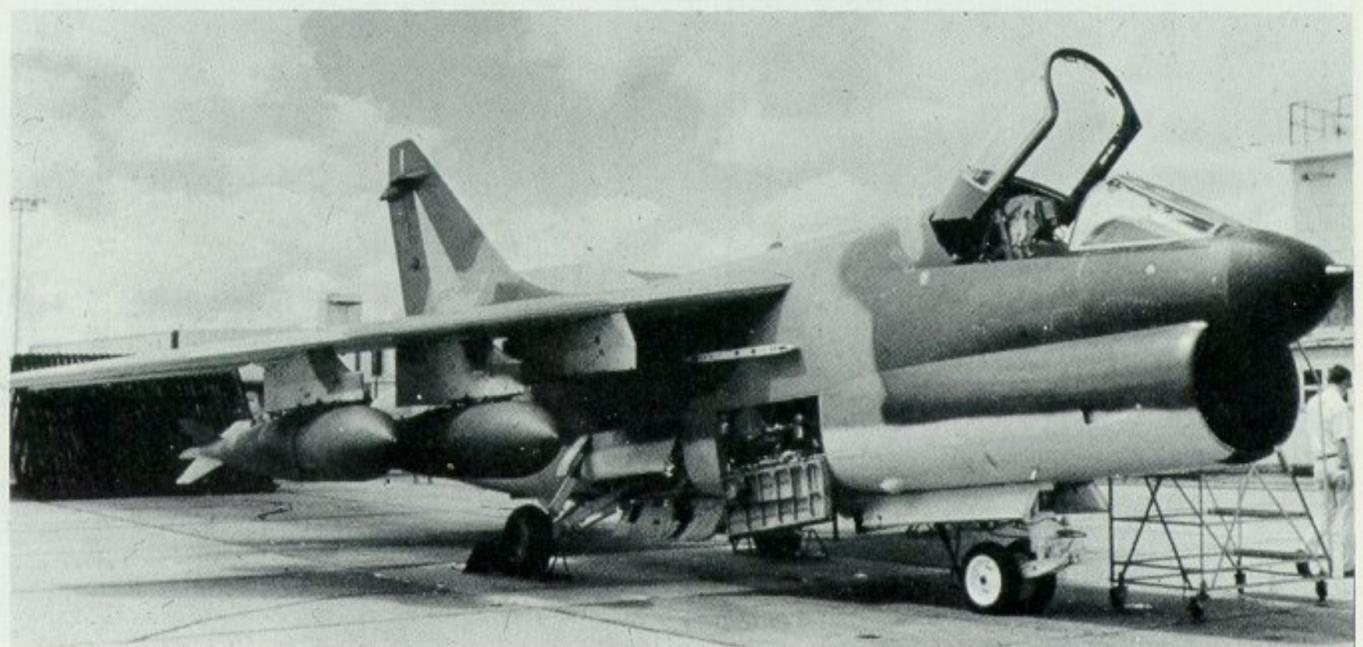
*Prototype A-7D (AF67-14582) shows off biggest-yet bombs (4 × 3,000-lb.) carried by Air Force Corsair IIs; but not heaviest total load.*
