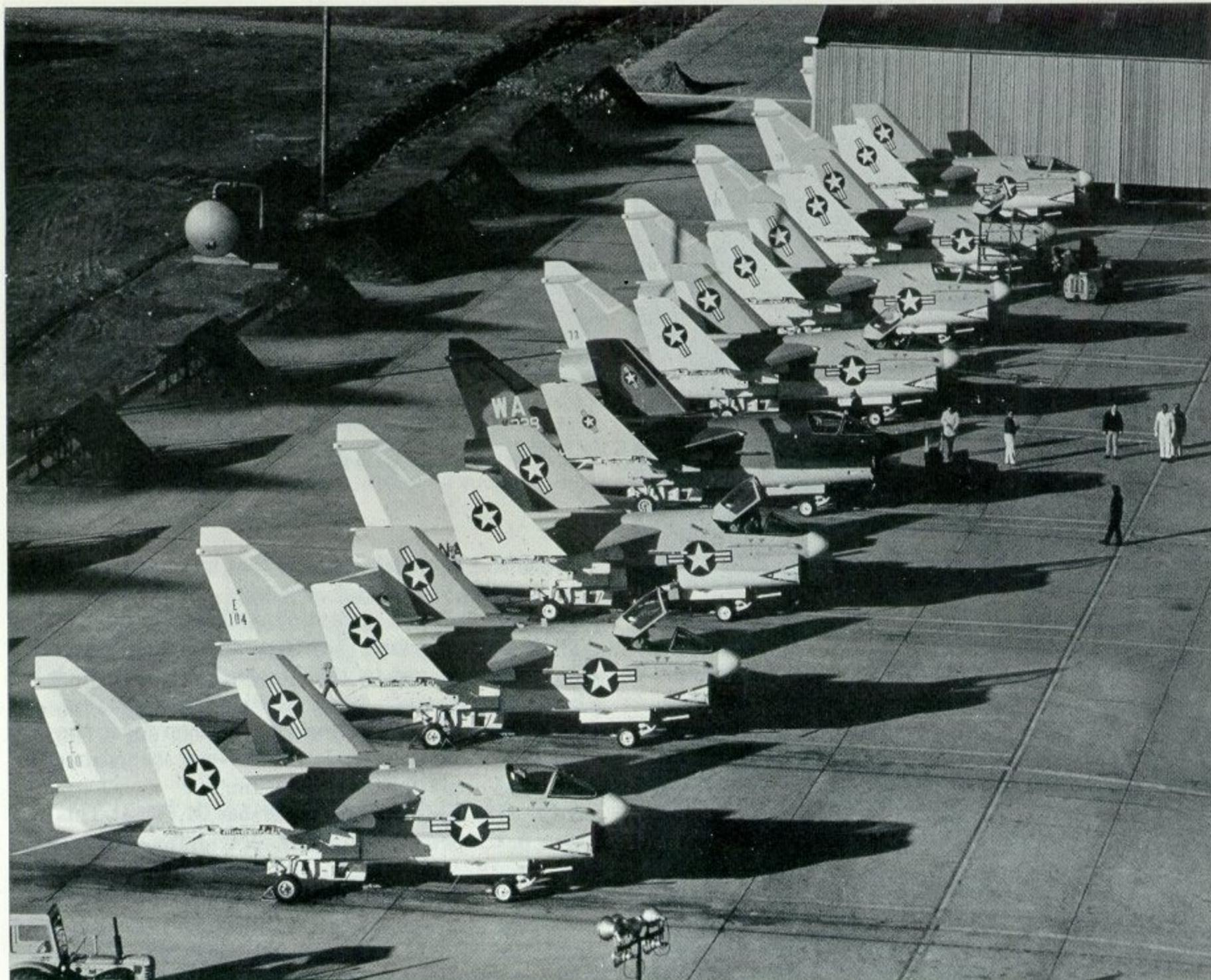
Flight line at Dallas, Texas, where the Vought Aeronautics Company (a division of LTV Aerospace Corporation) built these US Navy A-7Es which sandwich a camouflaged US Air Force A-7D. This early-production A-7D (AF69-6238) bears the tail letters WA for the 57th Fighter Weapons Wing based at Luke AFB, Arizona. Nearest Navy Corsair II, with temporary "E80" on rudder, is BuNo. 156813. Table III on page 120 details USN/USAF serial numbers. (Photo: Vought, ref. PR-9192)
