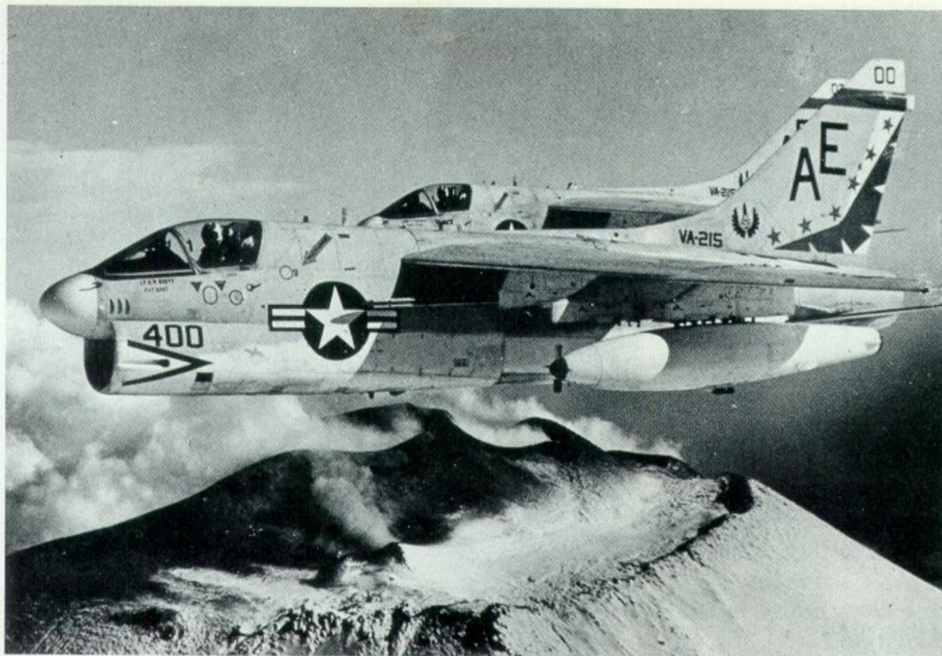
*VA-215 again . . . with Sicily's Mt. Etna for thermal lift. By 1970, the "Barn Owls" A-7Bs now sport AE for CVW-6 while aboard USS Roosevelt. Outer pylon supports "Buddy Mission" in-flight refuelling store which Douglas Aircraft (El Segundo) developed in mid-1950s. (Photo: US Navy via Vought PR-9374)*
