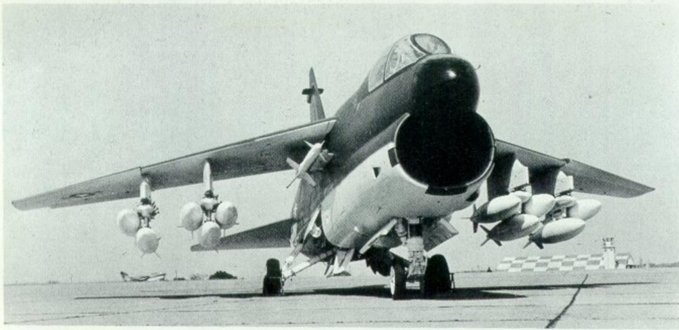
*Temporary A-7G configuration—to meet original Swiss Air Force requirements— was achieved by reworking a standard A-7D. Shown here is one of the loads offered for export, ten 1,000-lb. bombs and two AIM-9 Sidewinders. On April 11, 1972, a second “Swiss reconfigured” A-7D left Dallas Naval Air Station for the SwAF base at Emmen for several weeks’ evaluation.*
