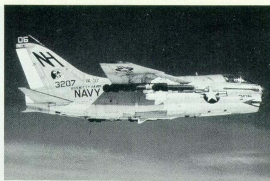
NH for CVW-11 aboard USS Kitty Hawk circa 1969. An A-7A (BuNo. 153207) of VA-37 with blue-painted nose radome and tips to wings and fin. Interdiction mission over Laos with Bullpup B VT-fused missiles and 500-lb. Mk. 82 Snakeye bombs.
