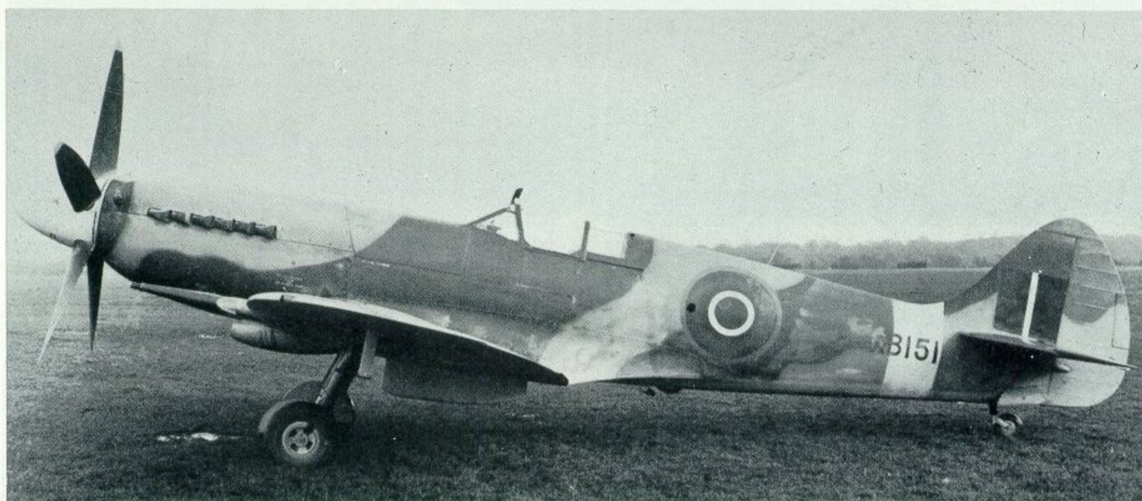
Serving as the Spitfire Mk. XIV conversion prototype was this Mark VIII (RAF serial JF319) which displays the modified fin and rudder of the interim stage. (Photo: Imperial War Museum, ref. MH.5269)
