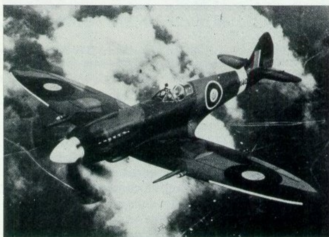
Serving as the Spitfire Mk. XIV conversion prototype was this Mark VIII (RAF serial JF319) which displays the modified fin and rudder of the interim stage. (Photo: Imperial War Museum, ref. MH.5269)
