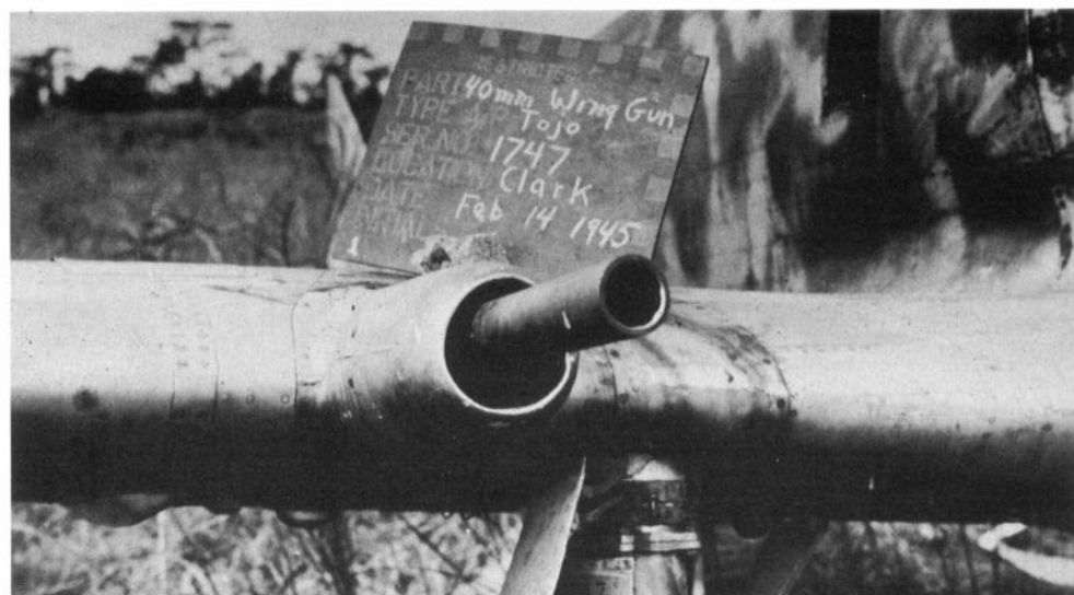
Close-up of a 40-mm. Ho-301 cannon installation on a Ki-44-II-Hei found at Clark Field, Manila, early in 1945. (Photo: US National Archives via Rene J. Francillon)
