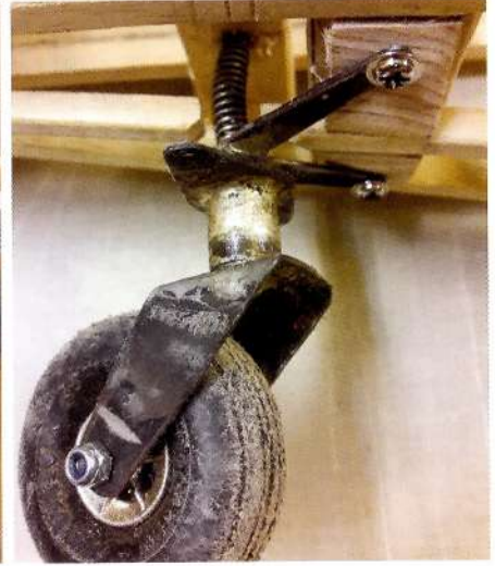
The landing gear has been accurately replicated, but the damping is based on springs rather than the hydraulic system used on the full size
