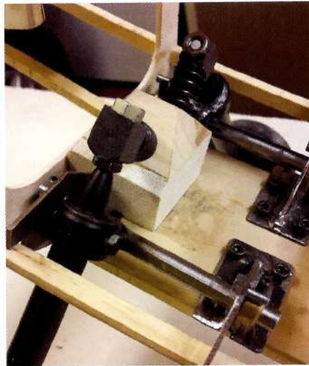
The landing gear has been accurately replicated, but the damping is based on springs rather than the hydraulic system used on the full size
