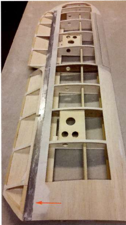
A 0.3 mm aluminium strip has been added to obtain the exact gap required between the wing and the control surfaces
