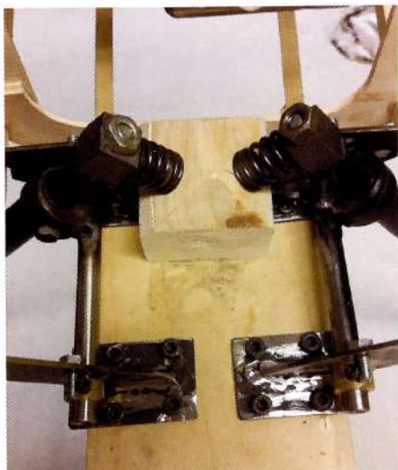
The landing gear has been accurately replicated, but the damping is based on springs rather than the hydraulic system used on the full size
