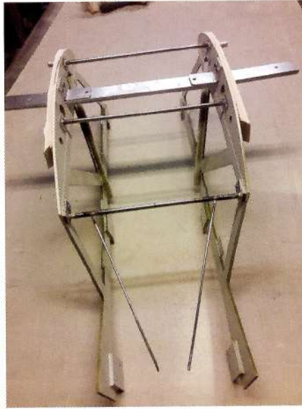
The central part of the fuselage includes these welded struts and metal wing panel joiner
