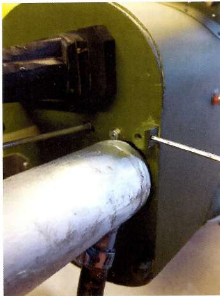
The system used to mount the cowl
