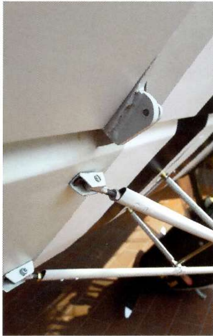
The wing struts are hinged on the wing panels
