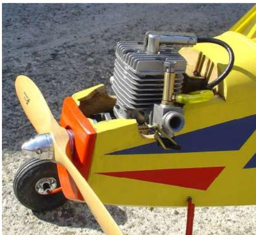
Anyway, after the fuel changing, the fuel economy will be dramatically increased and the maximum rpm will decrease. The bad news is an almost 20% reduction in power output using gasoline in comparison with the same engine feed with alcoholic fuel.
